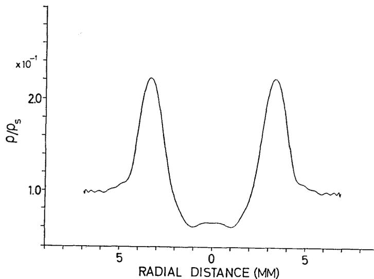
Fig. 8. Radial distribution of density ( $z=9$  mm,  $p_s=13.3$  kPa,  $p_\infty=1.31$  kPa).
