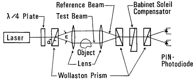
Fig. 1. Optical system for laser differential interferometry.
