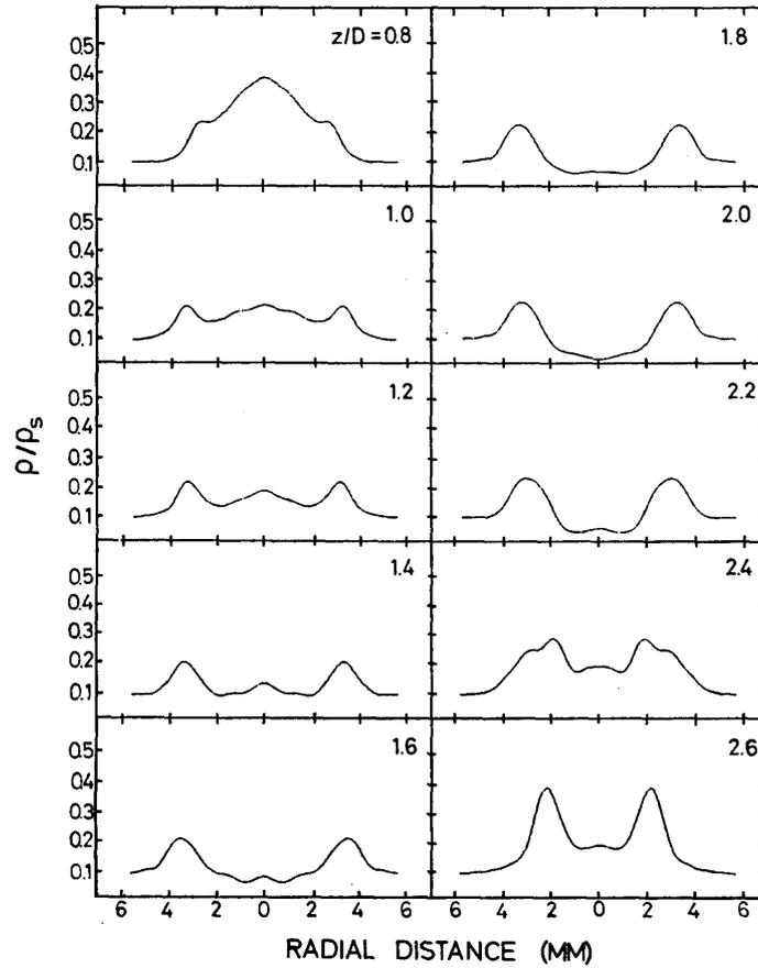
Fig. 9. Radial distributions of density at 10 locations between  $z=4$  mm and  $z=13$  mm from the orifice.
