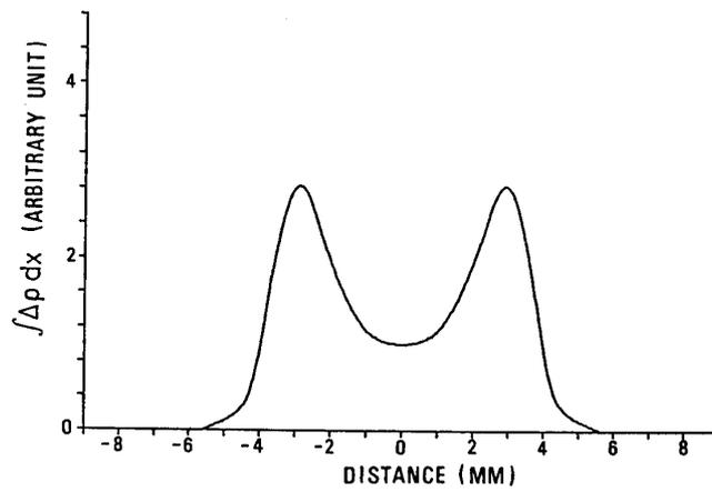
Fig. 6. Variation of  $\int \Delta\rho dx$  in the  $y$ -direction ( $z=9$  mm,  $p_s=13.3$  kPa,  $p_\infty=1.31$  kPa).
