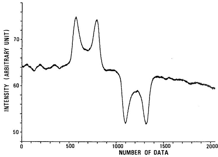
Fig. 5. Measured interference intensity ( $z=9$  mm,  $p_s=13.3$  kPa,  $p_\infty=1.31$  kPa).
