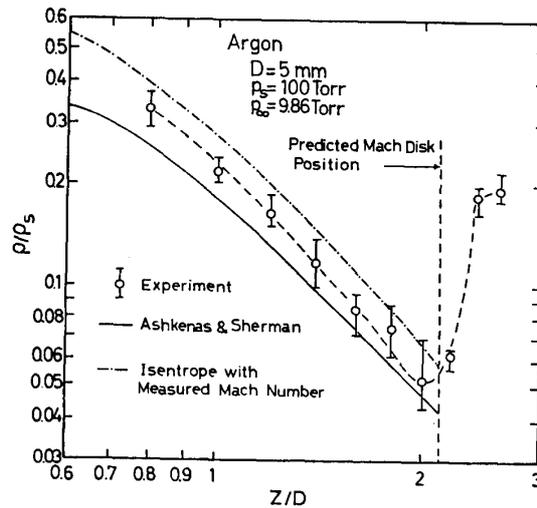
Fig. 10. Comparison of measured densities with predicted ones on the flow centerline.
