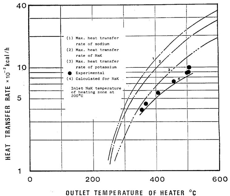
Fig. 6. Hea. transfer rate for looped type heat pipe employing NaK as working fluid.
