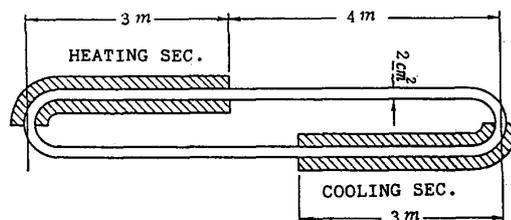
Fig. 1. The fundamental structure of the looped type heat pipe.
