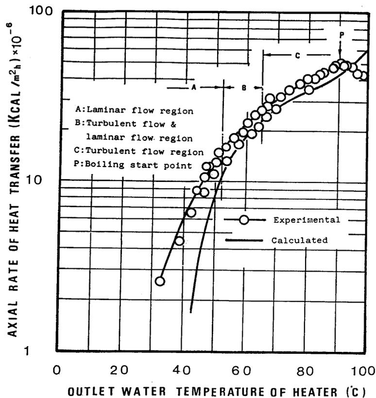
Fig. 7. Heat transfer rate for looped type heat pipe employing water as working fluid.
