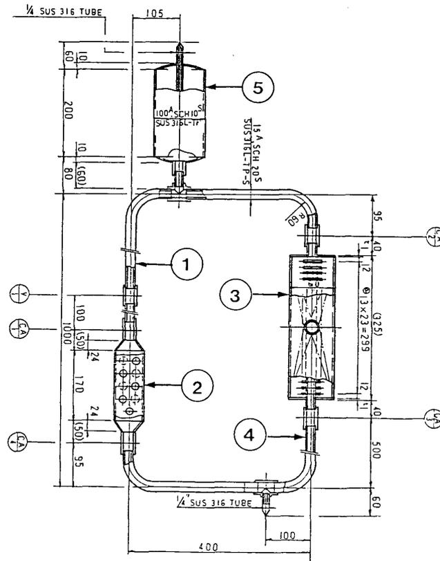
Fig. 3. Schematic diagram of looped type heat pipe employing NaK as working fluid.
