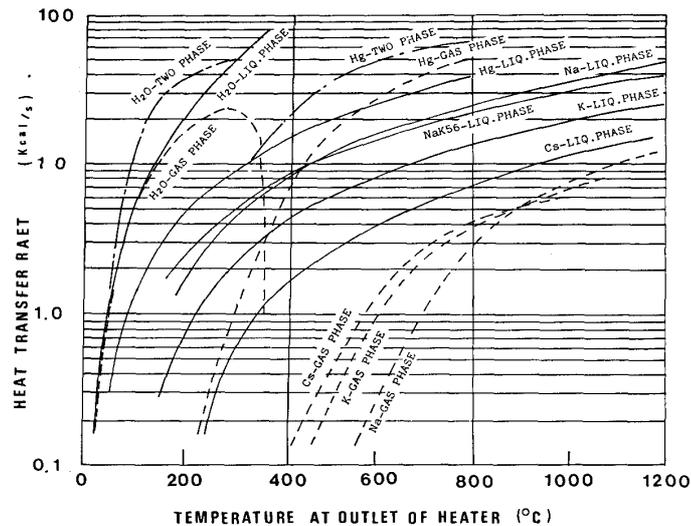
Fig. 2. The calculated heat transfer rate of the looped type that pipe.
