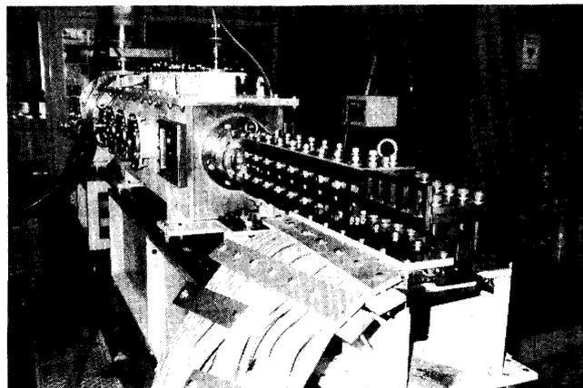
Fig. 2. 95 cm railgun attached to a vacuum chamber
