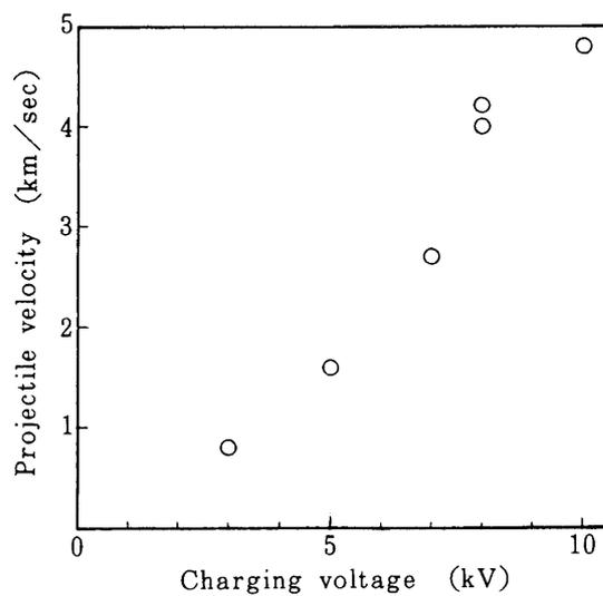
Fig. 10. Projectile velocity versus charging voltage of the capacitor bank
