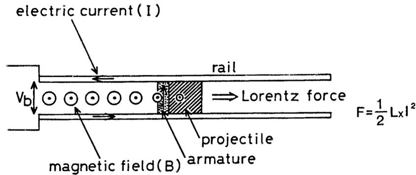
Fig. 1. Principle of railgun
