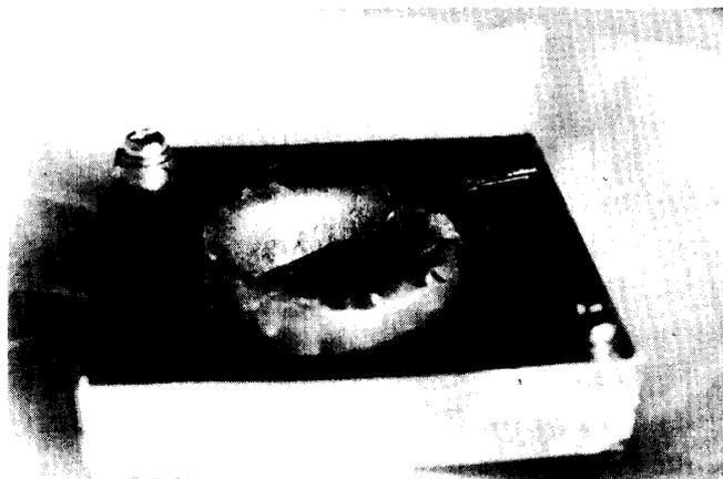
Fig. 11. An crater on an aluminum plate by projectile collision for velocity 3.7 km/sec.
