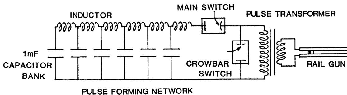
Fig. 6. Circuit diagram of power supply
