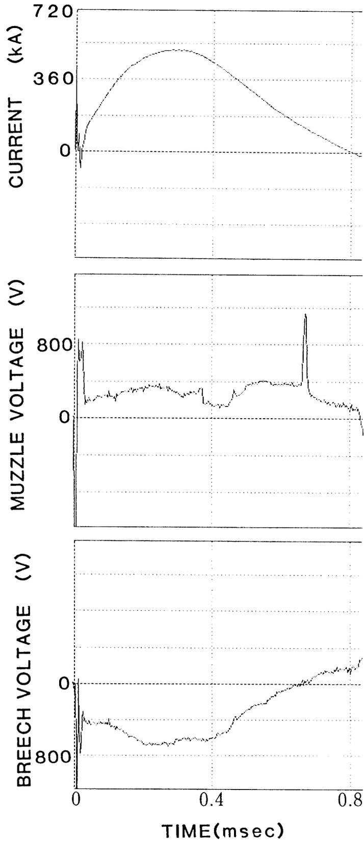
Fig. 9. Total current, breech voltage, and muzzle voltage of one shot
