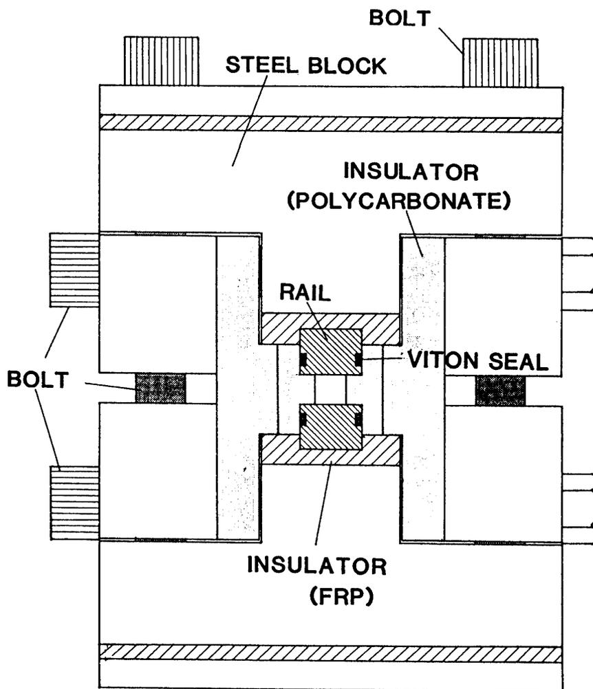
Fig. 4. Cross section of 95 cm railgun
