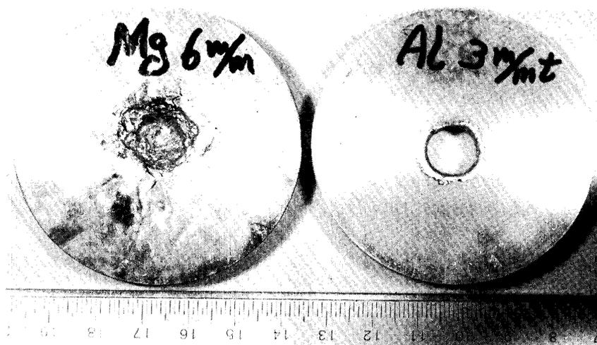
Fig. 15. The pictures of the penetrated aluminum plate of 3.0 mm in thickness (right) and the damaged Mg stopper (microcrater).
