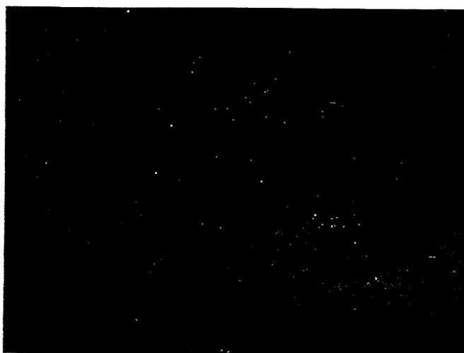
Fig. 4. An XMA distribution pattern of iron at the same region. The white dots occupied the dark area of aluminum distribution.
