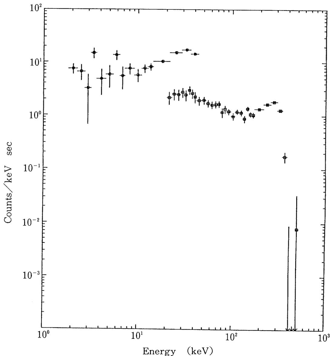
Fig. 2. The energy loss spectrum of the burst of artificial origin. Circles and squares are pulse-height distributions of the proportional counter and the NaI (TI) counter respectively. Discontinuity around 20 keV is evidence for charged particle incidence.
