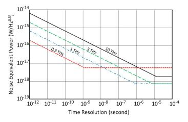
**Figure 1.** Requirements to NEP for photon counting as a function of detector time resolution at 0.3 THz, 1 THz, 3 THz and 10 THz. Spectral resolutions are  $\nu/\Delta\nu = 3$  for all frequencies. The horizontal levels at low time resolution side indicate the background limited NEPs (Matsuo and Ezawa 2016).
