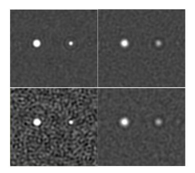
**Figure 3.** Simulated synthesized images of double stars for amplitude (left) and intensity (right) interferometry. amplitude interferometry is with 10 GHz bandwidth and 60 sec integration, and intensity interferometry is with 100 GHz bandwidth and 600 sec integration. Path length fluctuation of 50  $\mu$ m and 100  $\mu$ m are introduces in top two and bottom two images, respectively. Intensity interferometry have blurred image due to lower signal-to-noise ratio at longer baselines.
