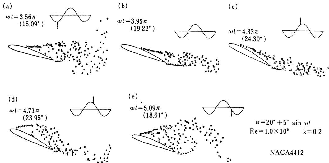
Fig. 11. Flow pattern around pitching airfoil (NACA4412)
