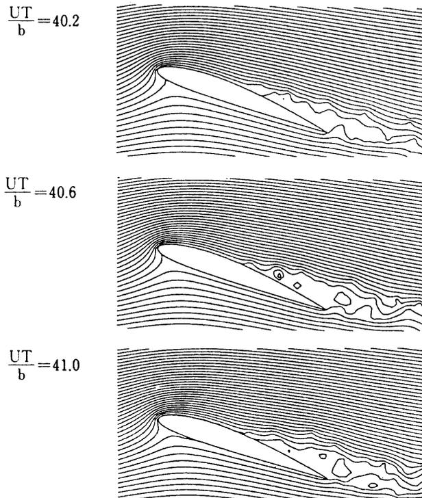
Fig. 3. Stream lines (NACA4412,  $\alpha = 20^\circ$  and  $Re = 3.1 \times 10^6$ )
