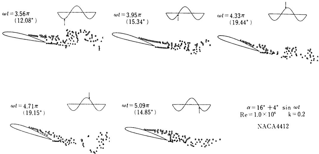
Fig. 7. Flow pattern around pitching airfoil (NACA4412)
