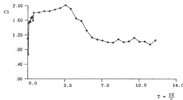
Fig. 16. Time histories of  $C_l$  of wing section under abrupt increase of attack angle (NACA4412)
