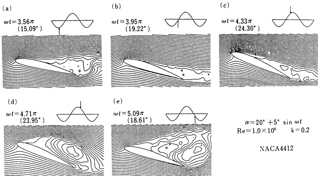
Fig. 12. Stream lines around pitching airfoil (NACA4412)
