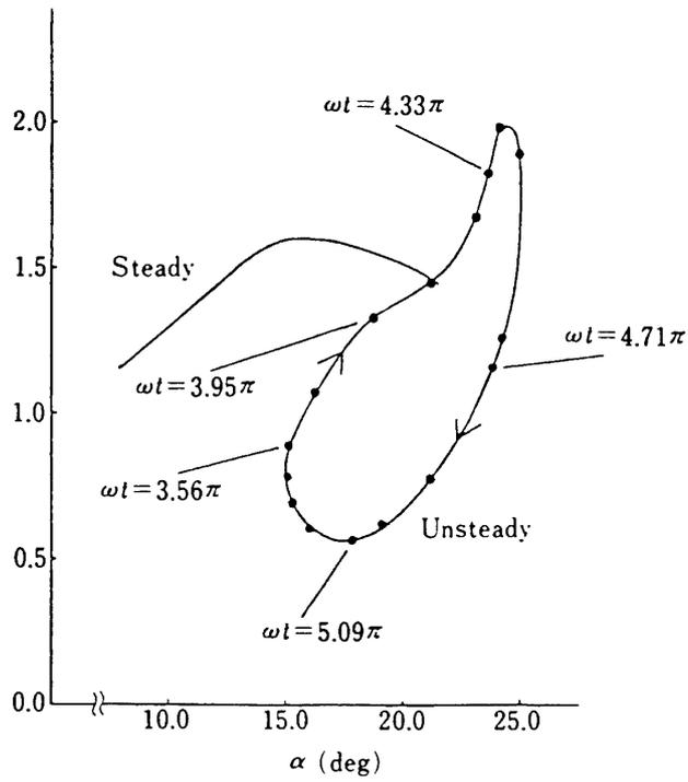
Fig. 13. Hysteresis of  $C_l$  of pitching airfoil (NACA4412)
