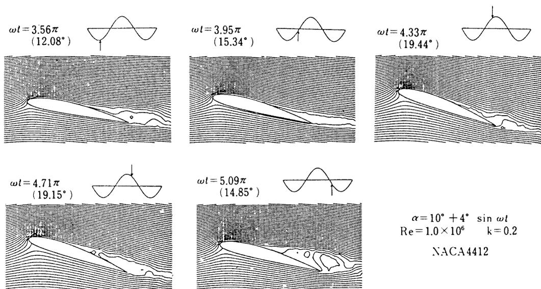
Fig. 8. Stream lines around pitching airfoil (NACA4412)
