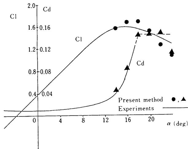
Fig. 5. Comparison of  $C_l$  and  $C_d$  curves with experiments (NACA4412)
