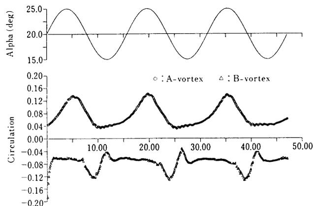
Fig. 10. Temporal change of attack angle and strength of shed vortex of pitching airfoil (NACA4412)
