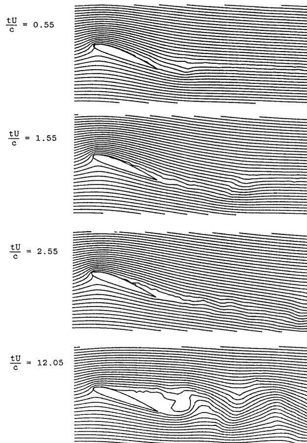
Fig. 15. Transient stream lines around wing section under abrupt increase of attack angle (NACA4412)
