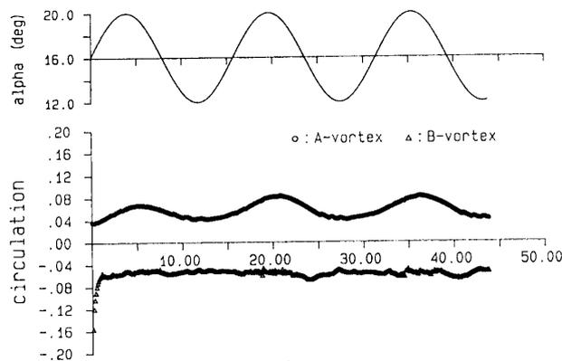
Fig. 6. Temporal changes of attack angle and strength of shed vortex of pitching airfoil (NACA4412)
