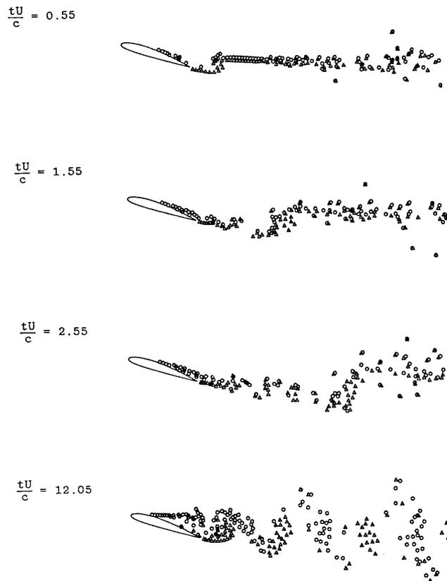
Fig. 14. Transient flow patterns around wing section under abrupt increase of attack angle (NACA4412)
