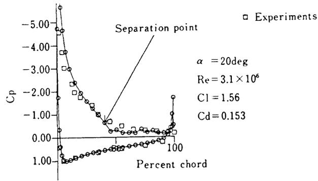
Fig. 4. Pressure distribution (NACA4412,  $\alpha = 20^\circ$ )
