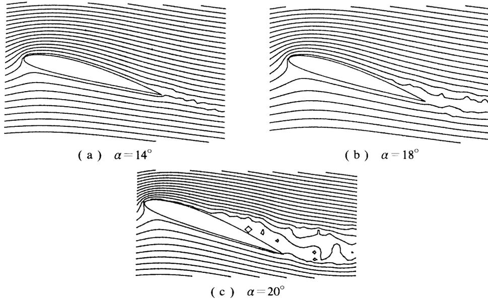
Fig. 2. Flow pattern (NACA4412)
