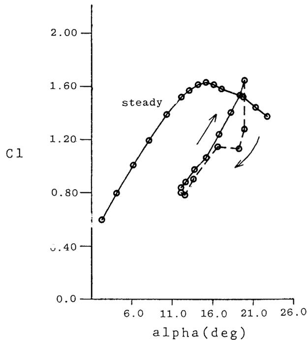
Fig. 9. Hysteresis of  $C_l$  of pitching airfoil (NACA4412)
