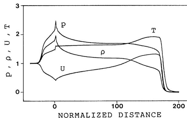
Fig. 4. Distributions of normalized pressure, density, temperature and velocity along the wall surface in case.
