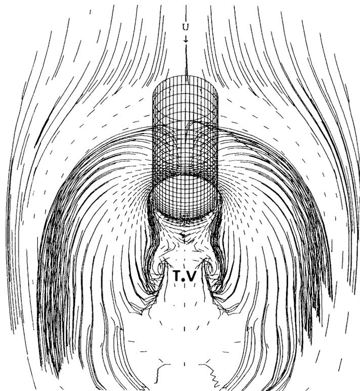
Fig. 6. Surface streamline on the flat vlate:  $Re=1800$ ,  $t=8.79$ .
