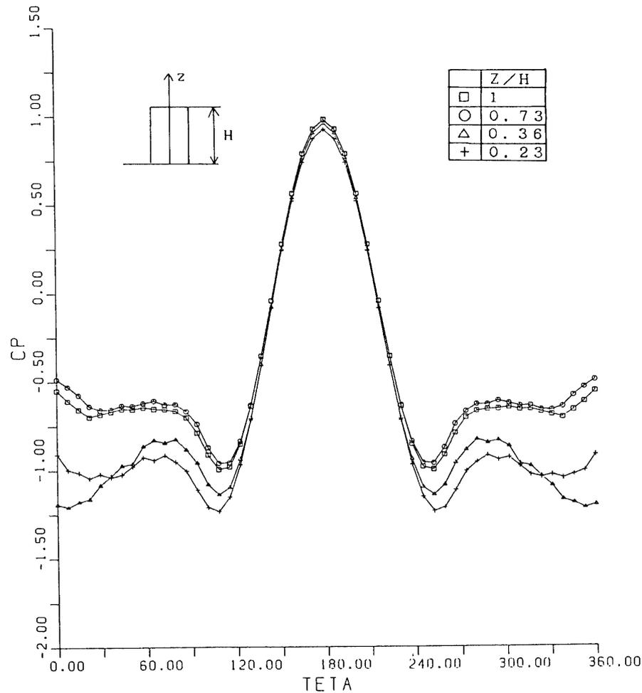
Fig. 9.  $C_p$  Distribution along cylinder surface.
