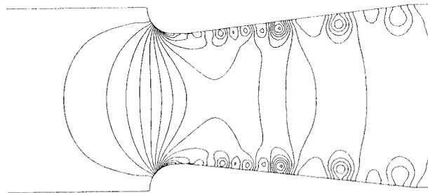
Fig. 11. Pressure contour in venturi by HSMAC scheme:  $T = 2.5$
