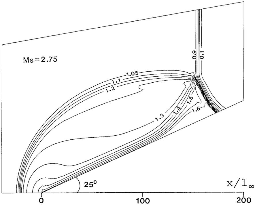
Fig. 3(b). Temperature contours  $(T - T_1)/(T_2 - T_1)$  in case.
