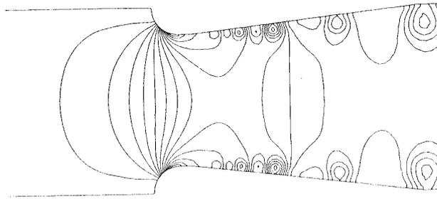
Fig. 10. Pressure contour in venturi by HSMAC scheme:  $Re = 20000$
