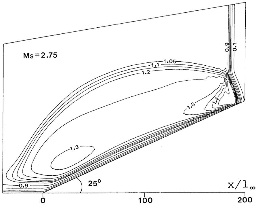
Fig. 2(b). Temperature contours  $(T - T_1)/(T_2 - T_1)$  in case.
