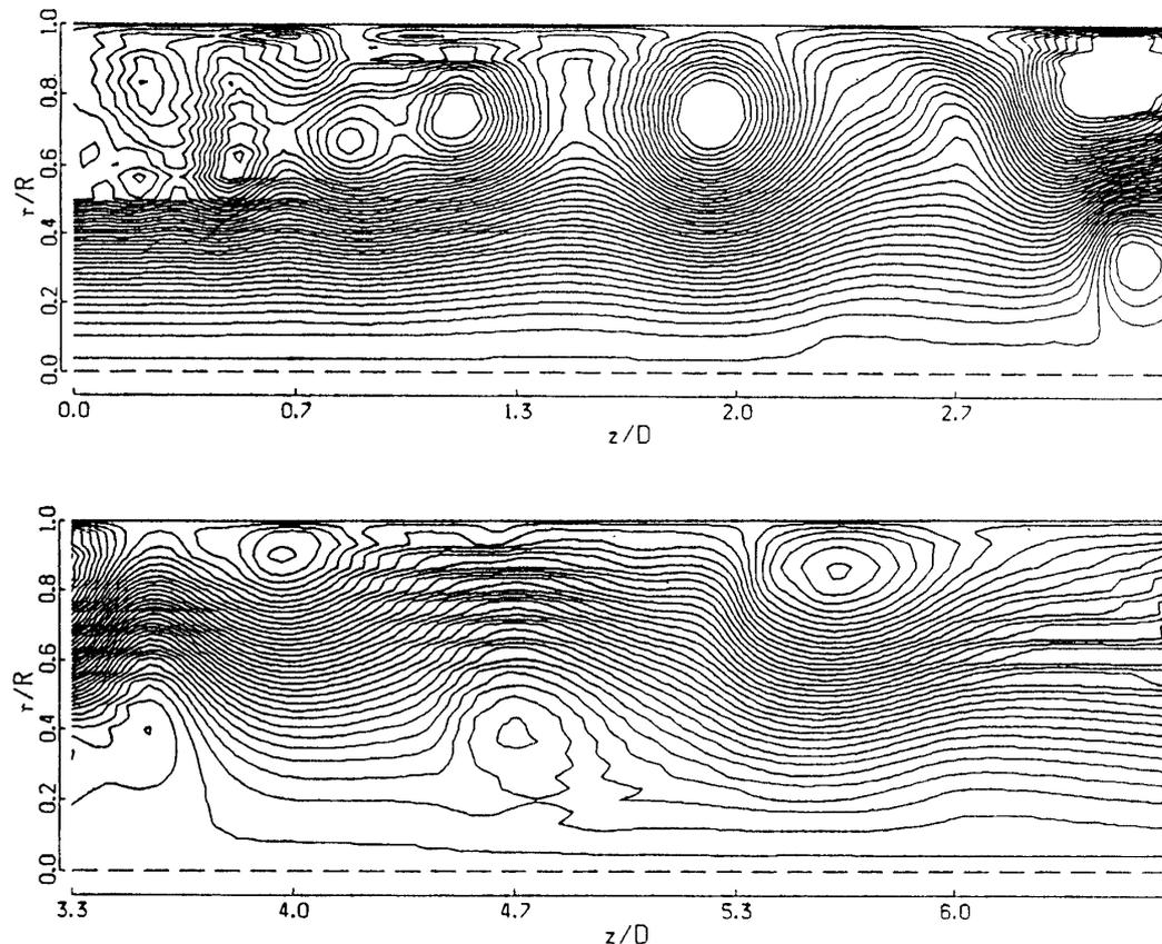
Fig. 19. Flow patterns after impulsively started from the rest condition with swirling velocity, the Reynolds number is 50000.
