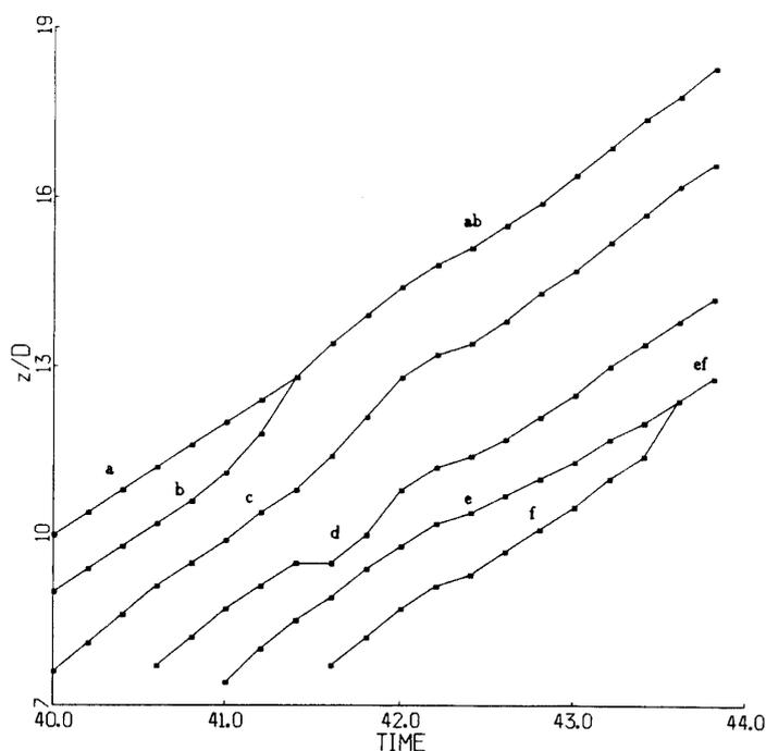
Fig. 8. History of vortices position by numerical simulation at  $Re=3000$ .
