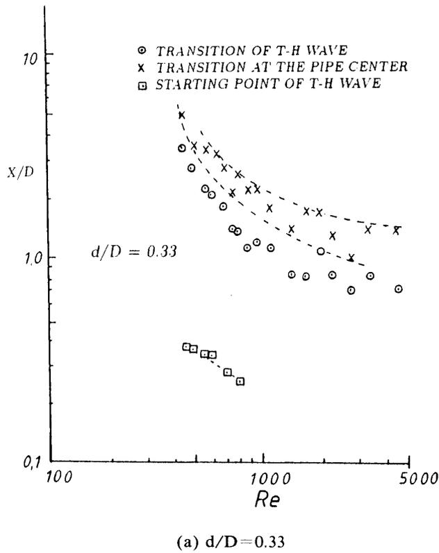
Fig. 11. Experimental data of breakdown-transition.
