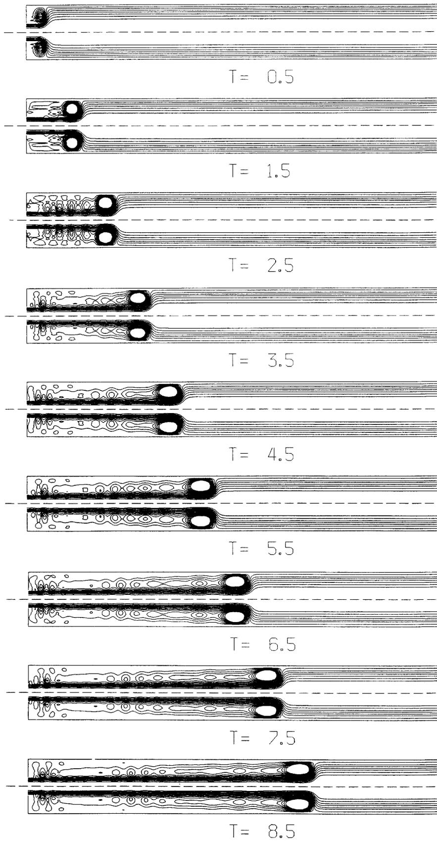
Fig. 2. Flow patterns after impulsively started from the rest condition, the Reynolds number is 2000.
