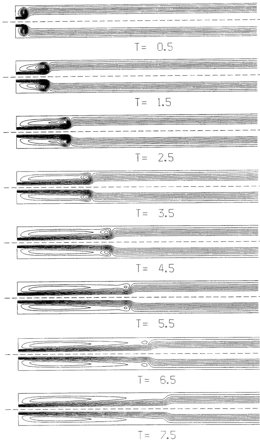
Fig. 1. Flow patterns after impulsively started from the rest condition, the Reynolds number is 100.
