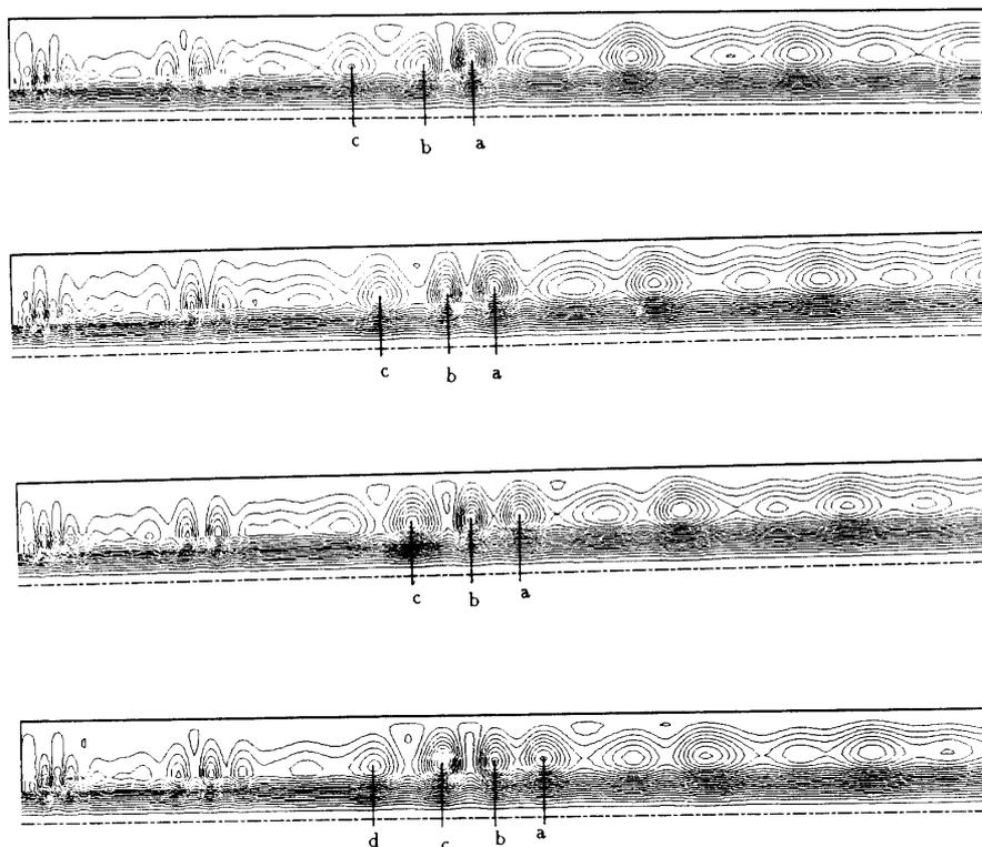
Fig. 7. The processes of vortex shedding and pairing at  $Re = 3000$ .
