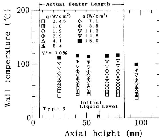
Fig. 6. Heater wall temperature distributions.
