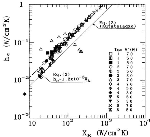
Fig. 7. Comparison of measured data with Kutateladze's correlation as for boiling heat transfer coefficient.
