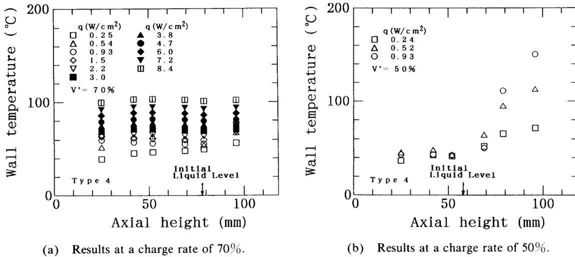
Fig. 5. Heater wall temperature distributions.
