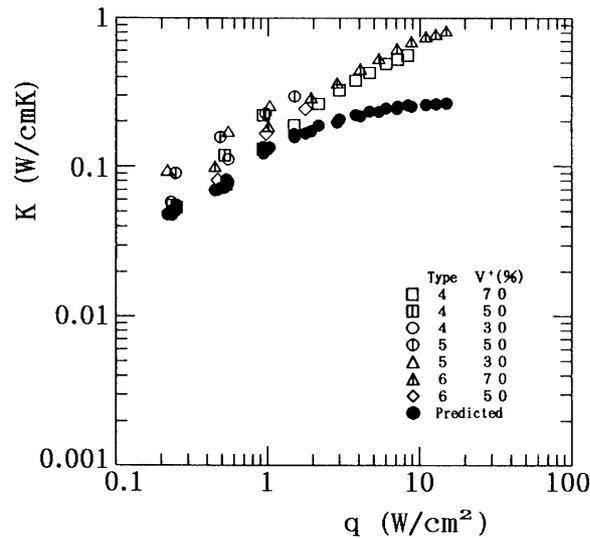
Fig. 8. Comparison of measured with predicted results as for overall coefficient of heat transmission.
