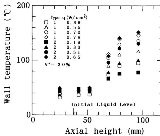
Fig. 3. Heater wall temperature distributions (Type 1 and 2).
