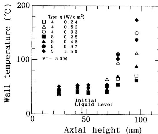
Fig. 4. Heater wall temperature distributions (Type 4 and 5).
