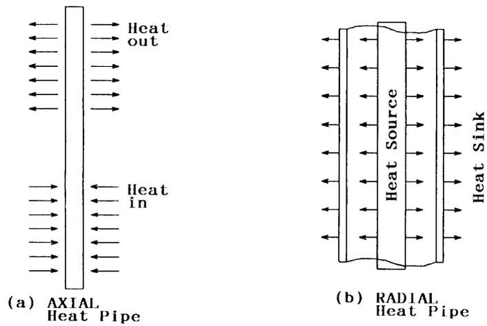
Fig. 1. Conception of radial heat pipe.
