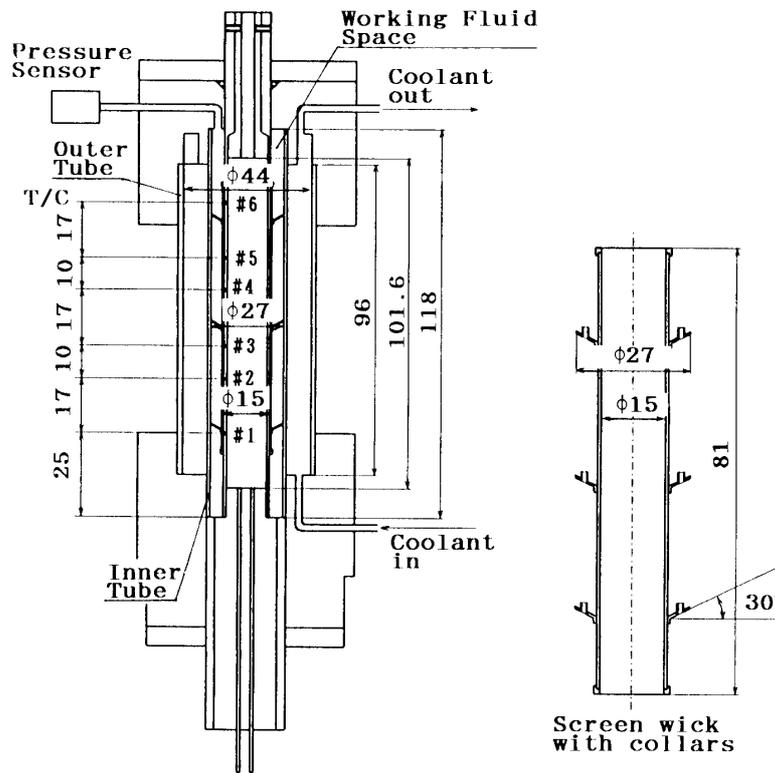
Fig. 2. Experimental apparatus.
