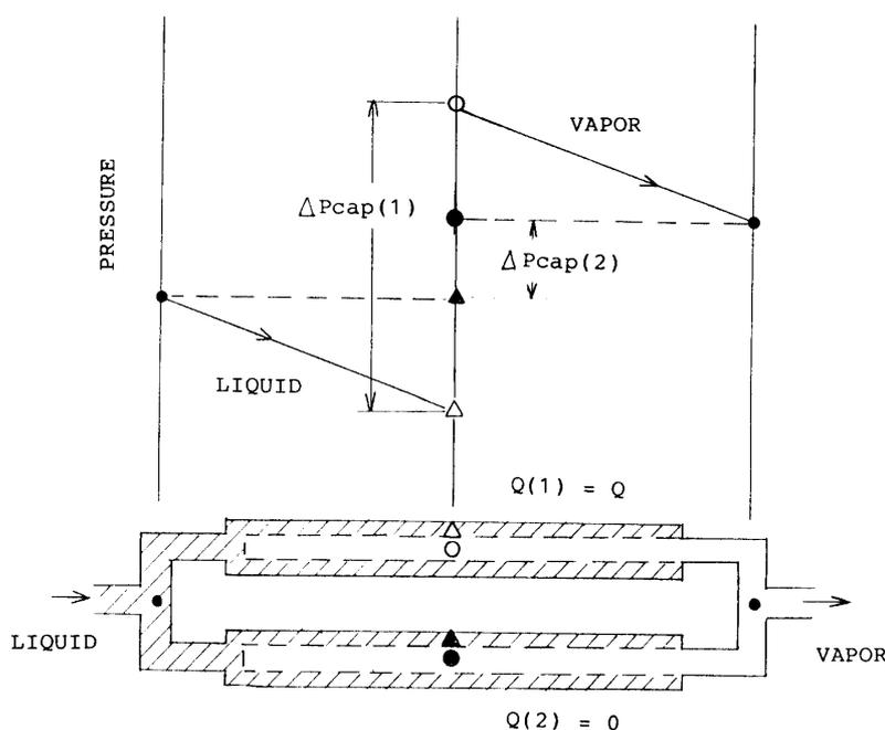
Fig. 9. Desirable Pressure Profile.
