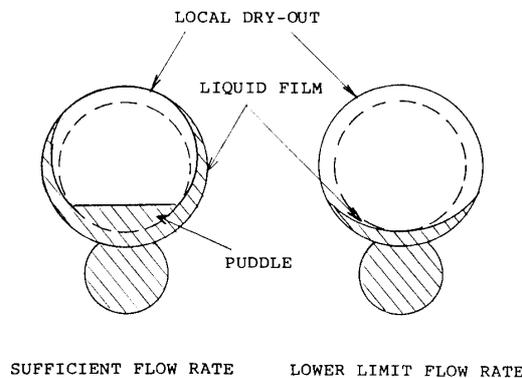
Fig. 5. Liquid Behavior in Evaporator.
