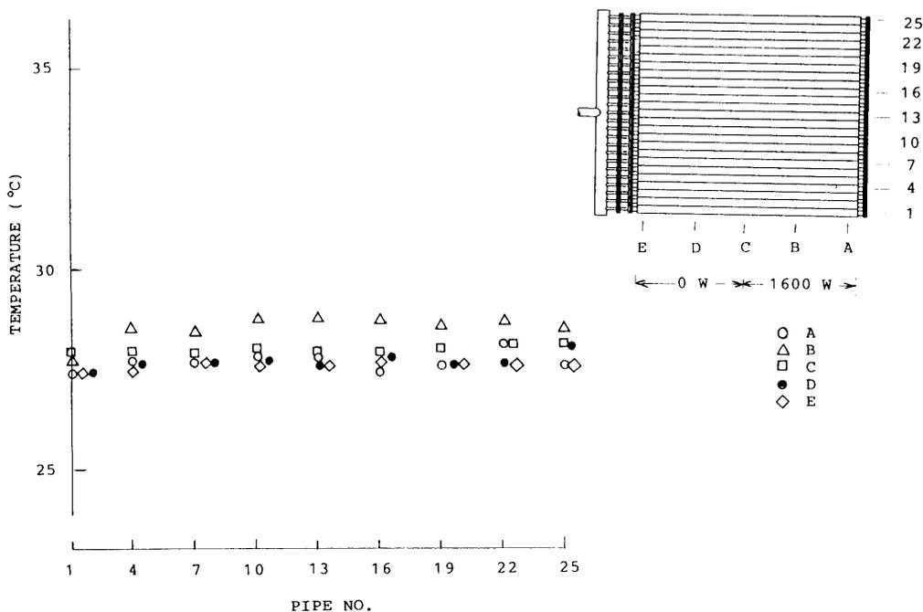
Fig. 8. Test Results of Uneven Heat Load along the Cold Plate
