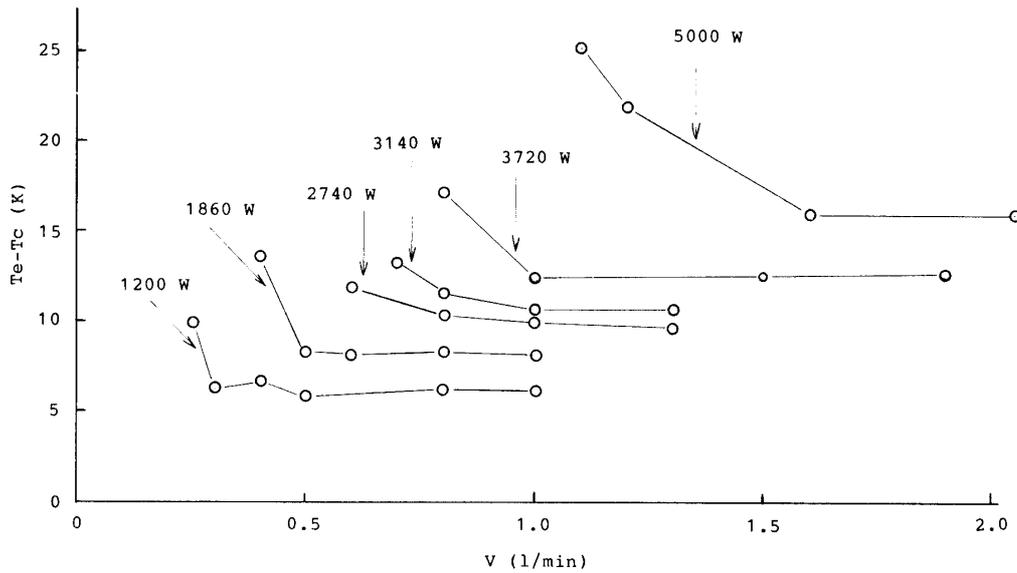
Fig. 4. Heat Transfer Characteristics
