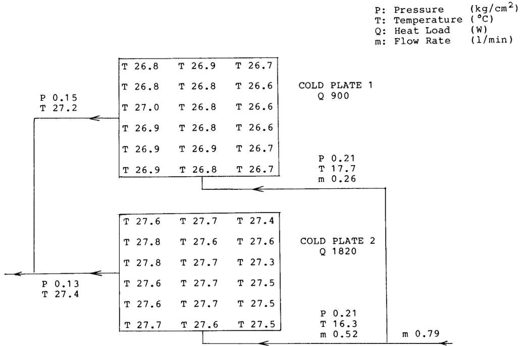
Fig. 11. Test Result of Parallel Operation
