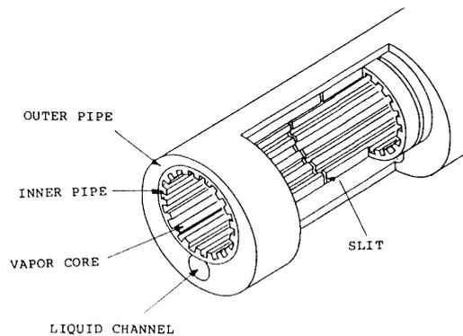
Fig. 1. Grooved Double Pipe Heat Pipe
