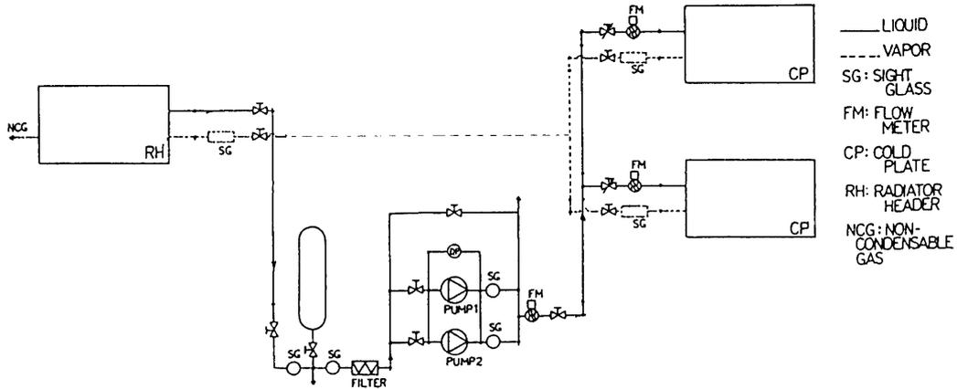
Fig. 10. Schematic Diagram of Parallel Operation Test Loop
