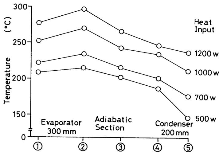
Fig. 3. Temperature distribution in horizontal mode.
