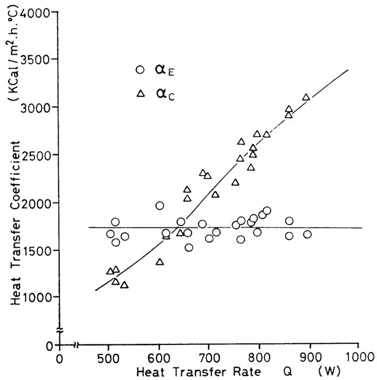
Fig. 9. Heat transfer coefficient in horizontal mode.
