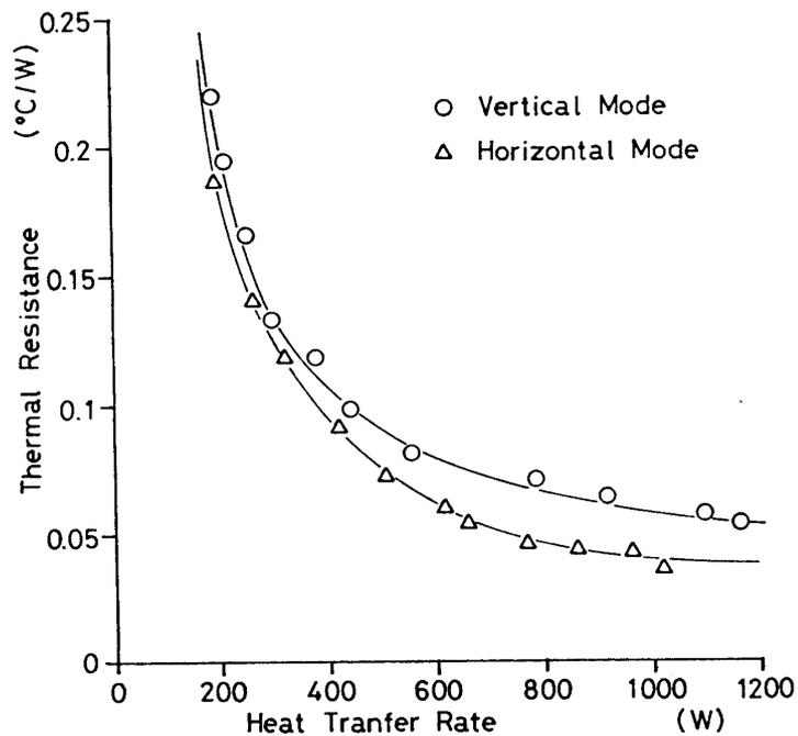
Fig. 5. Thermal resistance.
