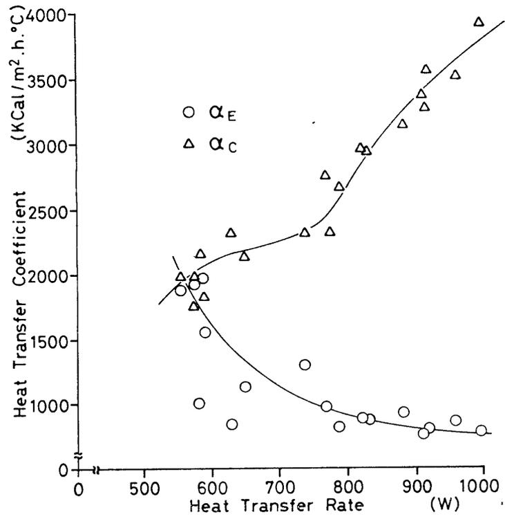
Fig. 8. Heat transfer coefficient in vertical mode.
