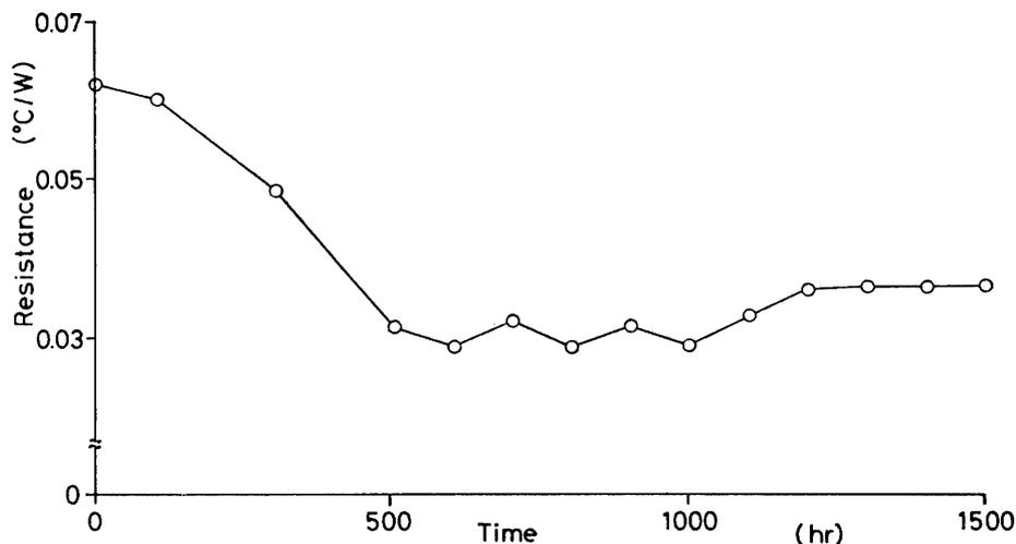
Fig. 10. Variation of thermal resistance during life test.
