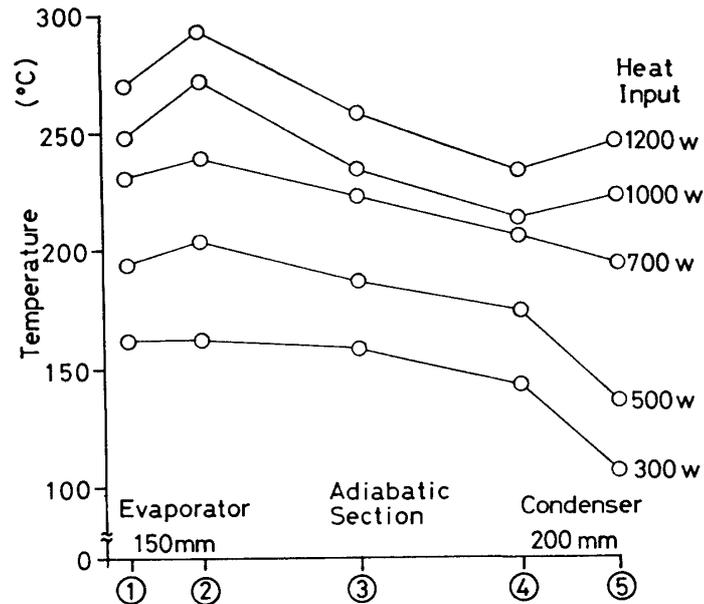
Fig. 4. Temperature distribution in horizontal mode with shortened heater.
