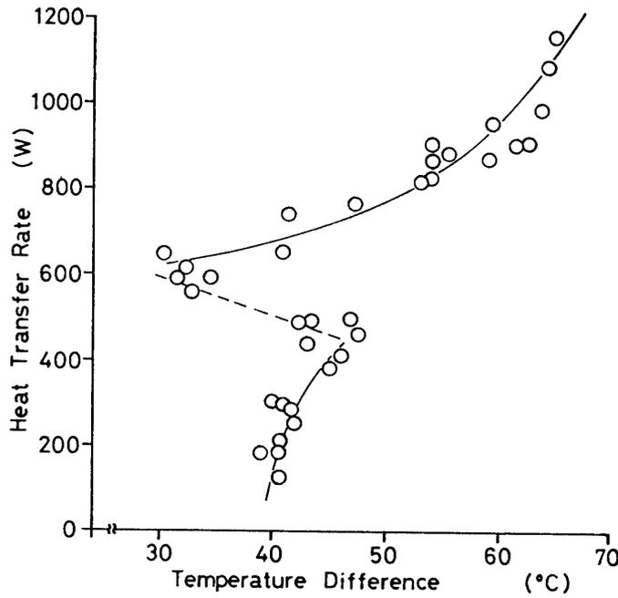
Fig. 6. Heat transfer rate in vertical mode.
