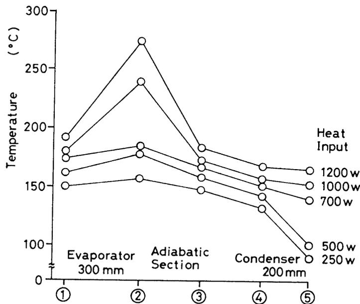
Fig. 2. Temperature distribution in vertical mode.
