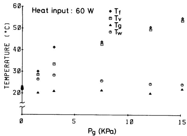
Fig. 4. Temperature distributions with partial pressure of non-condensable gas.
