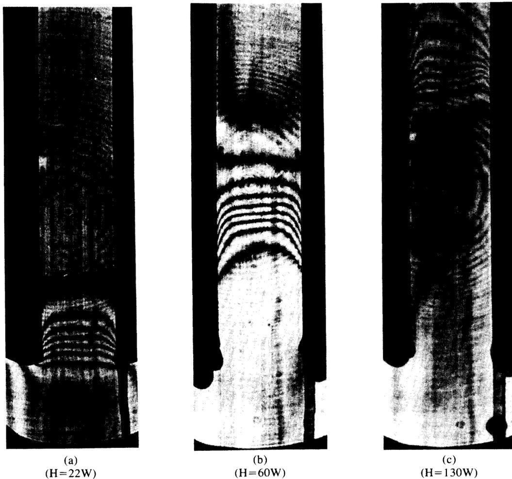
Fig. 8. Movement of interfacial layer according to heat input rate.
