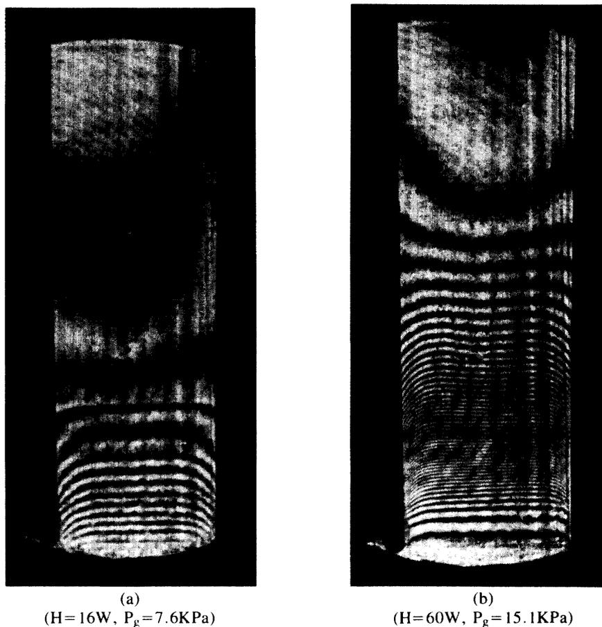
Fig. 7. Density contour figure pattern of condensation section.
