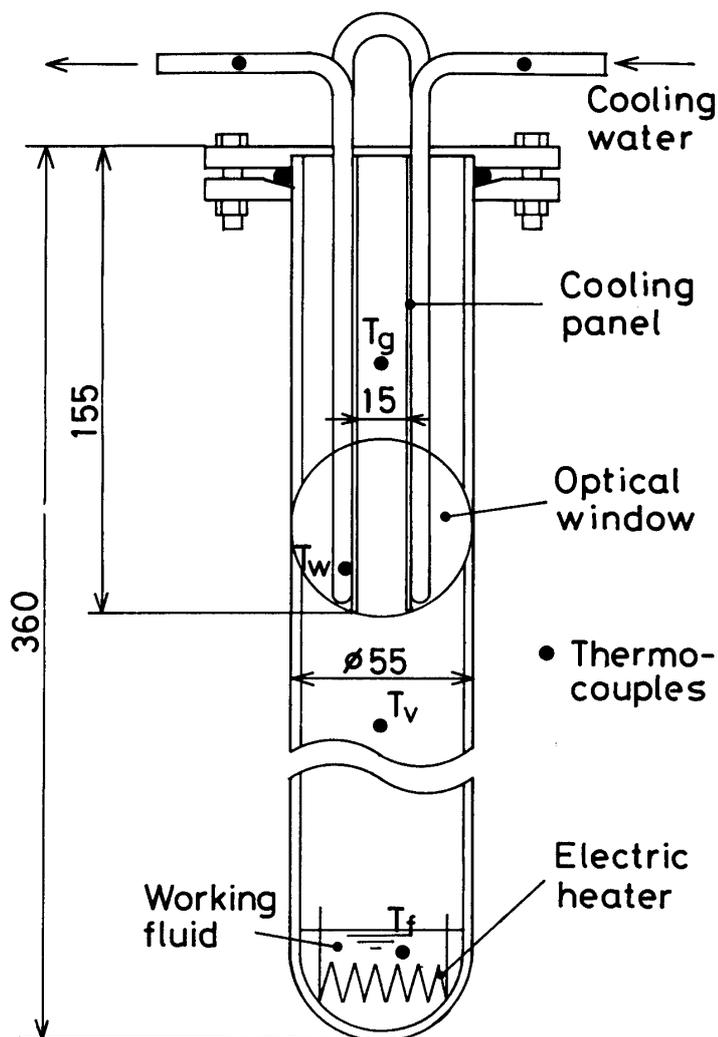
Fig. 1. Schematic view of the thermosyphon model.
