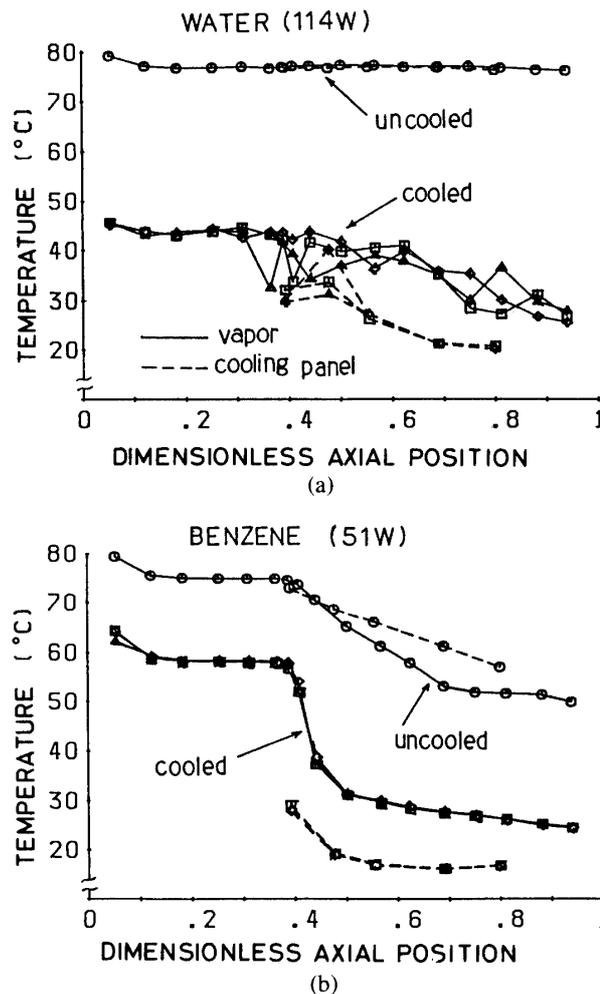
Fig. 2. Axial temperature distributions in thermosyphon.
