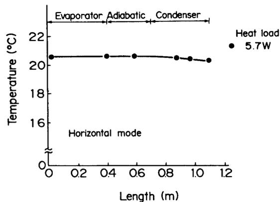
Fig. 9. Axial temperature distribution of the FCHP.
