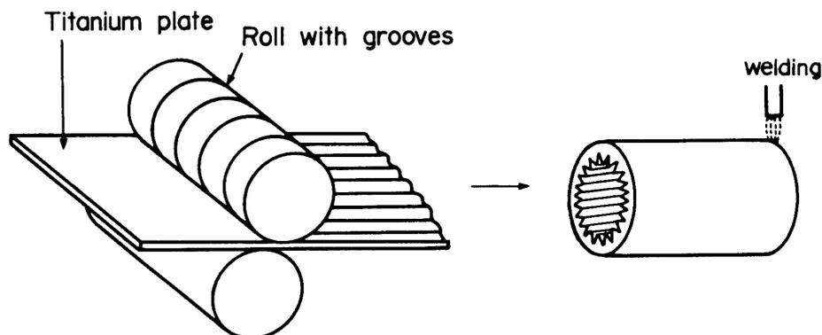
Fig. 3. Pipe fabrication process.
