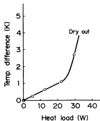
Fig. 10. FCHP characteristic curve.
