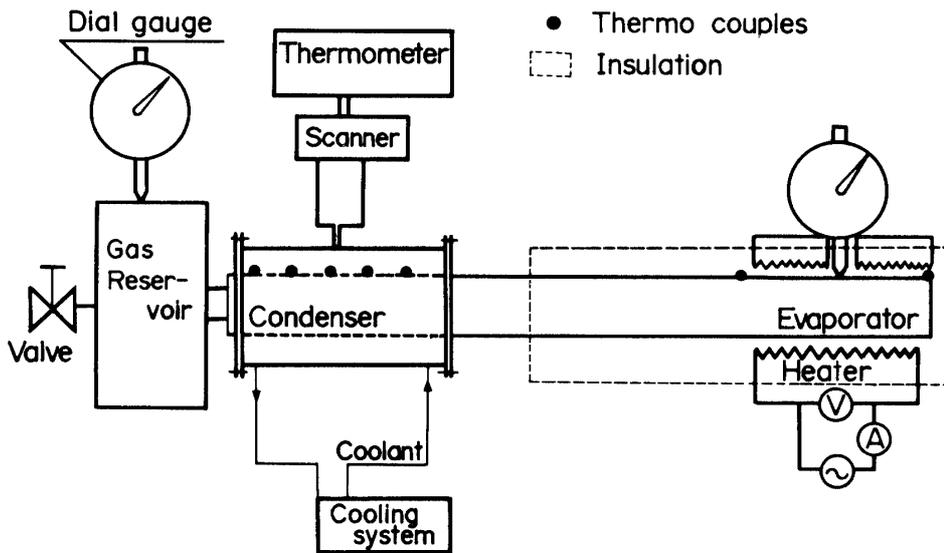
Fig. 7. Sketch of the Apparatus.
