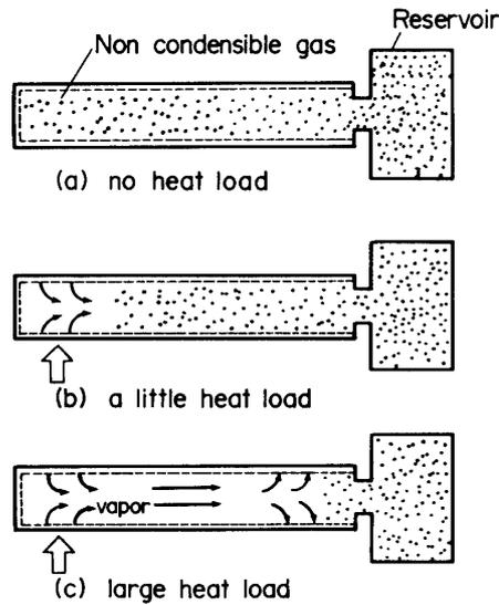
Fig. 1. Non-condensable gas control principle.
