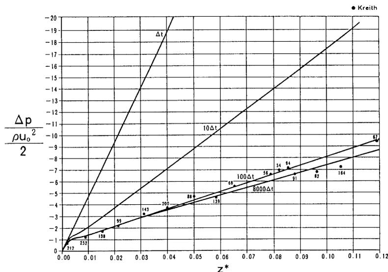
Fig. 10. Pressure Drop,  $Re=100$ , on wall.
