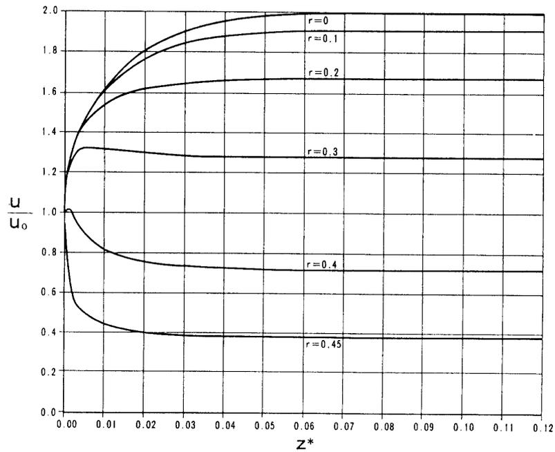
Fig. 7. Velocity Distribution, Re=2000, steady state.
