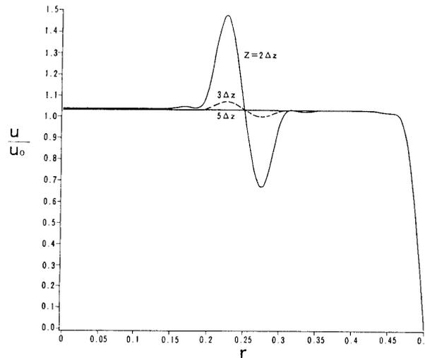
Fig. 16. Velocity Distribution with Disturbances,  $Re=2000$ ,  $T=10*\Delta t$ .
