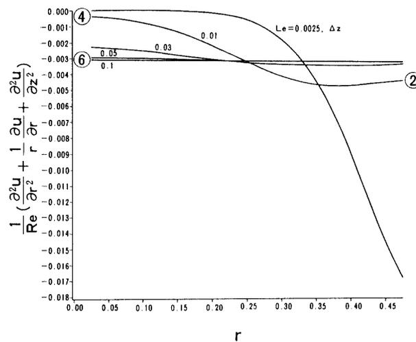
Fig. 15. Axial Viscous Term,  $Re = 10000$ .
