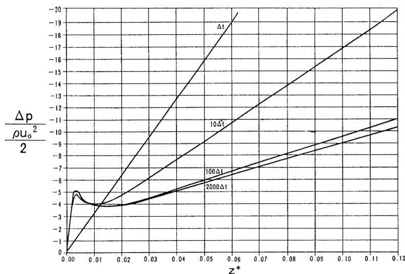
Fig. 9. Pressure Drop,  $Re=10$ , on wall.
