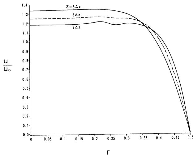
Fig. 18. Velocity Distribution with Disturbances,  $Re=2000$ ,  $T=500*\Delta t$ .
