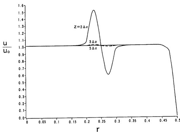
Fig. 19. Velocity Distribution with Disturbances,  $Re=10000$ ,  $T=10*\Delta t$ .
