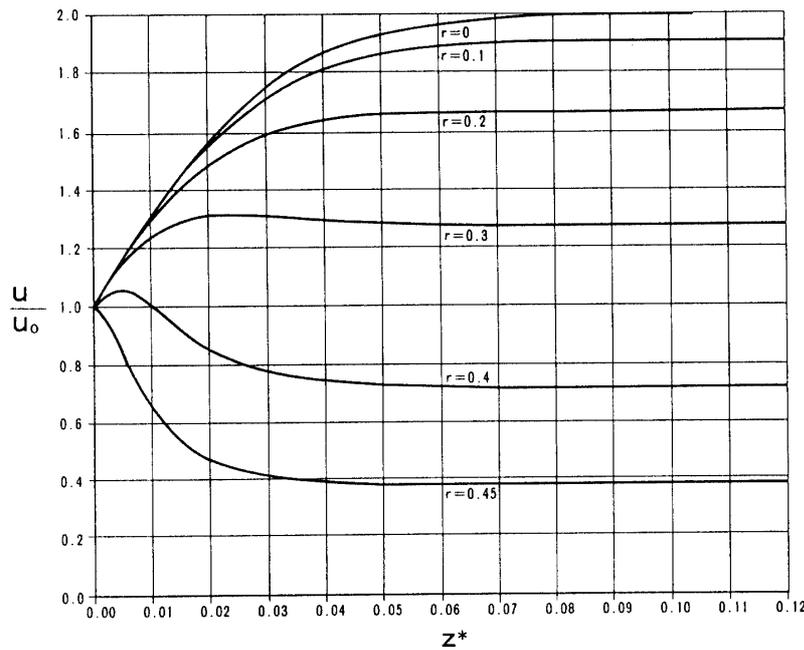
Fig. 5. Velocity Distribution, Re=10, steady state.
