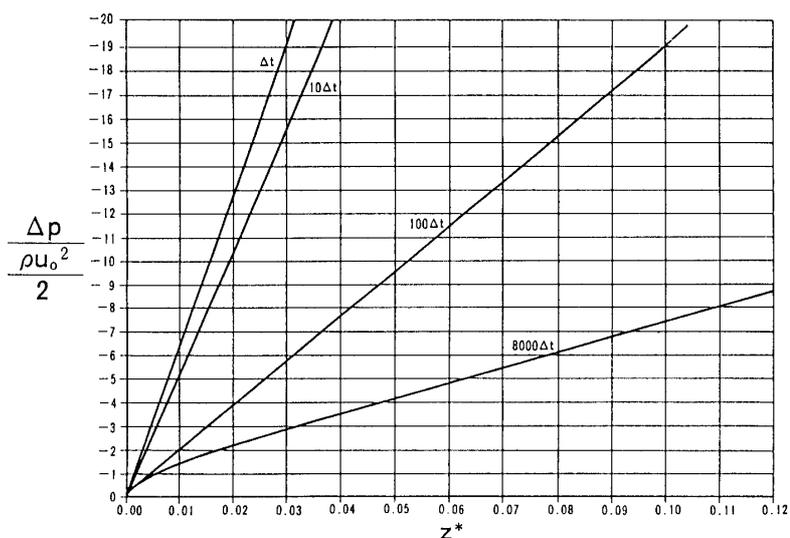
Fig. 11. Pressure Drop,  $Re=2000$ , on wall.
