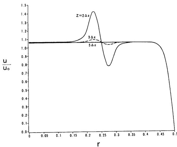
Fig. 20. Velocity Distribution with Disturbances,  $Re=10000$ ,  $T=50*\Delta t$ .
