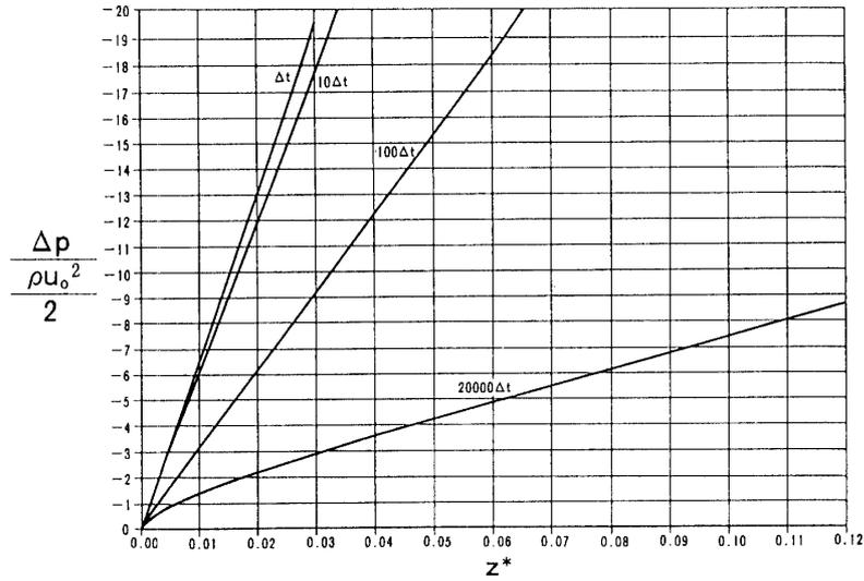
Fig. 12. Pressure Drop, Re=10000, on wall.
