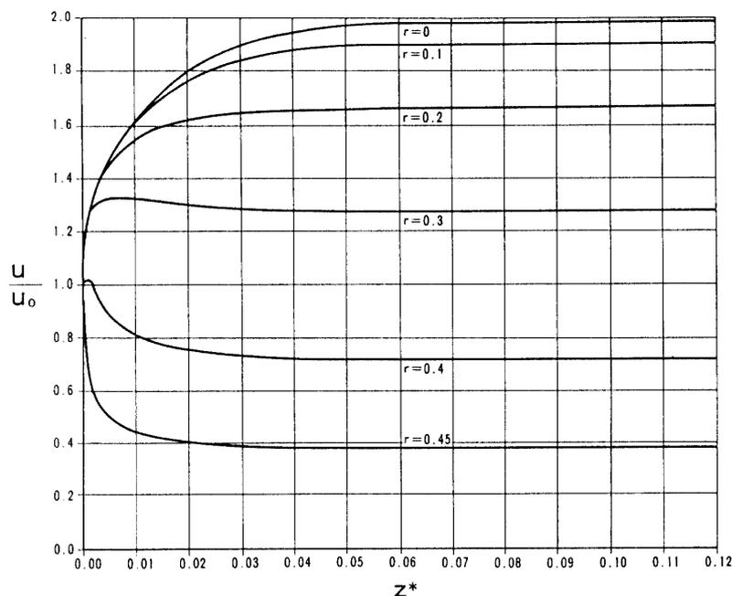
Fig. 8. Velocity Distribution,  $Re=10000$ , steady state.
