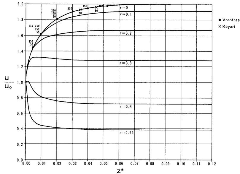
Fig. 6. Velocity Distribution, Re=100, steady state.
