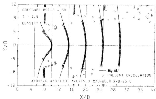
Fig. 4. Comparison of calculated density distributions in  $y$  direction with empirical formula, eq. [8].
