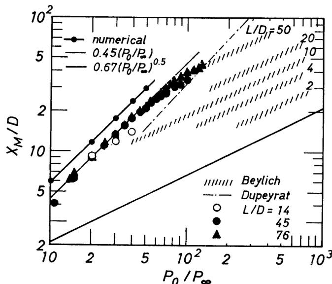
Fig. 6. Reduced normal shock location as a function of pressure ratio: Comparison of calculation with experiments.
