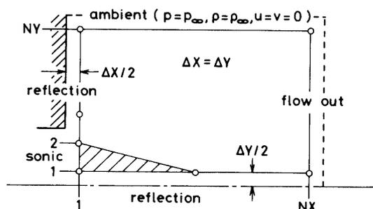
Fig. 1. Calculation region and initial and boundary conditions.
