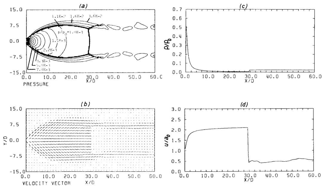
Fig. 2. Numerical results for  $p_0/p_\infty=50$ : (a) Isobars, (b) Velocity vectors, (c) Density profile on jet axis, (d) Velocity profile on jet axis.
