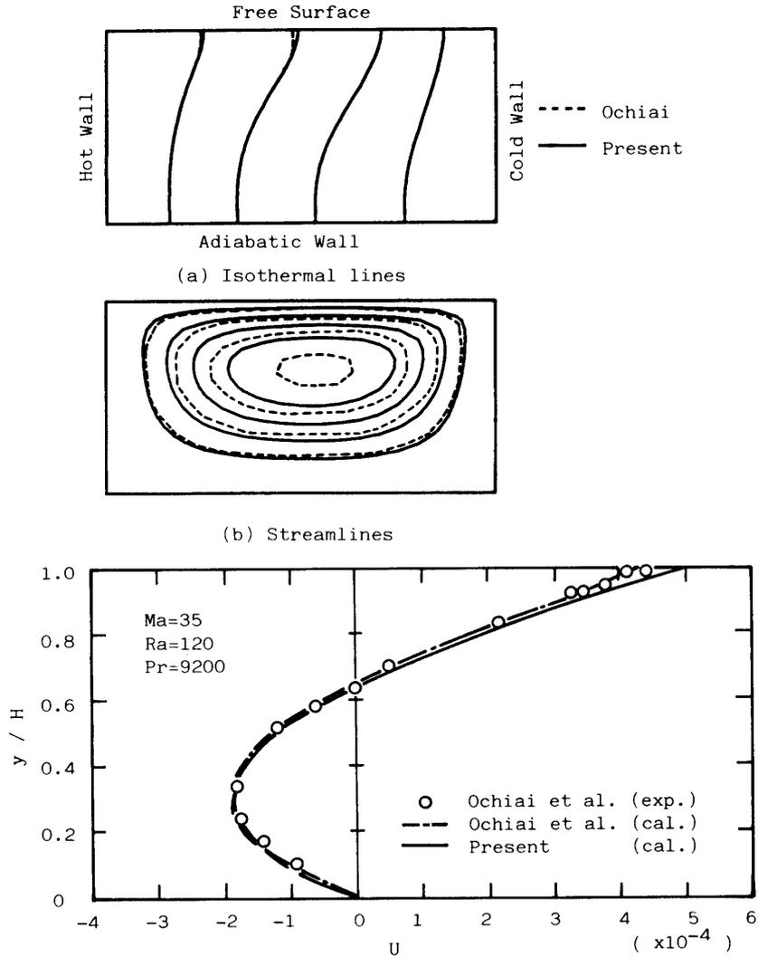
Fig.1(c) Velocity distributions on center vertical plane.
