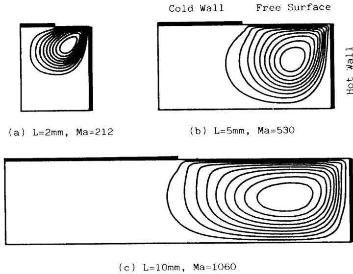
Fig. 4. Streamlines of Marangoni convection in Bridgman method.
