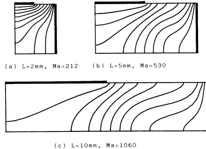
Fig. 5. Isotherms of Marangoni convection in Bridgman method.
