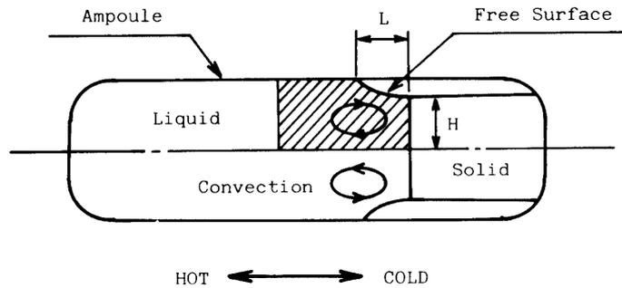
Fig. 2. Concept of Bridgman crystal growth method.
