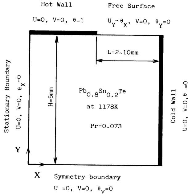
Fig. 3. Boundary conditions for analysis of Marangoni convection in Bridgman method.
