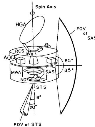
Fig. 1. "SAKIGAKE" and its nutation damper.
