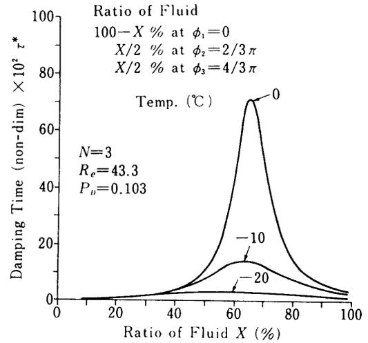
Fig. 6. Damping time as a function of ratio of fluid that is away from the stable point.
