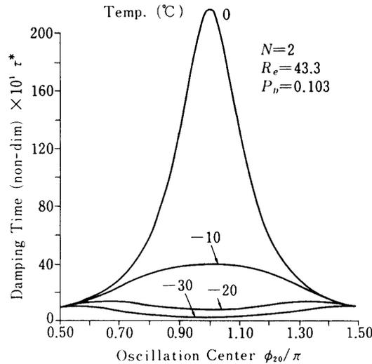
Fig. 7. Damping time as a function of the oscillation center of a generated slug.
