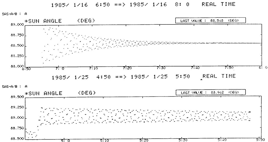
Fig. 2. Examples of damping motion of nutation.
