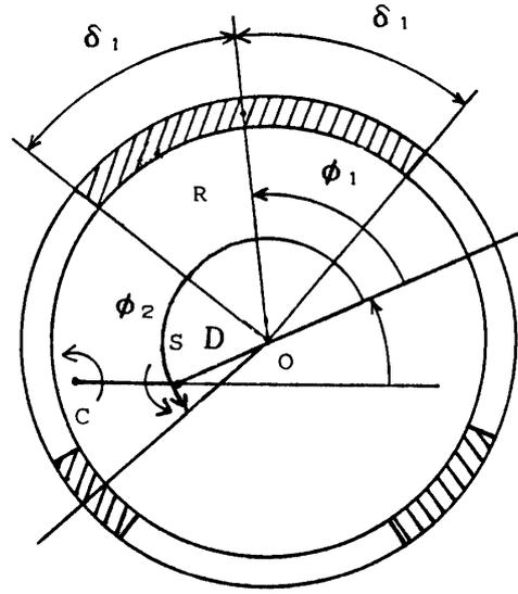
Fig. 4. Schematic view of fluid slugs in nutation damper (cross section A-A).
