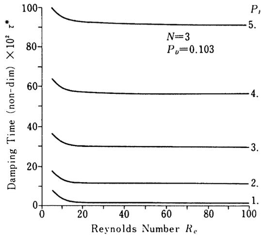
Fig. 10. Damping time as a function of Reynolds Number.
