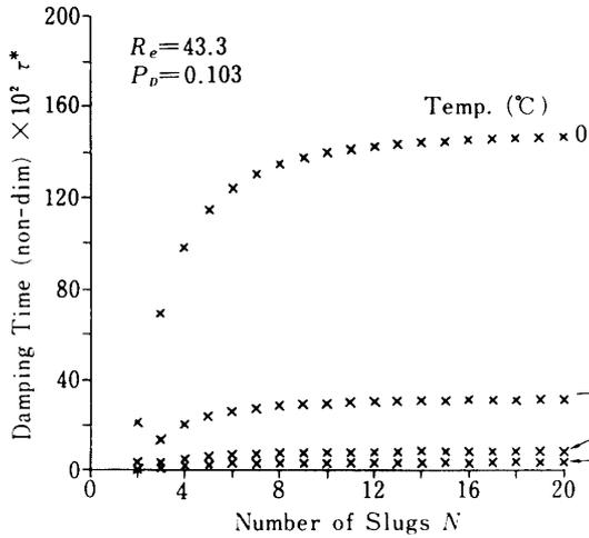
Fig. 5. Damping time as a function of number of slugs.
