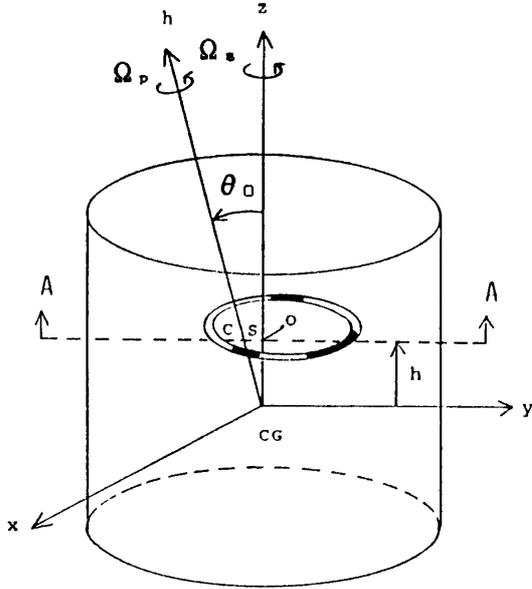
Fig. 3. Satellite and partially filled nutation damper.
