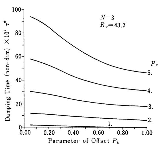
Fig. 9. Damping time as a function of offset.
