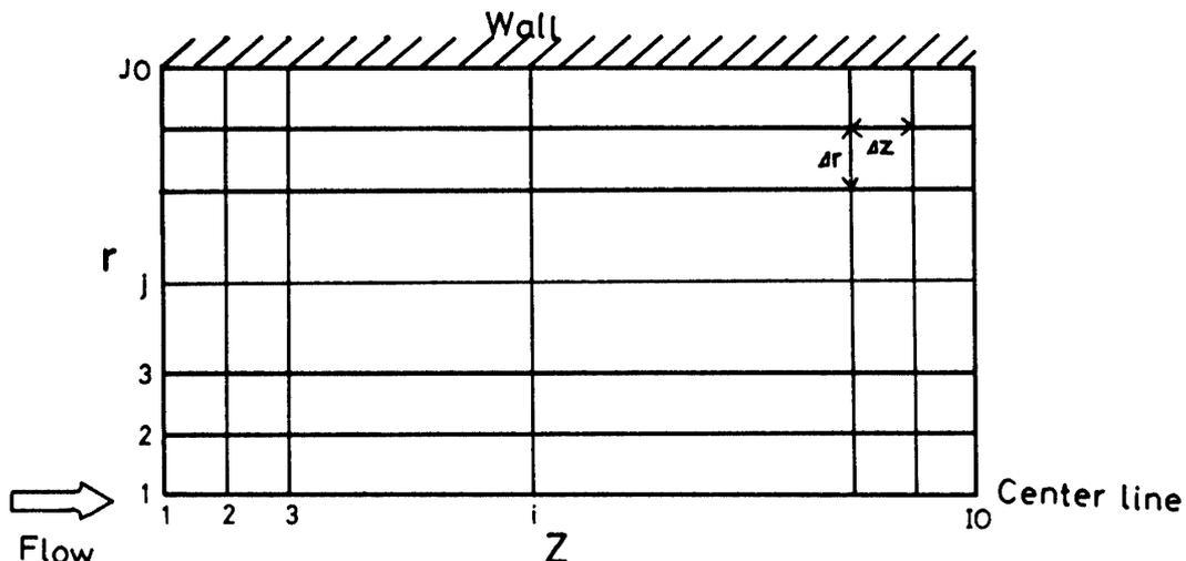
Fig. 3. Mesh system for numerical simulation.
