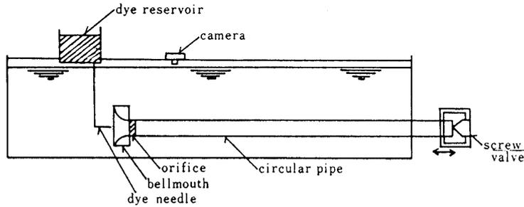
Fig. 1. Schematic diagram of the experimental apparatus.
