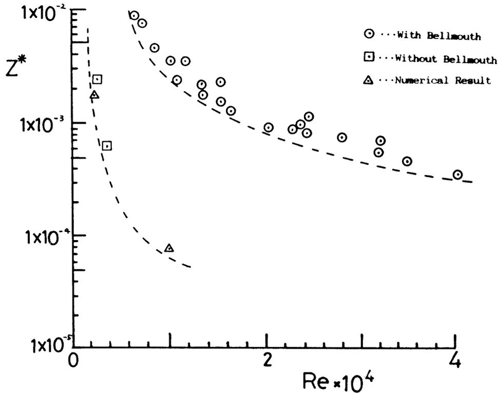
Fig. 9. Relation between the non-dimensional transition length and the Reynolds number with and without bellmouth.
