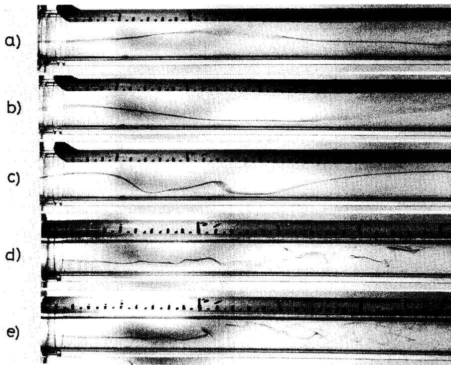
Fig. 5. A series of photographs visualized by tracer of dye for orifice (c).
