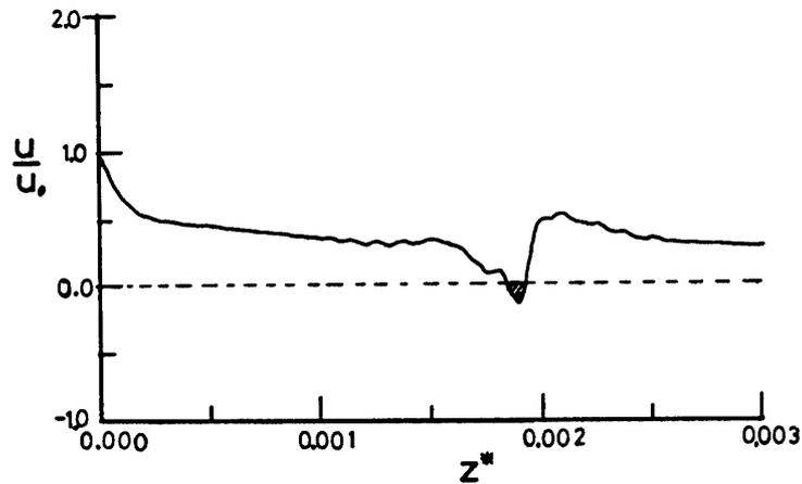
Fig. 7. Velocity variation along the pipe at  $Re=2,700$ .
