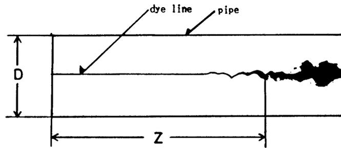
Fig. 2. Sketch of transition flow in the pipe.
