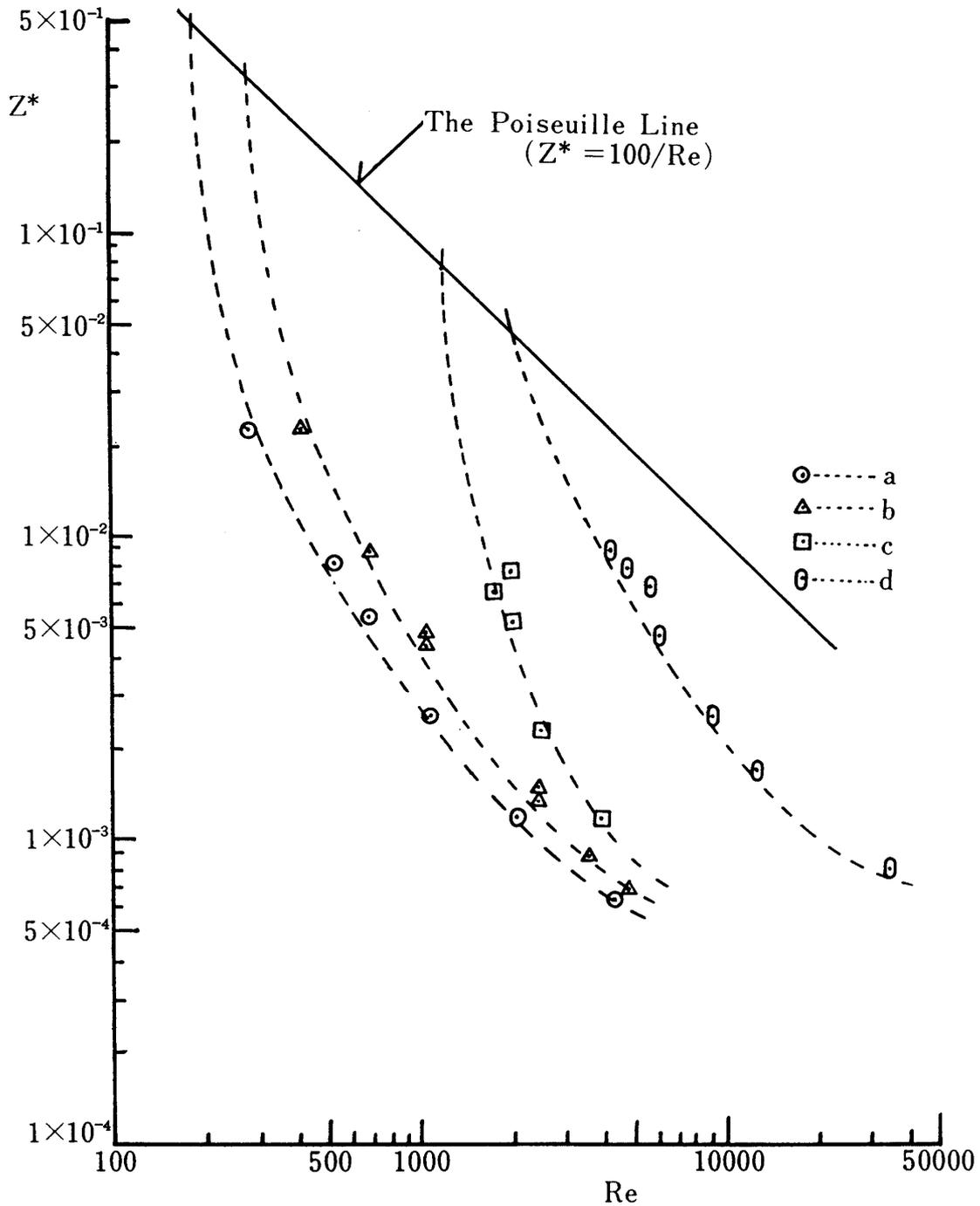
Fig. 6. Relation between the non-dimensional transition length and the Reynolds number.
