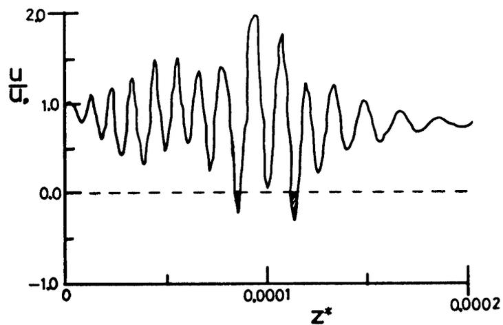
Fig. 8. Velocity variation along the pipe at  $Re=10,000$ .
