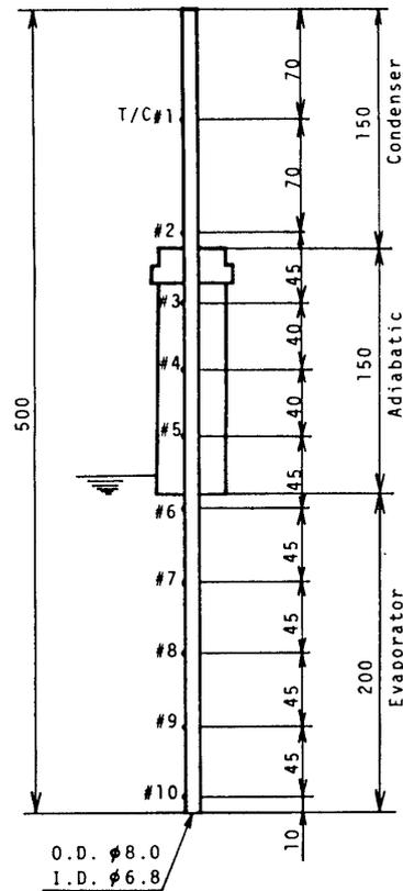
Fig. 1. Dimensions of heat pipe.
