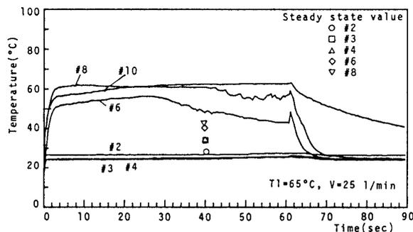
Fig. 4. Transient response at low water bath temperature.
