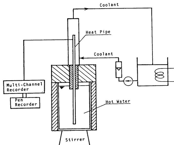
Fig. 2. Schematic diagram of experimental apparatus.
