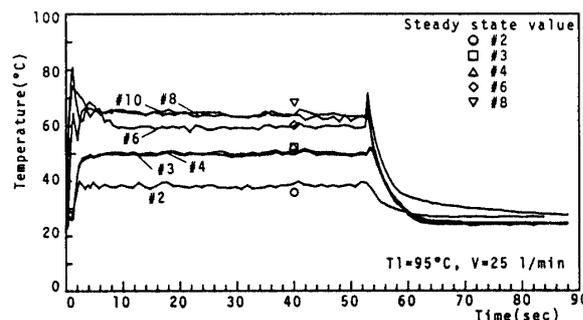
Fig. 3. Transient response at high water bath temperature.
