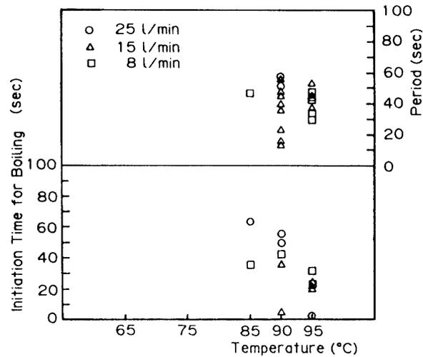
Fig. 8. Initiation time of nucleate boiling and period of temperature fluctuation.
