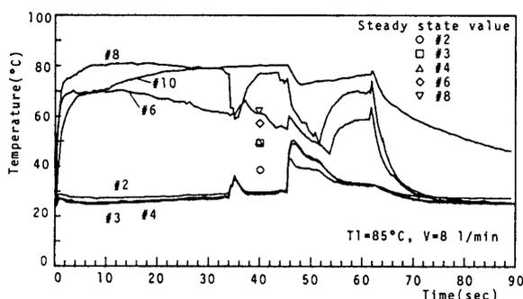
Fig. 5. Transient response at moderate water bath temperature.
