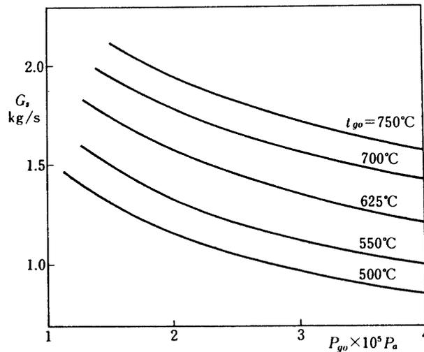
Fig. 6. Variation of  $G_3$  with  $P_{go}$  and  $t_{go}$ .
