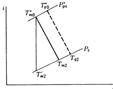
Fig. 4. Expansion process in turbo expander.
