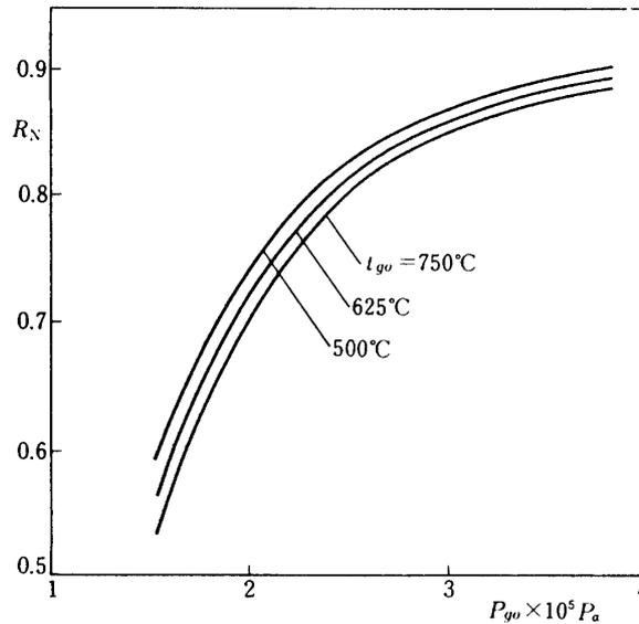
Fig. 9. Variation of ratio of relative power output increase  $R_N$  with  $P_{go}$  and  $t_{go}$ .
