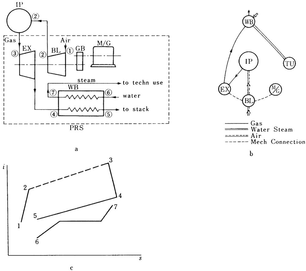
Fig. 1. Scheme of the conventional power recovery energy system (PRS).
