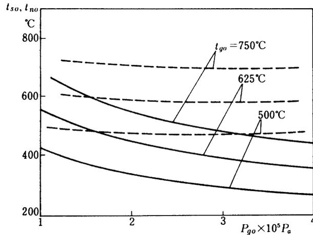
Fig. 5. Variation of  $t_{so}$ ,  $t_{no}$ ,  $t_m$ ,  $t_s$  with  $P_{go}$  and  $t_{go}$ .
