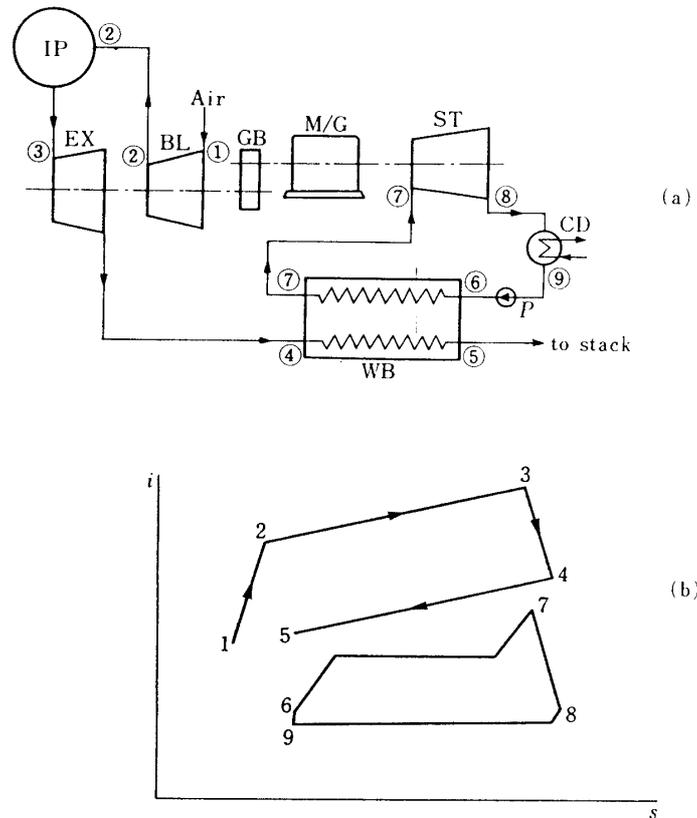
Fig. 7. Scheme of the conventional combined steam power recovery energy system.
