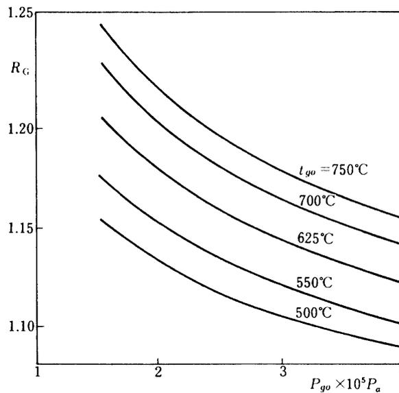
Fig. 8. Variation of relative power output increase  $R_G$  with  $P_{g0}$  and  $t_{g0}$  for TPRS.
