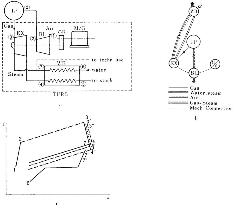
Fig. 3. Scheme of the total power recovery energy system (TPRS).
