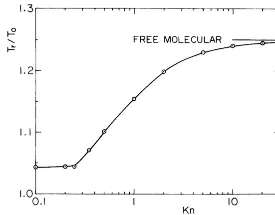
Fig. 13. Recovery temperature.
