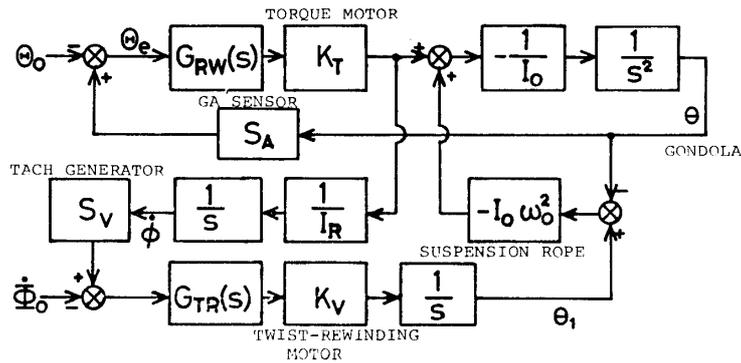
FIG. 3-1. Block diagram of the servo-control system based on the reaction wheel in conjunction with the twist-rewinding motor.
