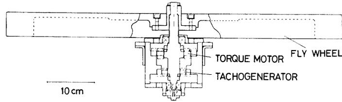
FIG. 2-1. Mechanical structure of the reaction wheel driving system. The wheel has a diameter of 68 cm, a mass of 22 kg and a moment of inertia of  $1.7 \text{ kg}\cdot\text{m}^2$ . The torque motor is a model T-2967 of Inland Co. and the tachogenerator is a model TG-2179B.
