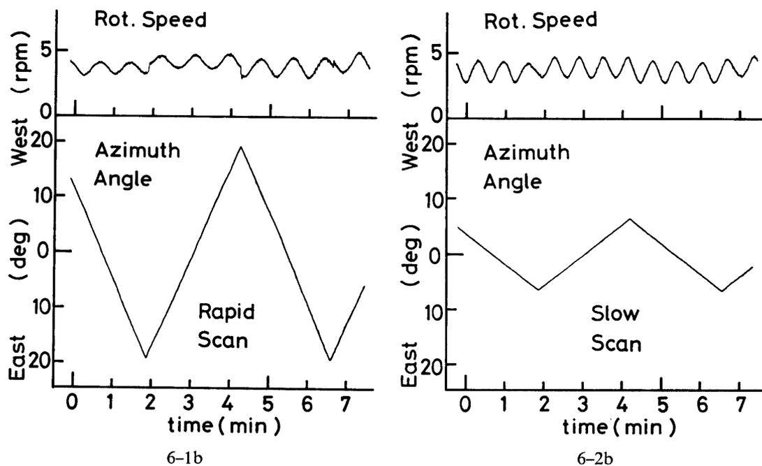
FIG. 6-1, 2b. Scanning profiles in the rapid and the show modes at the balloon experiments.
