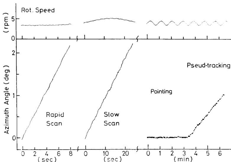
FIG. 6-1a. Profiles of the azimuthal angle of the gondola and the rotation speed of the wheel in the various maneuvering modes at the balloon experiments.
