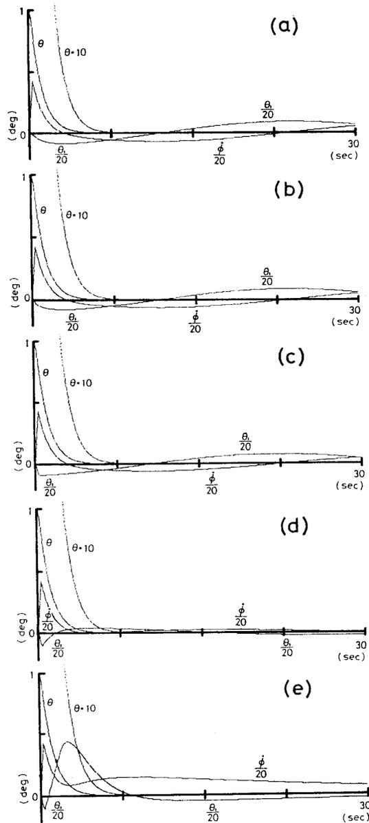
FIG. 4-3. Same as FIG. 4-1, but parameters of the servo-control is  $a=2500 \text{ sec}^{-1}$ ,  $b=2500 \text{ sec}^{-2}$  and  $B=0.18$ . A damping term related to the twist-rewinding motor,  $A$ , is taken as follows; (a) 0.005 sec, (b) 0.05 sec, (c) 0.18 sec, (d) 0.5 sec and (e) 5.0 sec.
