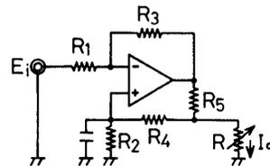
FIG. 5-1. Voltage-to-current converter based on an operational amplifier exploited in this experiment. A register  $R_4$  is introduced for the usage at large current. Resistors are taken as  $R_1=60$  k,  $R_2=30$  k,  $R_3=120$  k,  $R_4=60$  k and  $R_5=0.5 \Omega$ .
