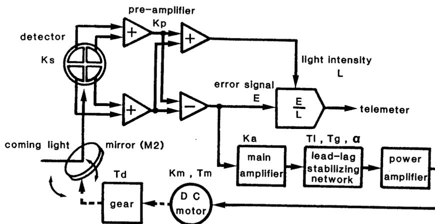
Fig. 7. Block diagram of the fine pointing system. Detector connection is only e.g. for yaw.
