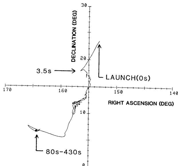
Fig. 10. Locus of nose direction determined by gyro.
