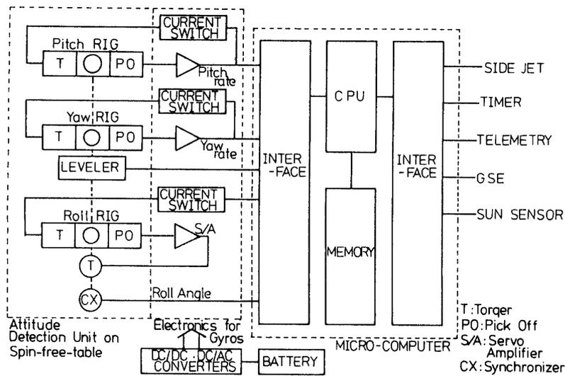
Fig. 3. Block diagram of attitude control system for S-520-5.
