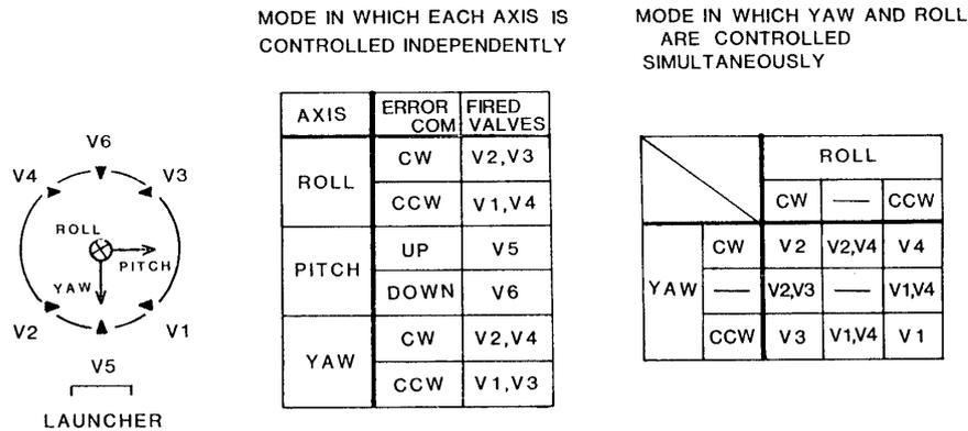
Fig. 1. Engine configuration and its firing logic.
