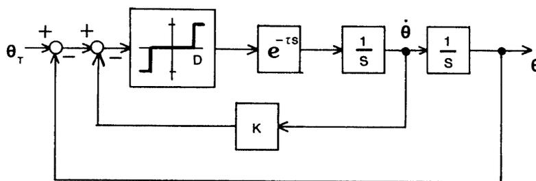
Fig. 5. Block diagram of attitude control system.
