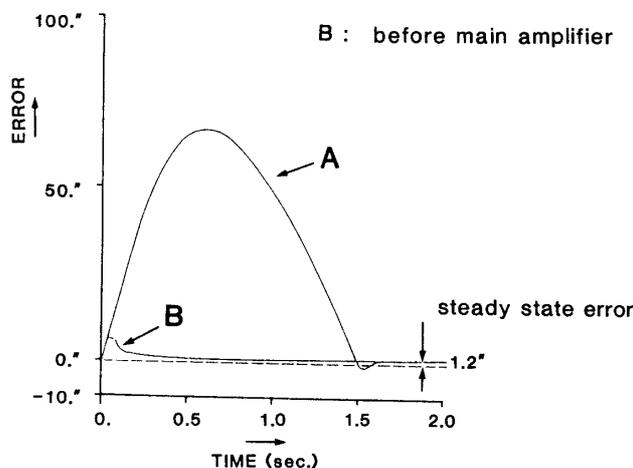
Fig. 8. Simulated transient response to a ramp-function input ( $0.1^\circ \text{ s}^{-1}$ ).
