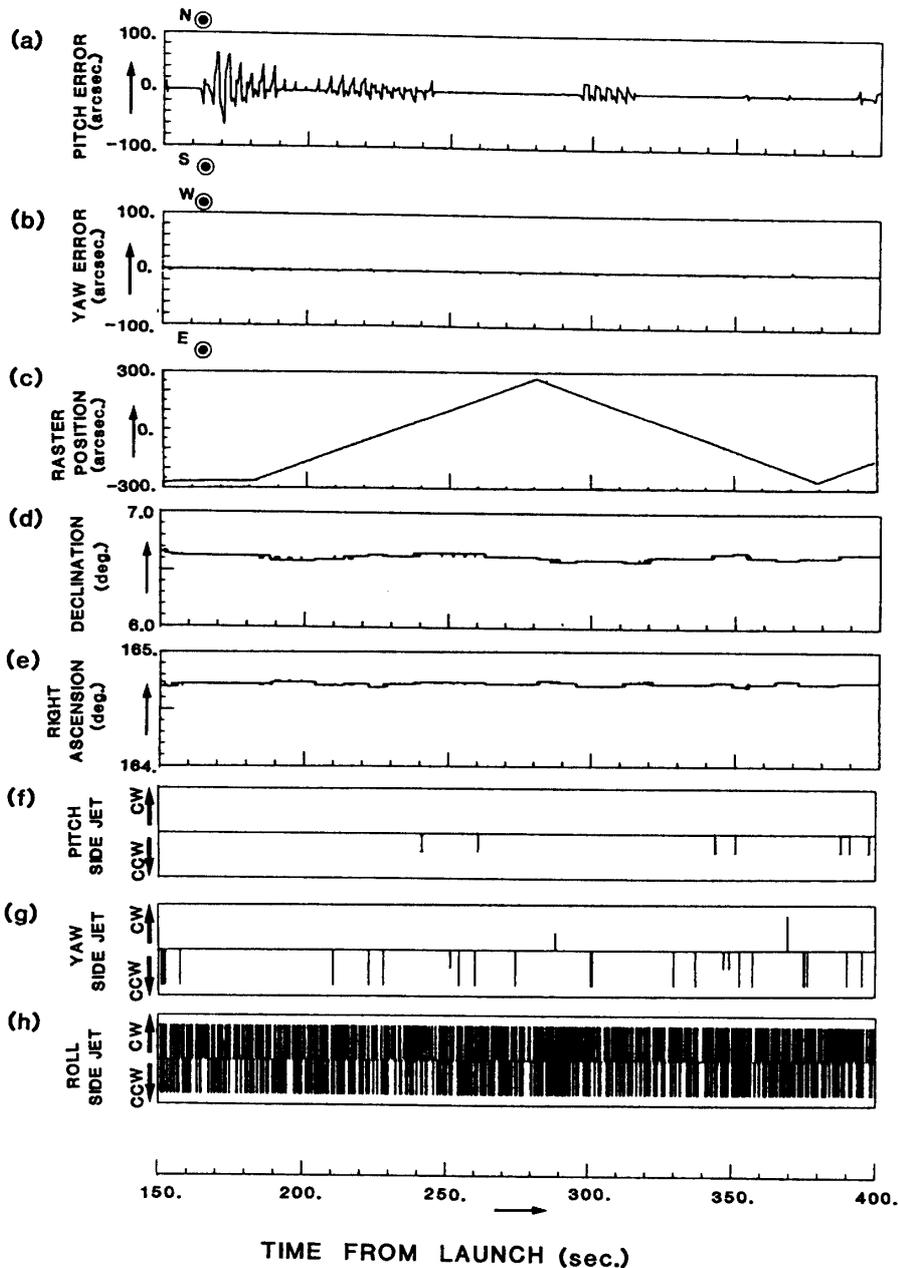
Fig. 12. The result of the fine pointing during the flight. In the bottom are shown timings of side jets. (see Fig. 1 for the definition of V's).
