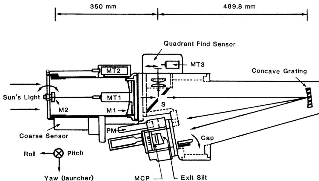
Fig. 6. Solar EUV telescope-spectrograph.
