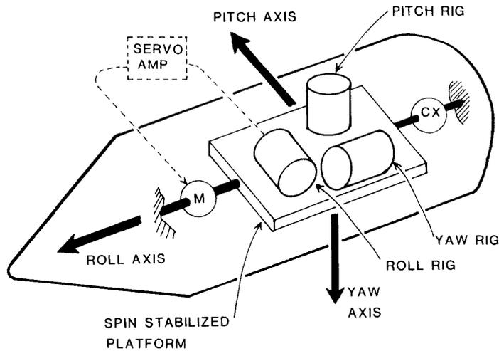
Fig. 2. Attitude measurement unit.
