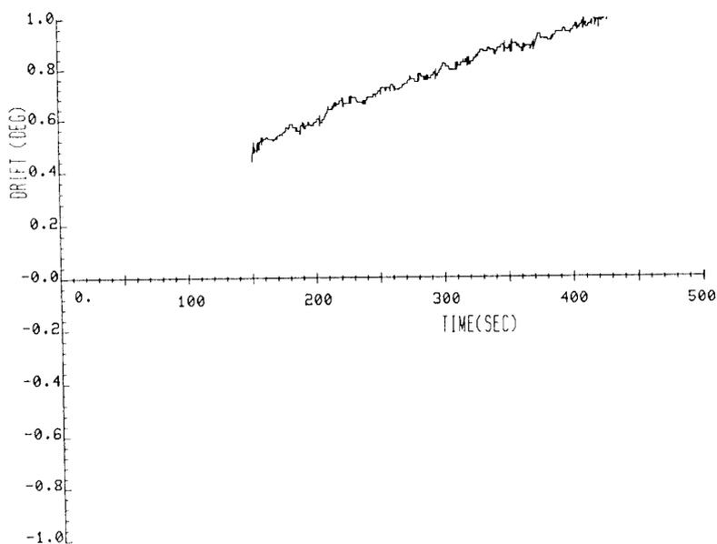
Fig. 11. Gyro drift in right ascension direction vs. time.
