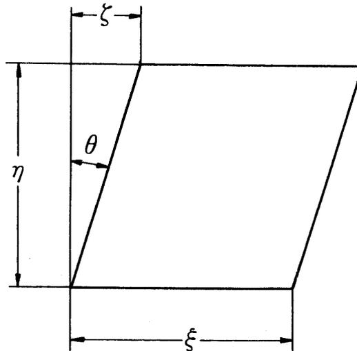
Fig. 7. Basic parallelogram element whose tessellation composes fold lines of two-dimensional folding by DDC surface.
