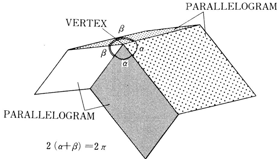
Fig. 5. Fundamental region of developable double corrugation (DDC) surface.
