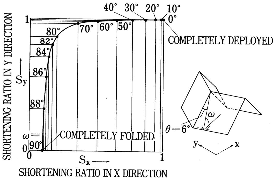
Fig. 8. Locus of folding and deployment of two-dimensional folding by DDC surface (relation between shortening ratios  $S_x$  and  $S_y$ ).
