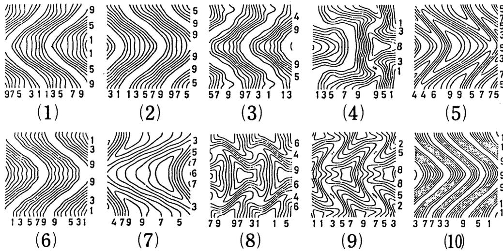
Fig. 3. Various solutions as to deformation of bi-axially shortened infinite plate (contour map).
