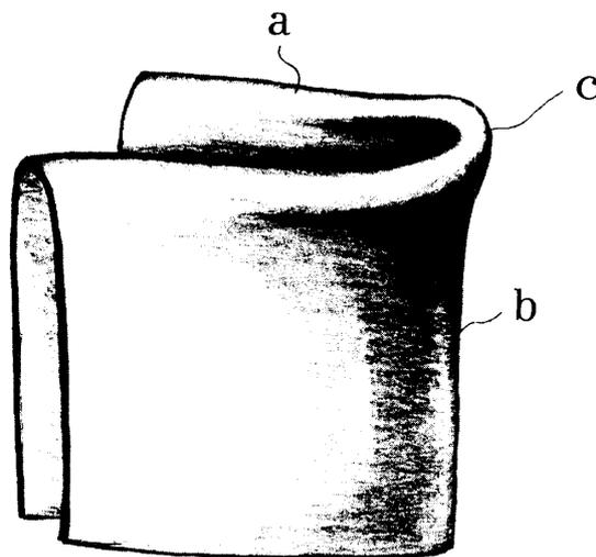
Fig. 2. Enlarged sketch showing deformation of a sheet at a node.
