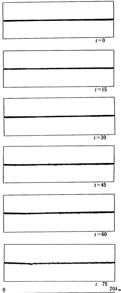
Fig. 14. Vorticity contours obtained by the present method with interval 0.04 from  $t=0$  to 75 (continued). (flow out boundary condition and random inflow disturbance are adopted)
