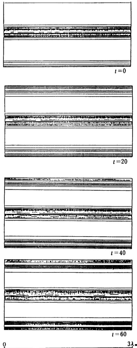
Fig. 13. Vorticity contours obtained by the present method with interval 0.04 from  $t=0$  to 60 (continued). (random initial disturbance and cyclic boundary condition are adopted)
