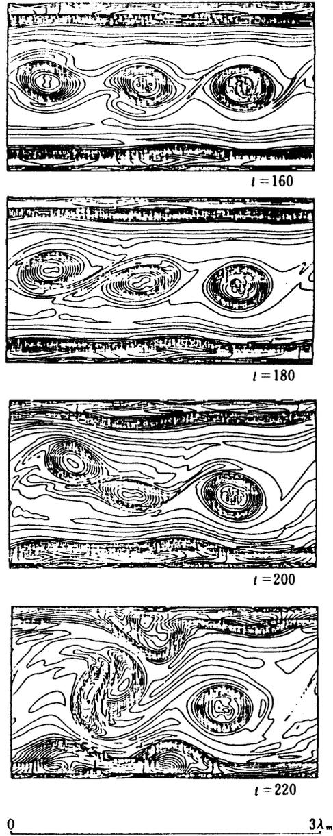
Fig. 13. Vorticity contours obtained by the present method with interval 0.04 from  $t=160$  to 220 (continued). (random initial disturbance and cyclic boundary condition are adopted)
