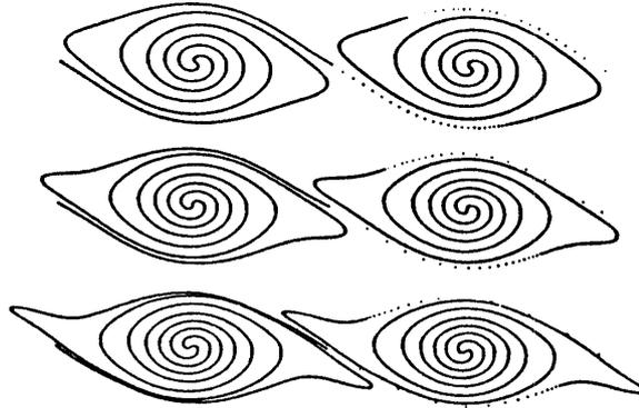
Fig. 10. asymptotic behavior of the rolled up vortex sheet by vortex method (from Ref. [16]).
