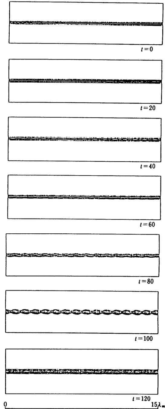
Fig. 3. Temporal evolution of the vorticity contours with step 0.04 obtained by Kawamura's method from  $t=0$  to 120 (continued). (monochronic initial disturbance and cyclic boundary condition are adopted)
