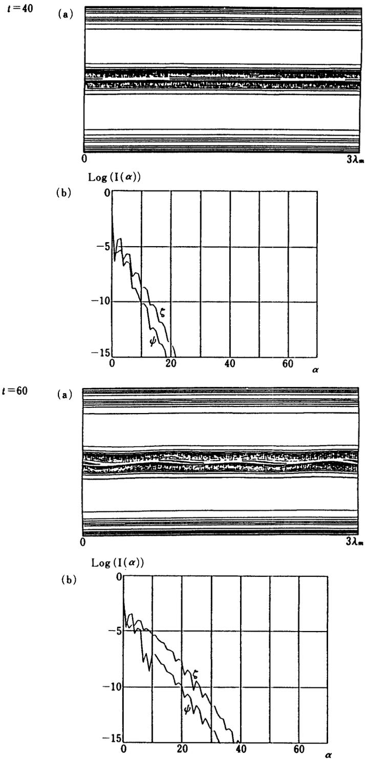
Fig. 11. (a) Vorticity contours of merging vortices obtained by the present method with interval 0.04.
