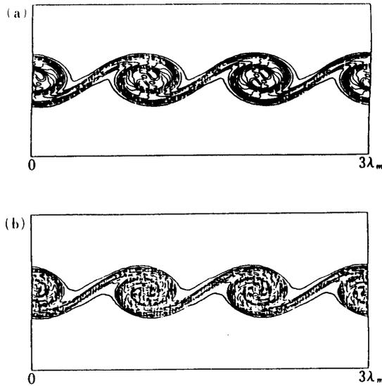
Fig. 17. Vorticity contours with step 0.04.
