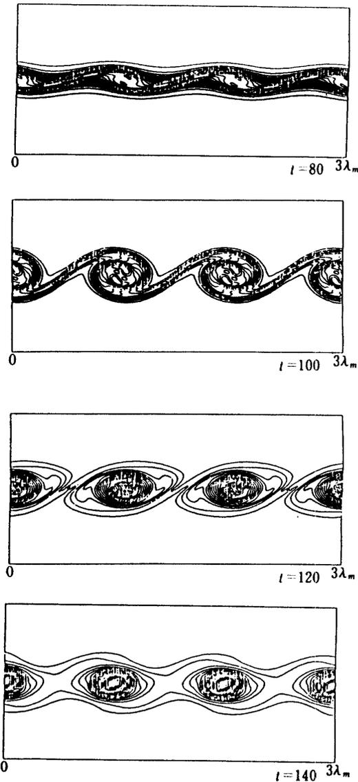
Fig. 16. Temporal evolution of the vorticity contours obtained by Kawamura's method with step 0.04 from  $t=80$  to 140 (continued). (monochronic initial disturbance and cyclic boundary condition are adopted)
