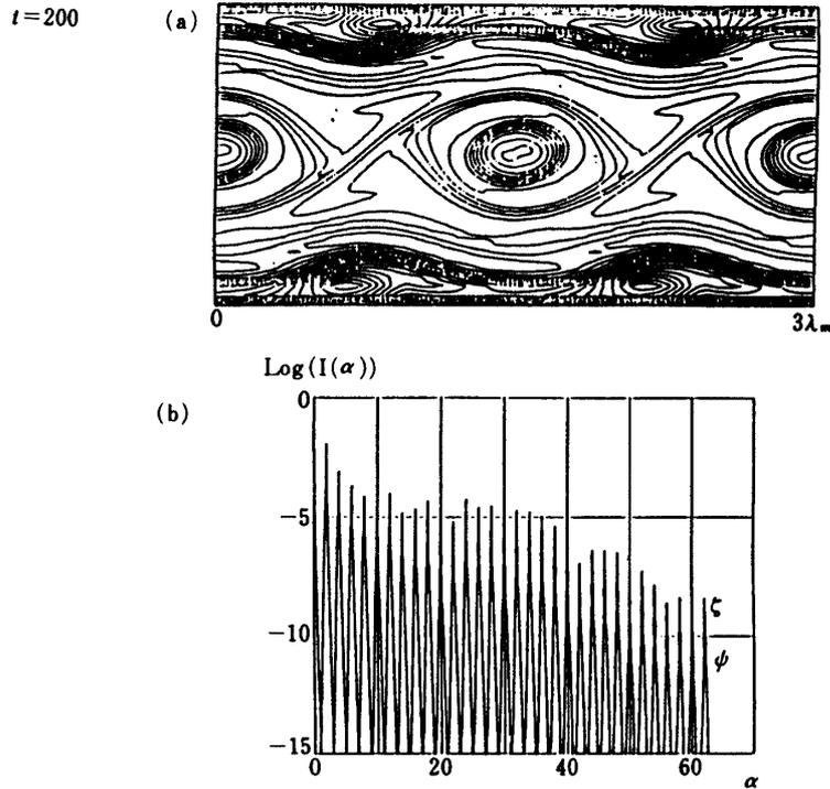
Fig. 12. (a) Vorticity contours of stretching vortices obtained by the present method with interval 0.04. (b) its Fourier analysis in x-direction.  $t=200$ . (cyclic boundary condition is adopted)
