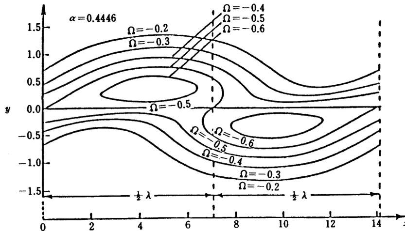
Fig. 9. Vorticity contours obtained by small disturbance theory (from Ref. [15]).
