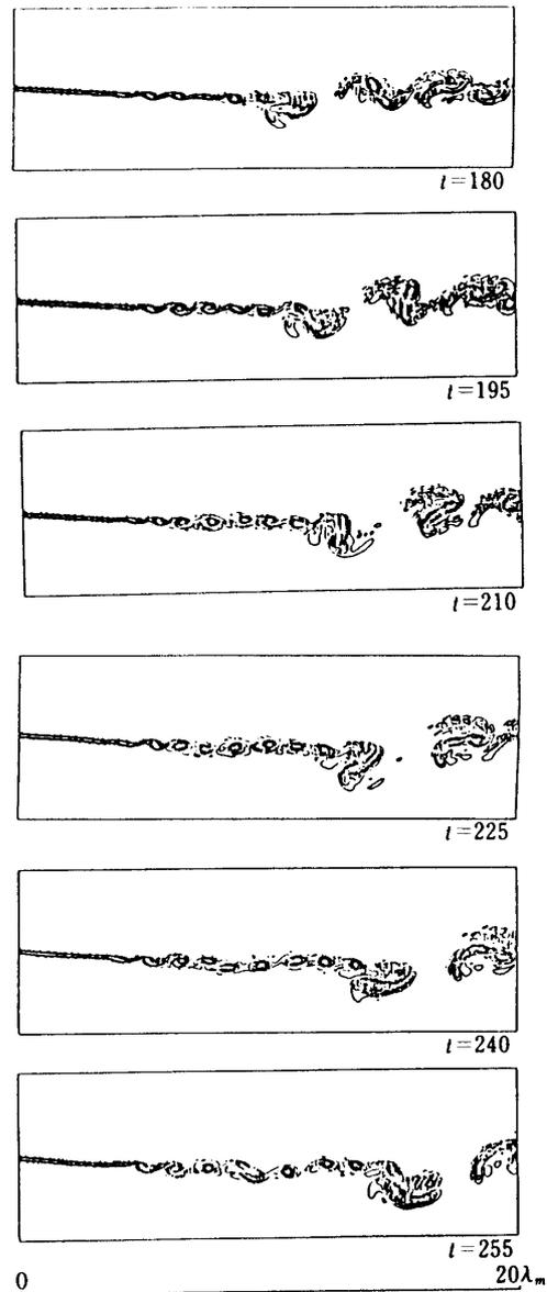
Fig. 14. Vorticity contours obtained by the present method with interval 0.04 from  $t=180$  to 255 (continued).
