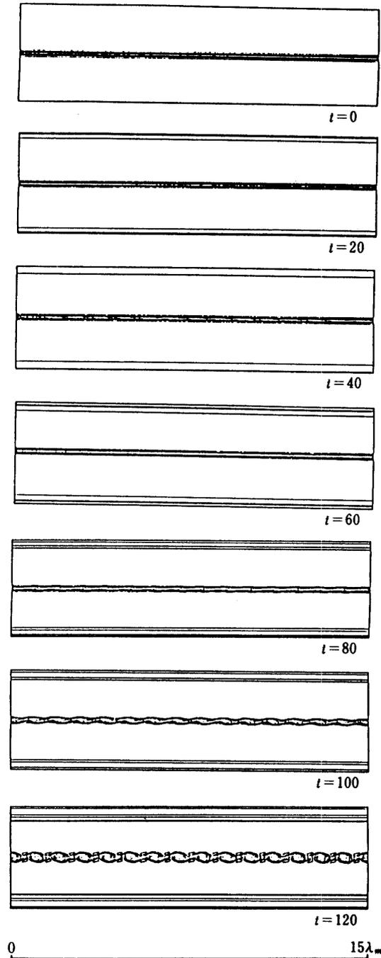
Fig. 2. Temporal evolution of the vorticity contours on the coarse grid system with step 0.04 obtained by the present method from  $t=0$  to 120 (continued). (monochronic initial disturbance and cyclic boundary condition are adopted)
