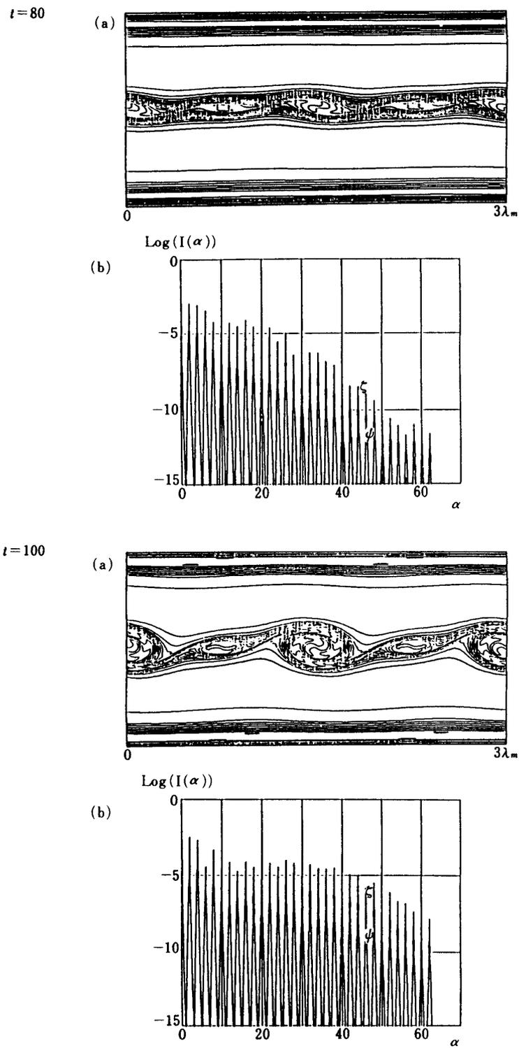
Fig. 12. (a) Vorticity contours of stretching vortices obtained by the present method with interval 0.04. (b) its fourier analysis in x-direction.  $t=80$  to 100 (continued). (cyclic boundary condition is adopted)
