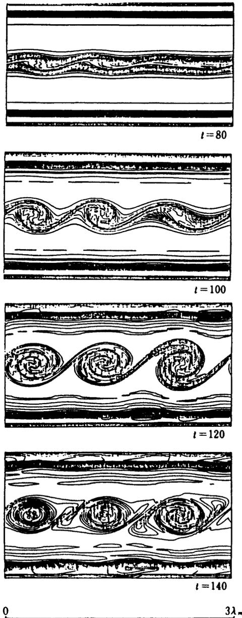
Fig. 13. Vorticity contours obtained by the present method with interval 0.04 from  $t=80$  to 140 (continued). (random initial disturbance and cyclic boundary condition are adopted)
