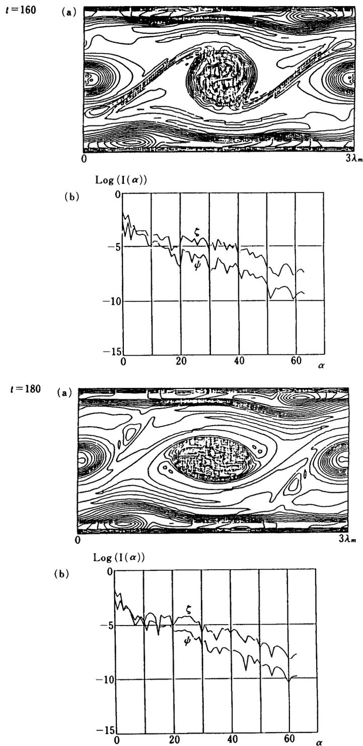
Fig. 11. (a) Vorticity contours of merging vortices obtained by the present method with interval 0.04.
