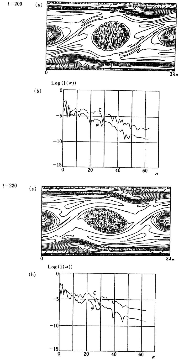
Fig. 11. (a) Vorticity contours of merging vortices obtained by the present method with interval 0.04. (b) its Fourier analysis in x-direction.  $t=200$  to 220. (cyclic boundary condition is adopted)
