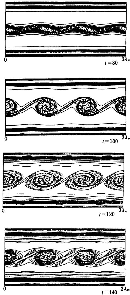
Fig. 8. Temporal evolution of the vorticity contours obtained by the present method with step 0.04 from  $t=80$  to 140 (continued). (monochronic initial disturbance and cyclic boundary condition are adopted)
