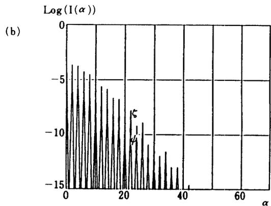
Fig. 12. (a) Vorticity contours of stretching vortices obtained by the present method with interval 0.04. (b) its fourier analysis in x-direction.  $t=40$  to 60 (continued). (cyclic boundary condition is adopted)
