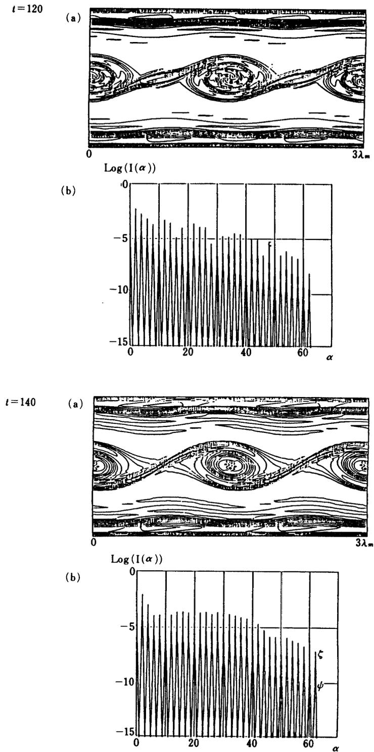
Fig. 12. (a) Vorticity contours of stretching vortices obtained by the present method with interval 0.04. (b) its fourier analysis in x-direction.  $t=120$  to 140 (continued). (cyclic boundary condition is adopted)
