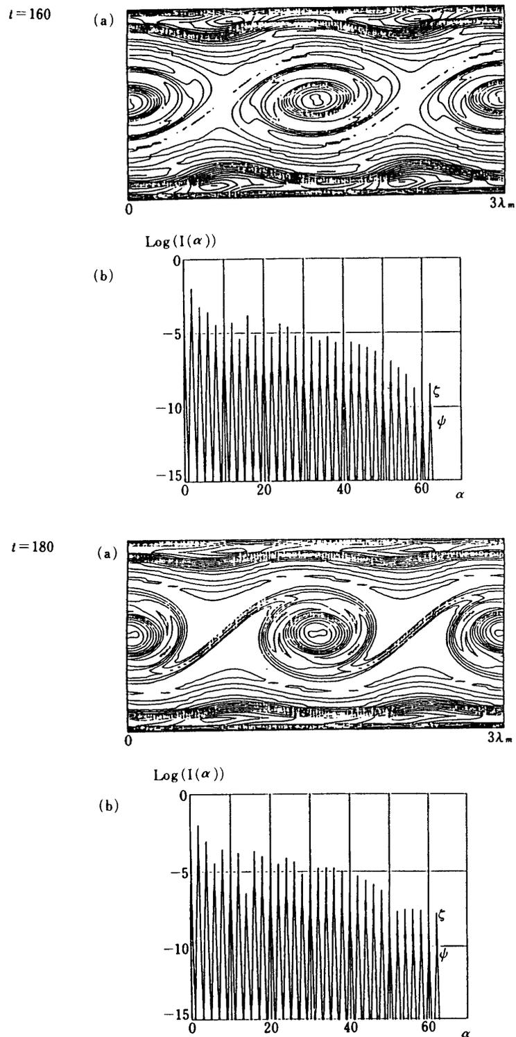
Fig. 12. (a) Vorticity contours of stretching vortices obtained by the present method with interval 0.04. (b) its Fourier analysis in  $x$ -direction.  $t = 160$  to 180 (continued). (cyclic boundary condition is adopted)
