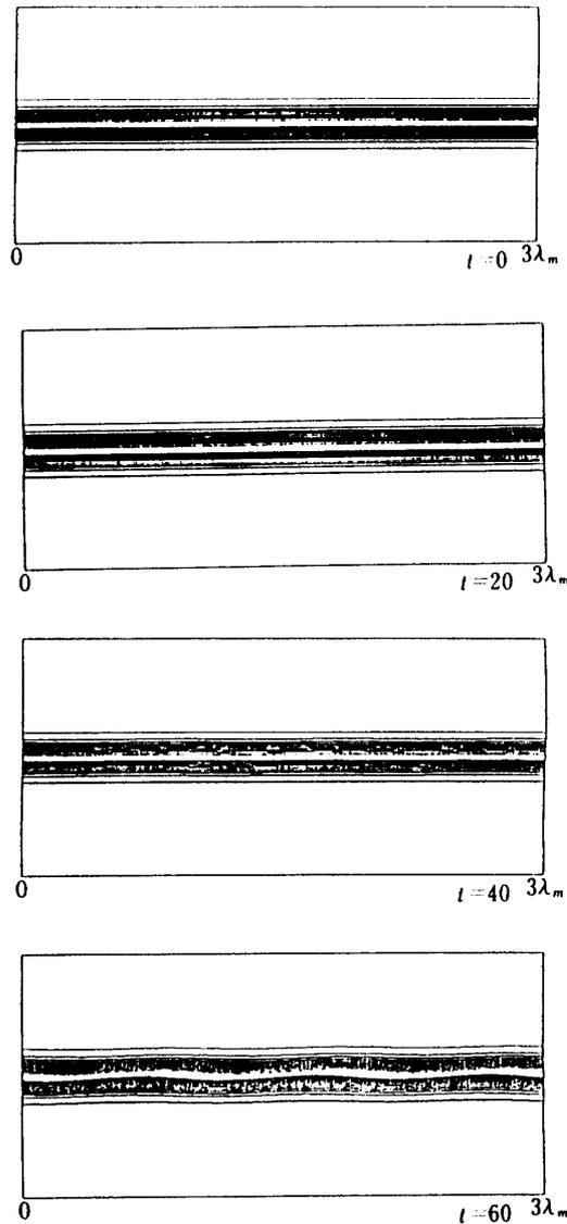
Fig. 16. Temporal evolution of the vorticity contours obtained by Kawamura's method with step 0.04 from  $t=0$  to 60 (continued). (monochronic initial disturbance and cyclic boundary condition are adopted)
