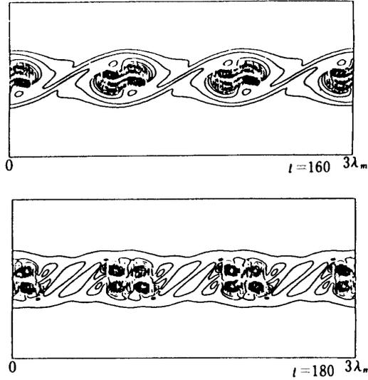
Fig. 16. Temporal evolution of the vorticity contours obtained by Kawamura's method with step 0.04 from  $t=160$  to 180 (continued). (monochronic initial disturbance and cyclic boundary condition are adopted)
