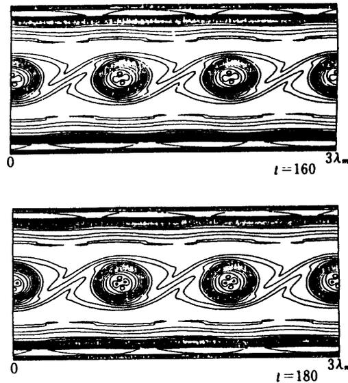
Fig. 8. Temporal evolution of the vorticity contours obtained by the present method with step 0.04 from  $t=160$  to  $180$ . (monochronic initial disturbance and cyclic boundary condition are adopted)
