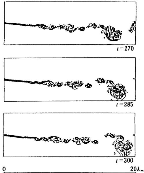
Fig. 14. Vorticity contours obtained by the present method with interval 0.04 from  $t=270$  to 300 . (flow out boundary condition and random inflow disturbance are adopted)
