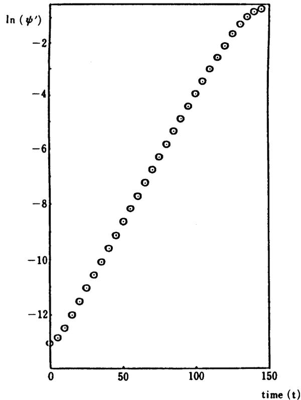
Fig. 7. Typical temporal evolution of the amplitude of the disturbance to the stream function in the linear regime ( $\alpha=0.4446$ ).
