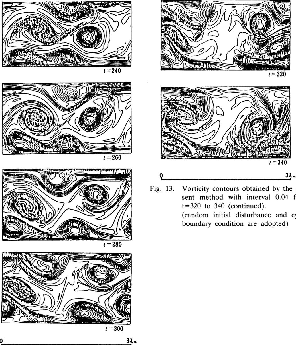
Fig. 13. Vorticity contours obtained by the present method with interval 0.04 from  $t=320$  to 340 (continued). (random initial disturbance and cyclic boundary condition are adopted)
