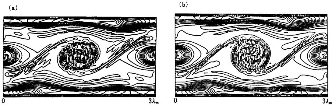
Fig. 1. Vorticity contours of merging vortices in the case of same intensity merging at  $t=140$ .
