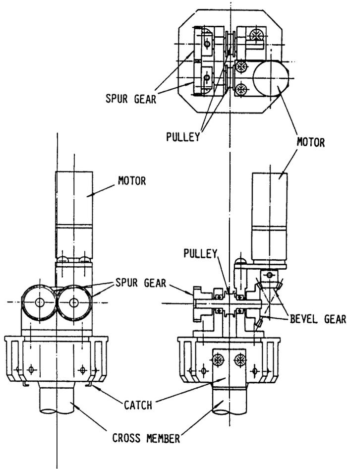
Fig. 11. The Fixed-Hinge-Assembly for Nodes 1 and 3 of Fig. 1.
