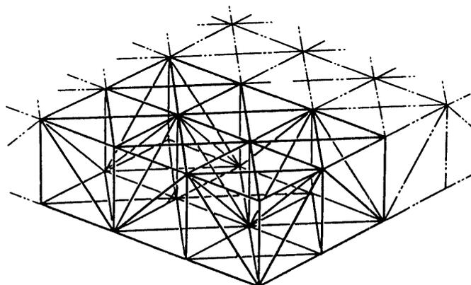
Fig. 3. A SHDF Truss Platform Composed of a Plurality of Modules.
