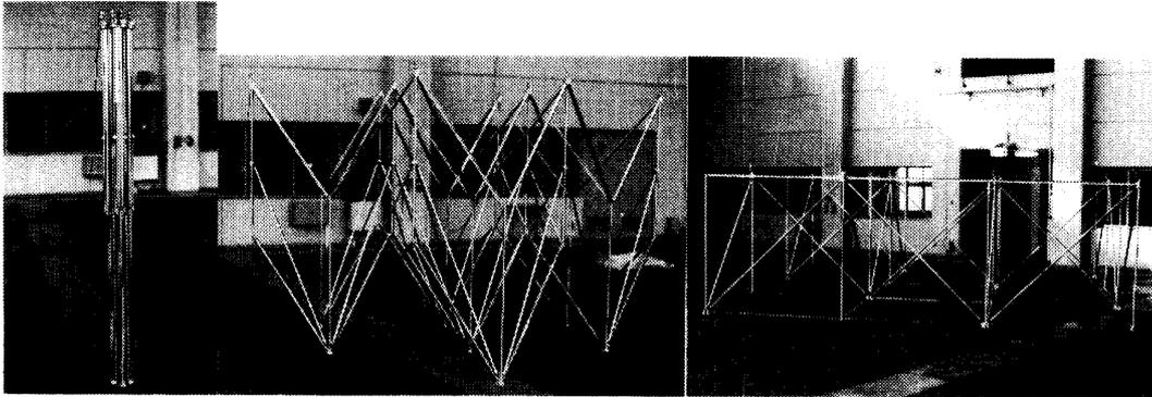
Fig. 16. Deployment/Folding Test of a SHDF Platform.
