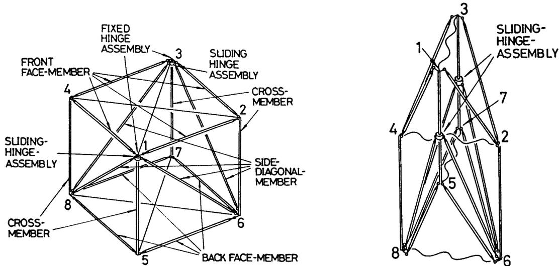
Fig. 1. A Fully Deployed Module of SHDF Truss.
