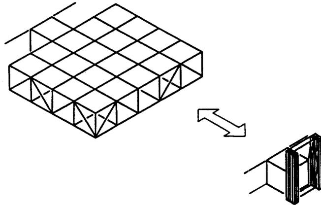
Fig. 9. A Combination of SHDF and SHSF Trusses.
