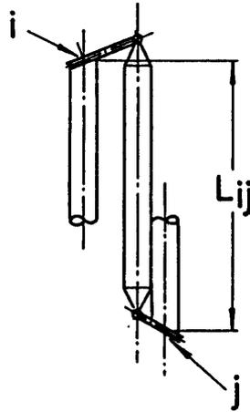
Fig. 5. Effective Length of the Member Connecting Node  $i$  to Node  $j$ .
