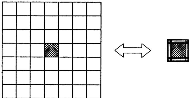
Fig. 18. A Plan View of Deployment/Folding of Space Antenna Composed of SHDF and SHSF Trusses.
