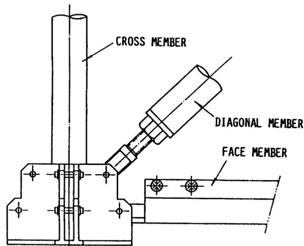
Fig. 15. The Fixed-Hinge-Assembly for Nodes 6 and 8 of Fig. 1.
