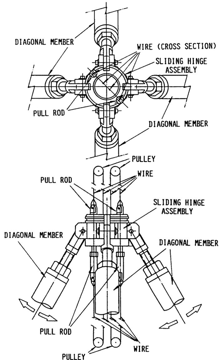
Fig. 13. A Sliding-Hinge-Assembly.
