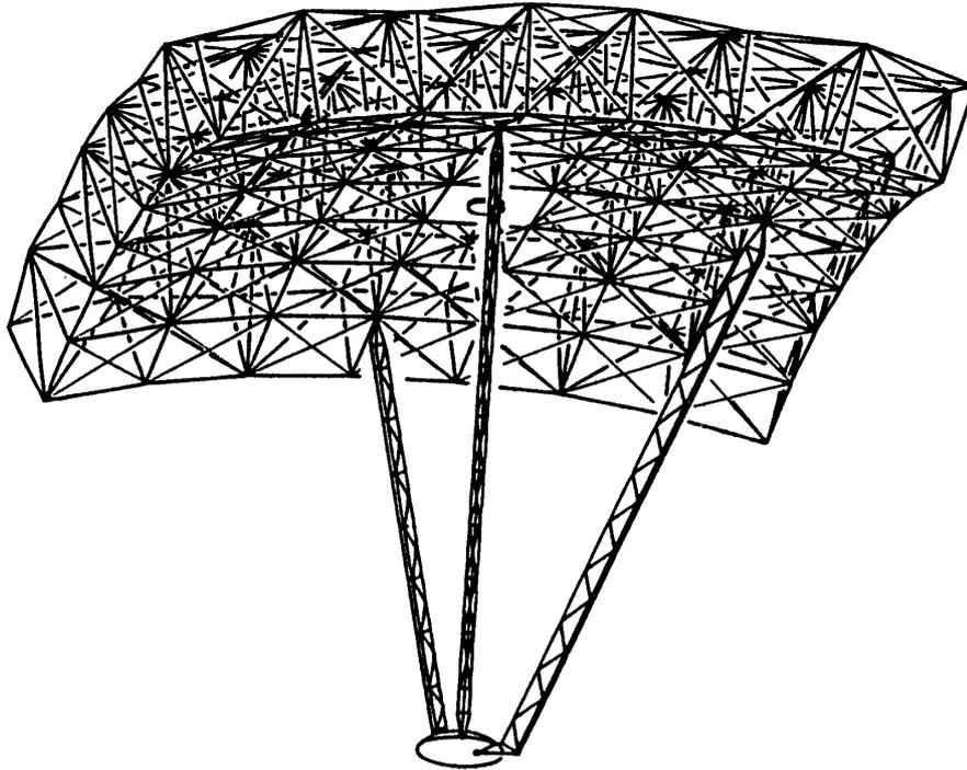
Fig. 17. A Huge Space Antenna Composed of SHDF and SHSF Trusses.
