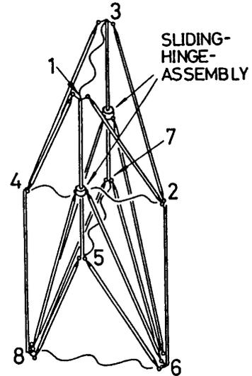
Fig. 2. A Half Folded/Deployed Module of SHDF Truss.
