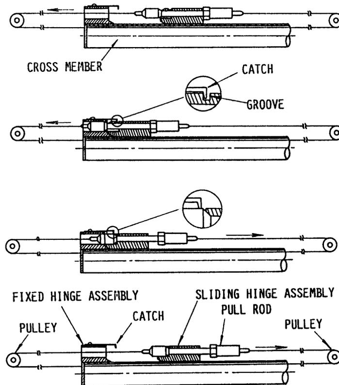
Fig. 14. The Lock/Release Mechanism.
