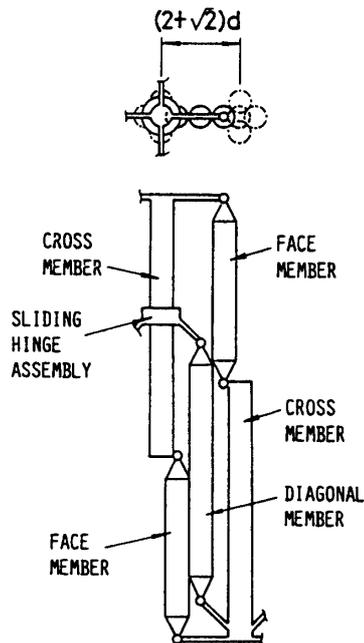
Fig. 4. Most Compactly Folded Side Face of a SHDF Truss Module.
