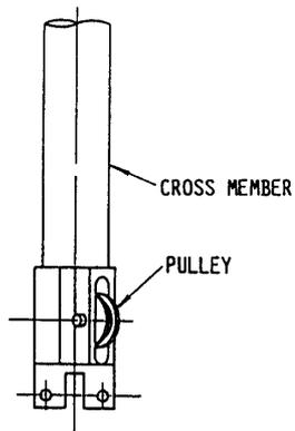
Fig. 12. The Fixed-Hinge-Assembly for Nodes 5 and 7 of Fig. 1.
