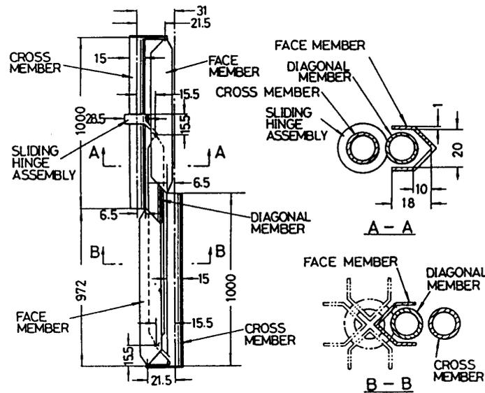
Fig. 10. Nesting Scheme and Dimensions of the Model Components. (unit=mm)
