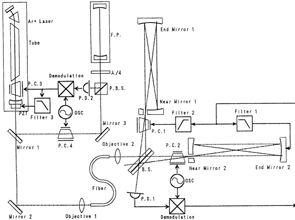
Fig. 1. Schematic diagram of the 10 m prototype of a laser interferometric gravitational wave antenna. The frequency stabilizing argon-ion laser, the optical fiber, the two arms of the interferometer with 4 beam delay-line, and fringe lock-in system are shown.
