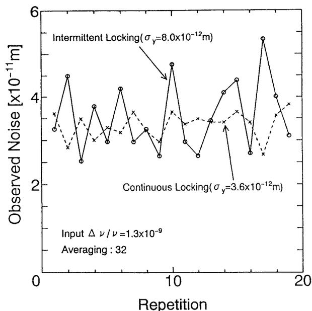
Fig. 7. Comparison between changes of observed noises due to additional frequency fluctuation in two conditions of locking the interference fringe by the main feedback system. Change of the observed noise in intermittent locking is larger than that in continuous locking.
