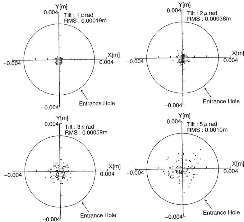
Fig. 3. The position of the outgoing beam from the delay-line consist of two mirrors with the local tilt. The cases of mirrors with the tilt of 1~5  $\mu$ rad are shown. In the case of the mirrors with the tilt of 1  $\mu$ rad, the beam position has a deviation of 0.2 mm<sub>rms</sub> from the center of entrance hole.
