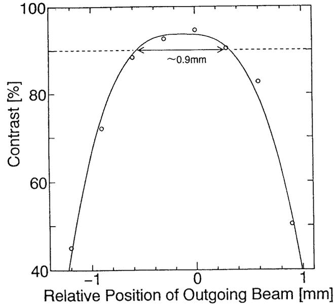
Fig. 2. An example of the contrast dependence of interference fringe upon the outgoing beam position on the near mirror with the same entrance position of beam. If we need a contrast better than 90%, the allowed region of the position change is about 0.9 mm.
