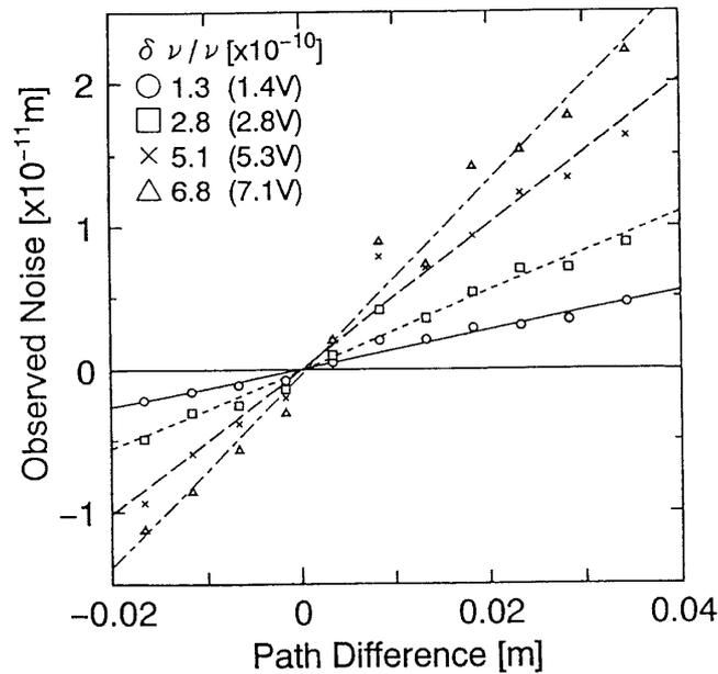
Fig. 4. Relations between noise due to artificial laser frequency fluctuation and relative statical path difference. Four kinds of data show measured values for additional signals of 1.4, 2.8, 5.3, and 7.1  $V_{rms}$  to P.C. 3 (Fig. 1), respectively. Each data is fitted to linear function by method of least squares. All of lines cross approximately at the same point where the path difference is zero.  $\delta\nu/\nu$ s evaluated from the slopes of fitting lines are written.
