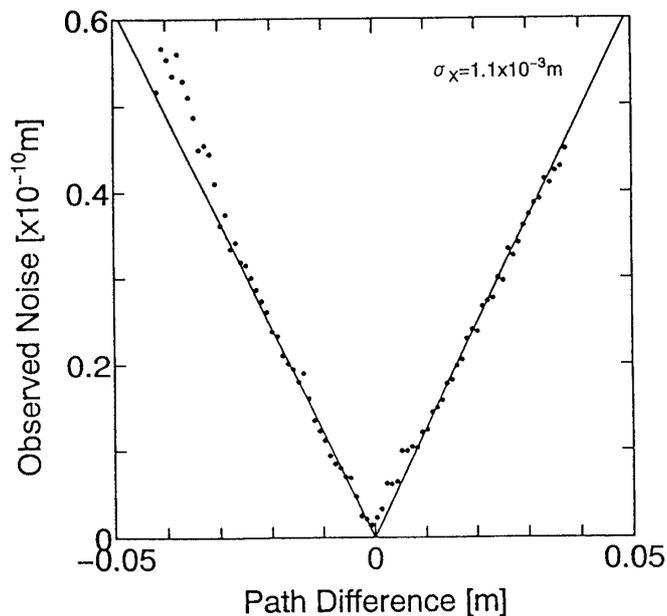
Fig. 5. The relation between noise due to the frequency fluctuation and statical path difference. In order to investigate measurement error of statical path difference, data were taken in detail to arm length change. By using method of least squares, standard deviation of measured point in direction of X-axis is decided to  $1.1 \times 10^{-3} m$ . The data less than  $-0.03 m$  or near  $0 m$  in path difference are not used for this calculation.
