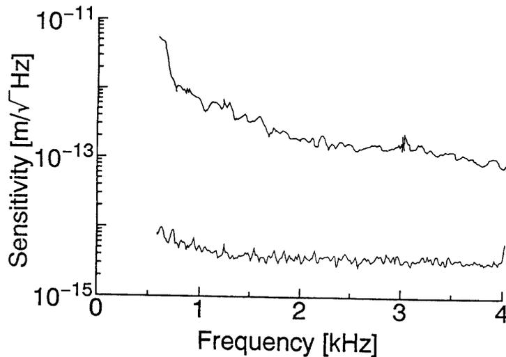
Fig. 6. Sensitivities of our interferometer without frequency stabilizing system. In the case of using old mirrors, since the residual difference of arm length is approximately 10 mm at the same number of reflection, noise due to frequency fluctuation is large (upper curve). On the other hand, the sensitivity a little larger than expected noise  $\delta L_{FR} = 2.9 \times 10^{-15}\text{m}/\sqrt{\text{Hz}}$  was acquired with new mirrors (lower curve).
