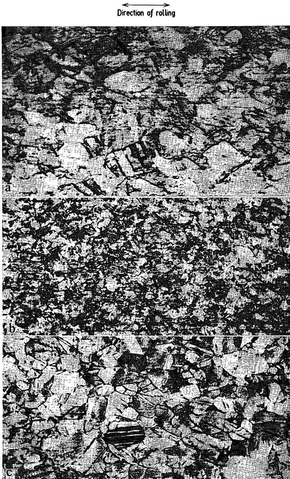
Fig. 3. Micrographs of nickel silver strip. (a) No. 1 sample. As tension-annealed. \times 750 . (b) No. 1 sample. As tension-annealed. \times 180 . (c) No. 2 sample. As received. \times 180 .
