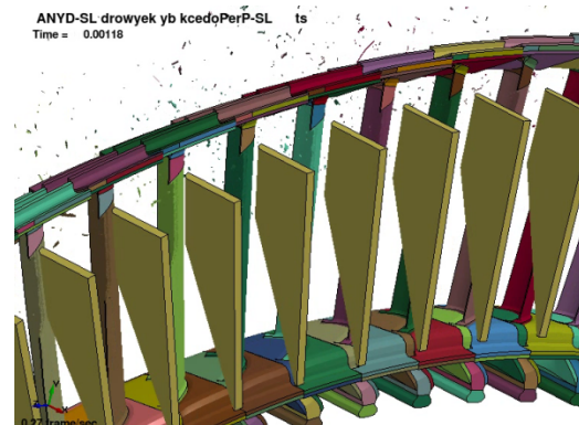
An analysis result of the cascades of CMC low pressure turbine blades.
