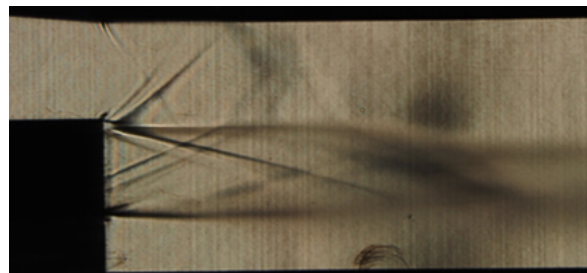
Schlieren photo — Rocket total pressure 20MPa
