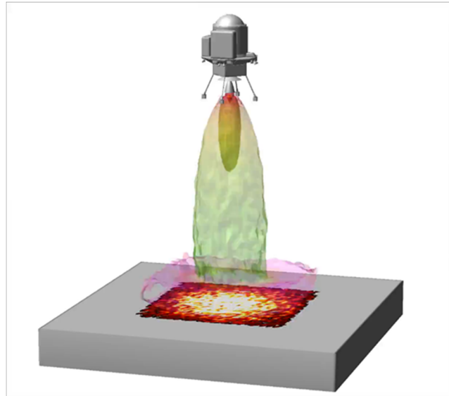
Main thruster plume distribution at landing on the moon
