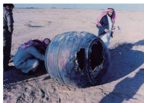
Titanium casting of STAR-48B SRM (Saudi Arabia, 2001)
