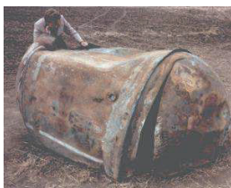
Delta II propellant tank (Georgetown, TX, 1997)
