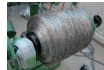
Tether spool (2 km Al-SUS tether)
