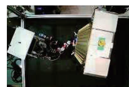
Robotic capture demonstration on an air-bearing table
