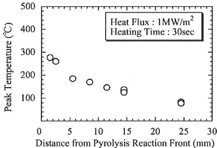
Fig. 14: Measured Spatial Distribution of the Peak Temperature in the T/P.
