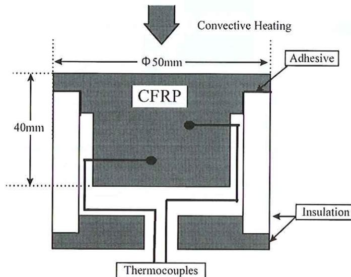
Fig. 4: Schematic of the MC-CFRP T/P Configuration at Arc Heating Experiments.
