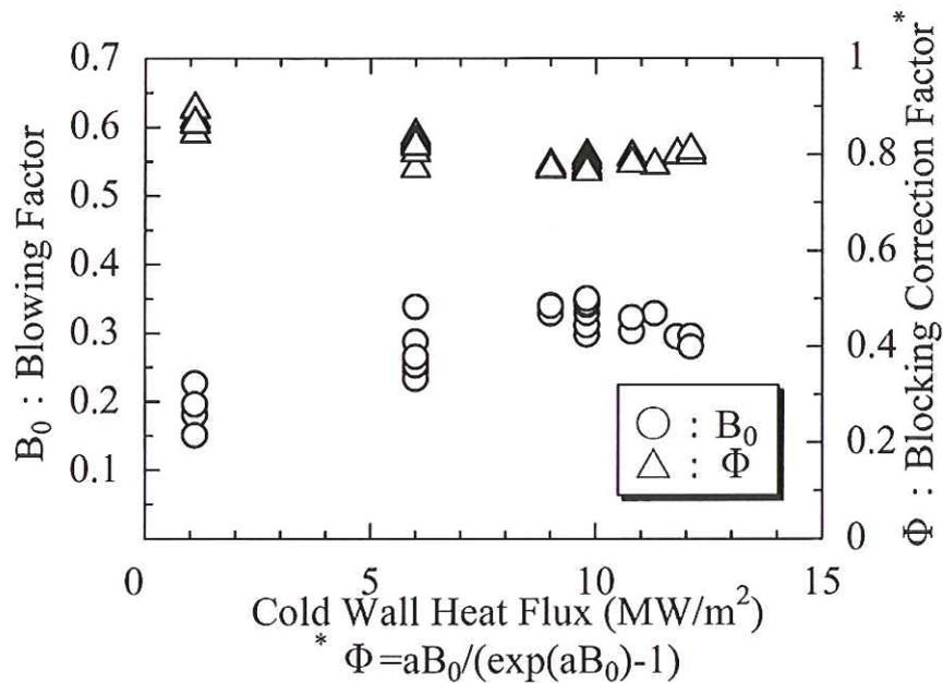
Fig. 13: Estimated Blocking Parameters from Measured Total Mass Loss.
