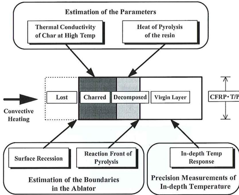
Fig. 2: Schematic of the Carbon Phenolic (MC-CFRP) T/P after the Arc Heating Experiments.
