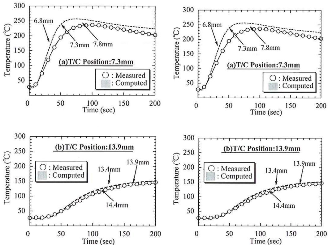
Fig. 15: Comparison of Measured and Computed In-depth Temperature Response (Heat Flux:1 MW/m<sup>2</sup>, Duration:30s).
