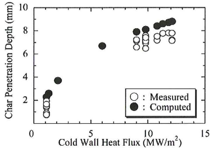
Fig. 12: Comparison of Measured and Computed Char Penetration Depth.
