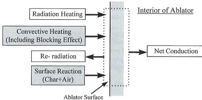
Fig. 5: Schematic of Surface Energy Balance and Semi-infinite Slab of Ablator Material.
