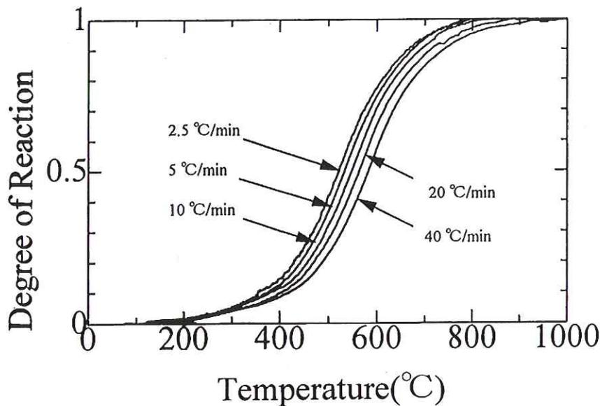
Fig. 8: Examples of Thermogravimetry Curves of MC-CFRP.
