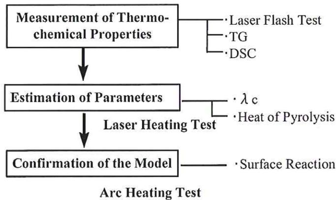
Fig. 3: Procedure of Construction of the Mathematical Model for the MC-CFRP Ablation.
