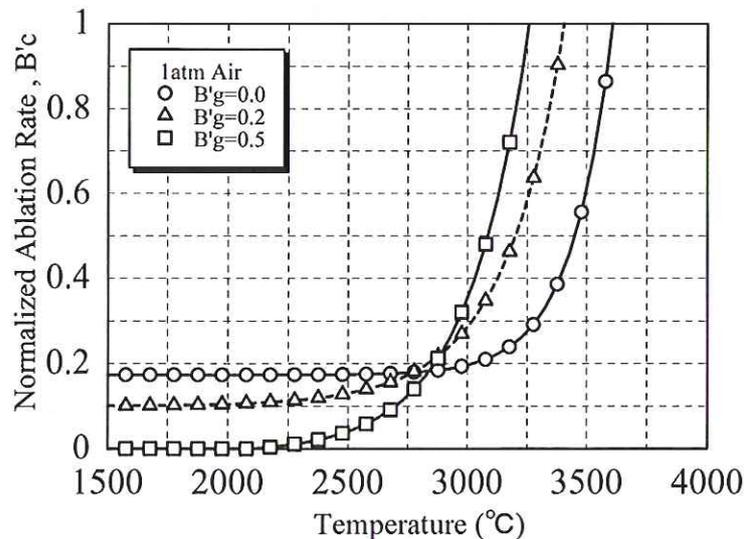
Fig. 7: A Typical Analytical Result of Nondimensional Recession Rate (@1 atm).
