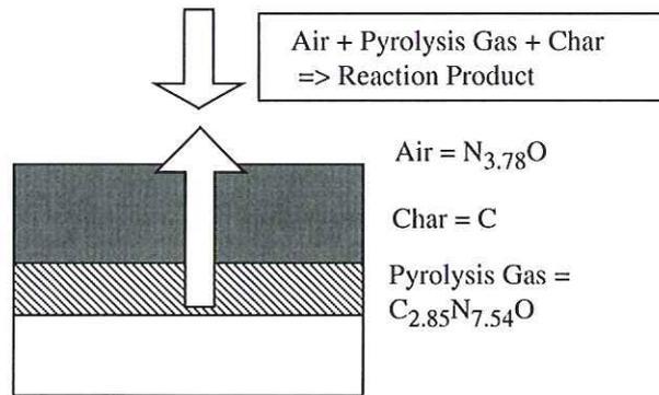
Fig. 6: Concept of the Reaction Model on the Charred Surface.
