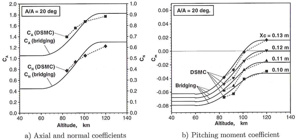
Fig. 1: Overall aerodynamic coefficient of MUSES-C capsule : obtained by empirical bridging formula ; angles of attack = 20 deg.
