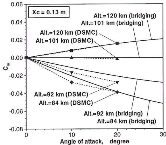
Fig. 2: Pitching moment coefficient as a function of angle of attack.
