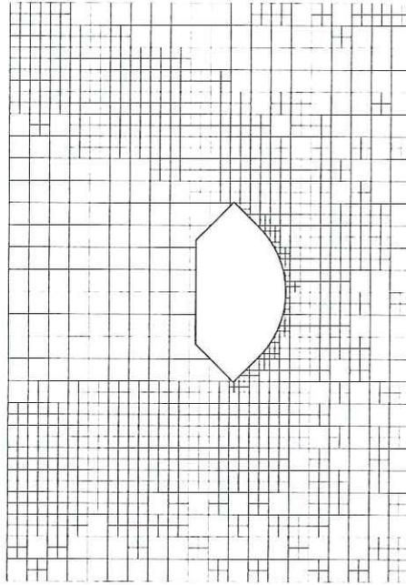
Fig. 3: Solution-adaptive grid based on cell Knudsen number : on symmetric plane, altitude = 92 km.
