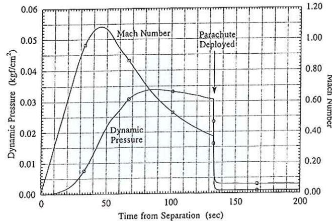
Fig. 18: Mach number and dynamic pressure during descent in free-flight test.
