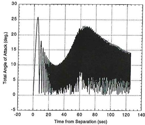
Fig. 20: Predicted total angle of attack history based on the wind-tunnel test.
