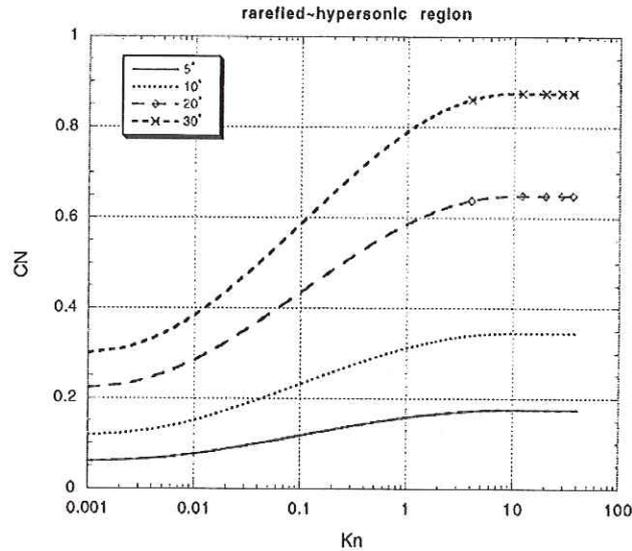
Fig. 5: Normal force coefficient vs. Knudsen number.
