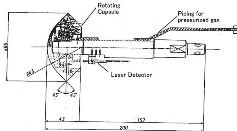
Fig. 21: Test device for damping-in-roll characteristics in wind tunnel.
