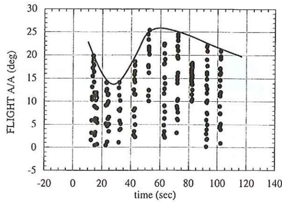
Fig. 19: Total angle of attack derived from CCD image in free-flight test.
