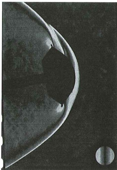
Fig. 11: Flow visualization with magnitude-indicating color mask (vertical layout) at  $M = 3.0$  and  $\alpha = 10deg.$
