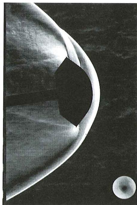
Fig. 12: Flow visualization with direction-indicating color mask at  $M = 3.0$  and  $\alpha = 10deg.$
