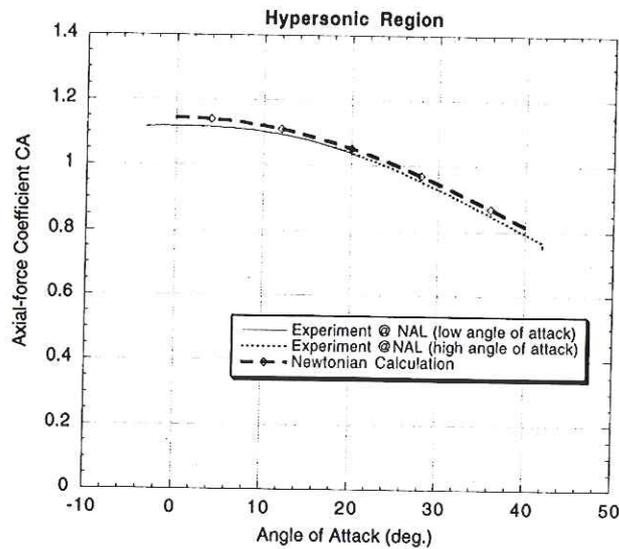
Fig. 8: Comparison of axial-force coefficient between experiments and newtonian calculation.
