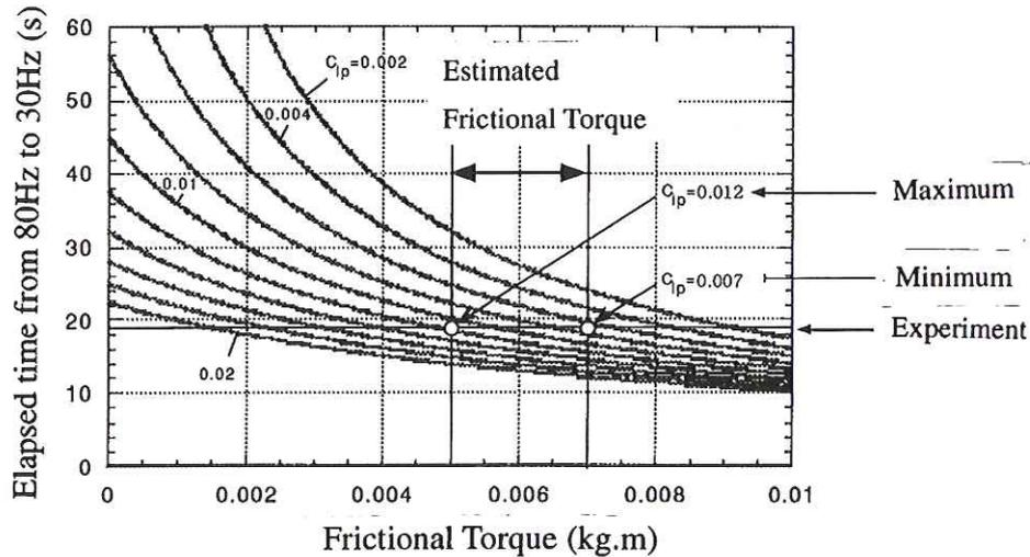
Fig. 22: Chart for estimation of damping-in-roll coefficient from experimental decay data of spin.
