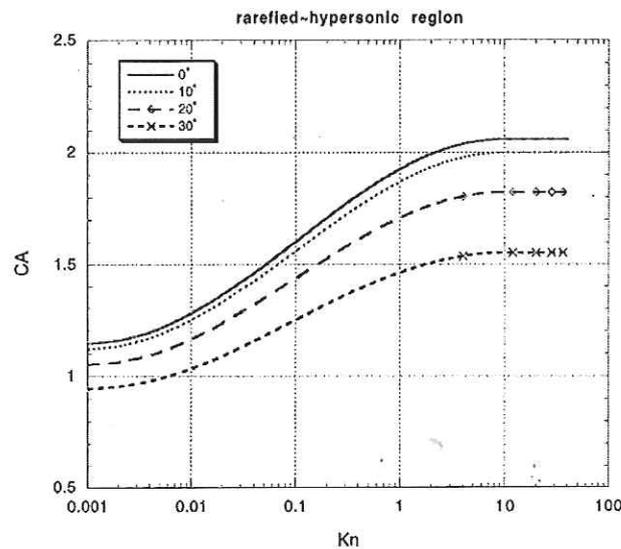
Fig. 4: Axial coefficient vs. Knudsen number.
