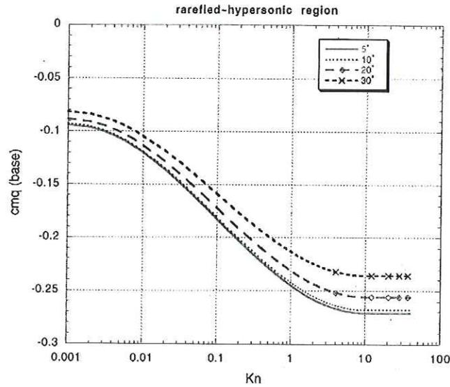
Fig. 7: Damping-in-pitch coefficient vs. Knudsen number.
