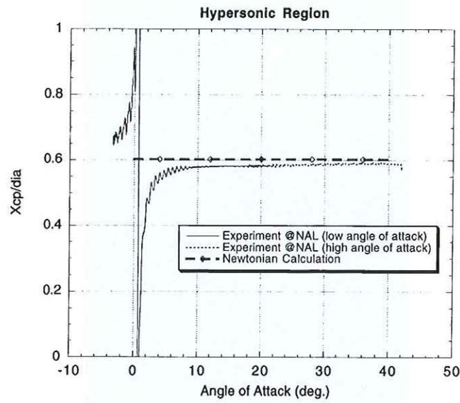
Fig. 9: Comparison of center-of-pressure location between experiments and newtonian calculation.
