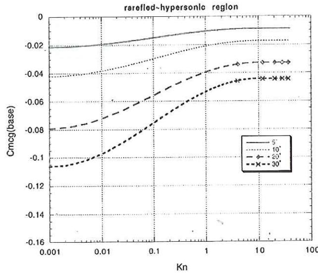
Fig. 6: Pitching Moment coefficient vs. Knudsen number ( $X_{cg}=0.122m$  from nose).
