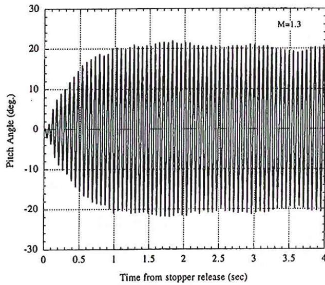
Fig. 14: Typical self-excited oscillation at  $M = 1.3$ .
