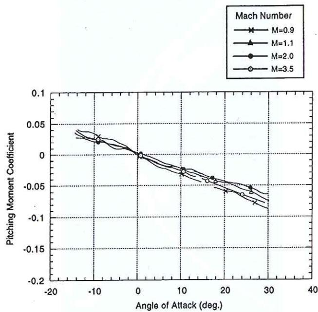
Fig. 10: Pitching moment slope ( $X_{cg}=0.122m$  from nose).
