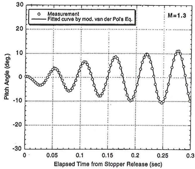
Fig. 15: Comparison of the curve-fit and the experimental oscillation at  $M = 1.3$
