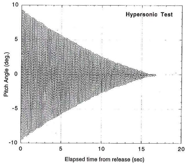
Fig. 17: Damping-in-pitch.
