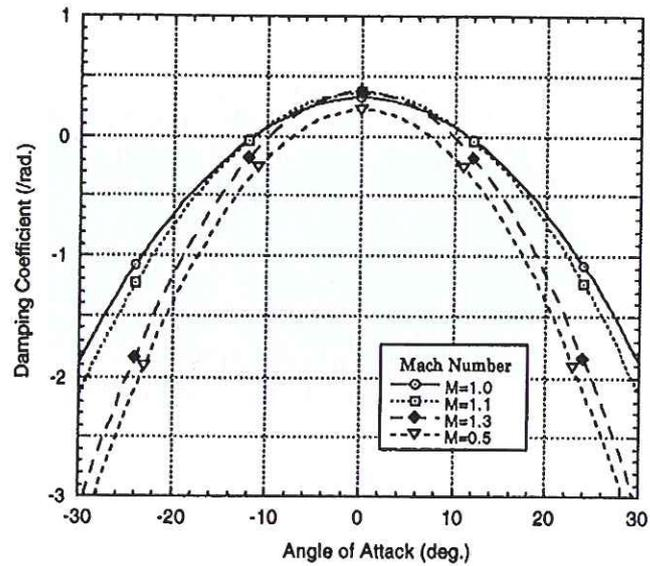
Fig. 16: Obtained damping-in-pitch coefficients by the curve-fit.
