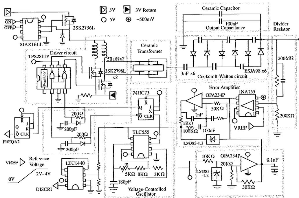
Fig1 Schematic circuit of high voltage power supply
