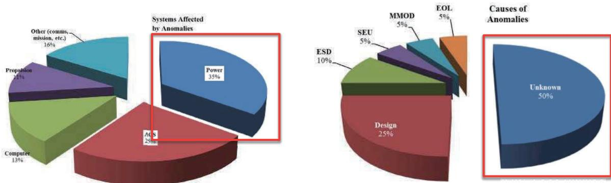
Fig. 1. The system most affected by anomalies is the power system which largely includes solar arrays and batteries.
