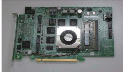
FPGA board specially designed for the algorithm. The board is manufactured by Soliton systems.
