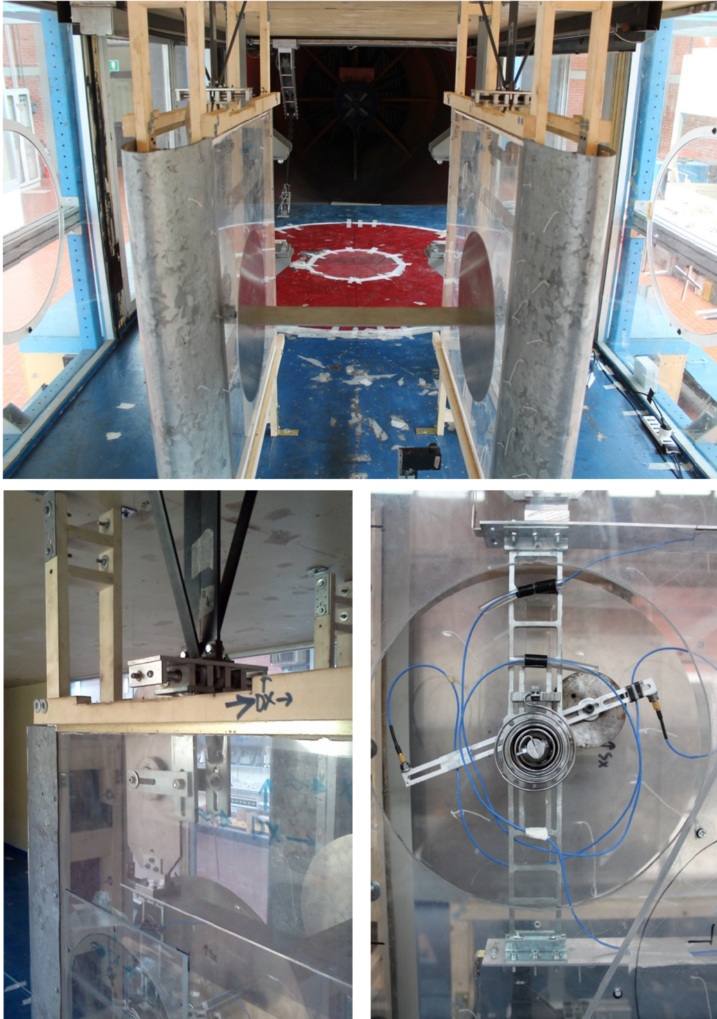
Figure 2: Frontal view of the aeroelastic setup (top); close-ups of the damping devices (bottom-left) and of the Vierendeel girder with clock spring and hooking system for the elastic/mass centre control (bottom-right).
