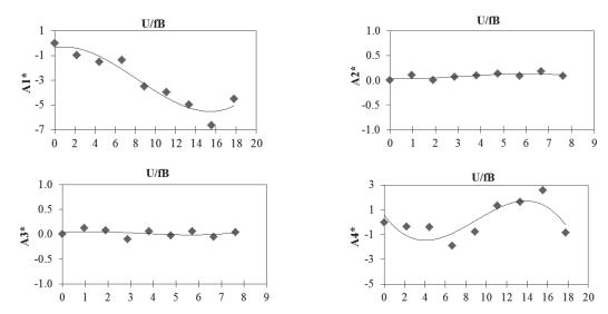
Figure 6: Torsional flutter derivatives and three order fitted polynomial, indicated by solid line
