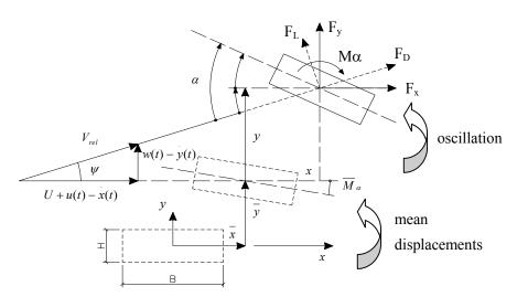
Figure 1: Instantaneous velocity and deck motion
