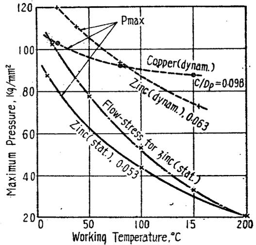
Fig. 9. Some Examples of Temperature Dependencies of Flow-Stress and Extruding Pressures.
