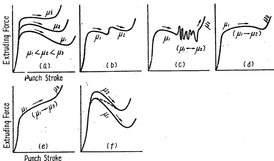
Fig. 18. Schematic Figures of Extruding Force-Stroke Diagram to Explain Effect of Coefficient of Friction.
