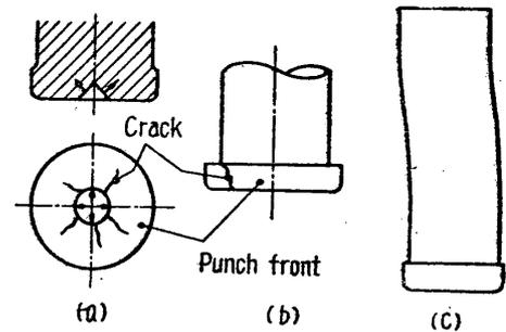
Fig. 27. Various Types of Punch Failure: (a) radial cracking around centre hole on punch front, (b) breakage of projected thin punch front, (c) buckling failure of punch body.
