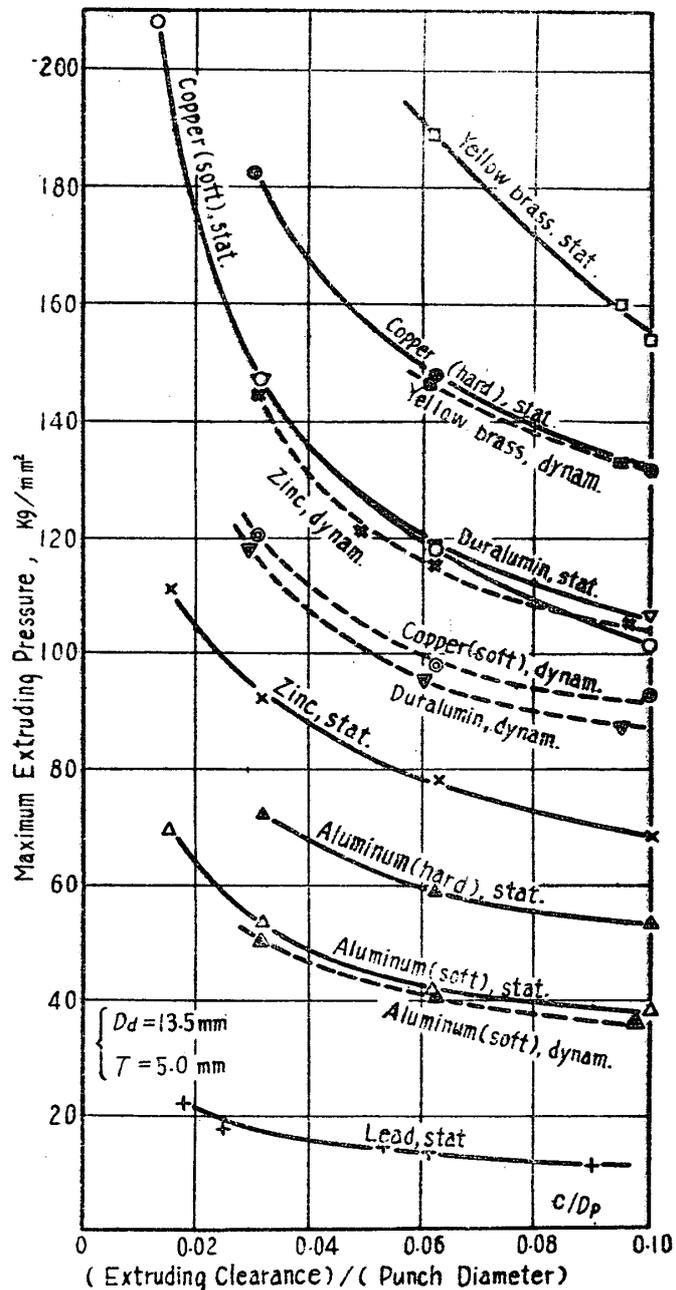
Fig. 6. Maximum Extruding Pressures for Various Metals and Tempers as Functions of Ratio of Extruding Clearance to Punch Diameter.
