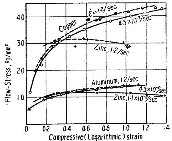
Fig. 12. Flow-Stresses at High and Low Strain-Rates.
