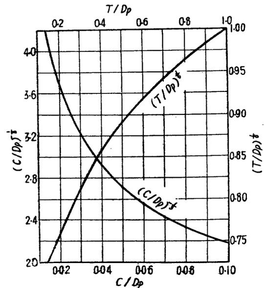
Fig. 29. Graphical Representation of  $(C/D_p)^{-1/3}$  and  $(T/D_p)^{1/6}$  Included in Empirical Formula for Maximum Statical Extruding Pressure.
