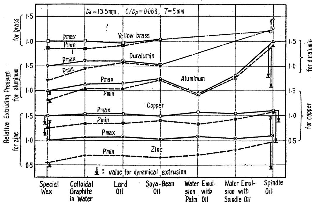
Fig. 19. Effects of Applied Lubricant on Statical Maximum and Minimum Extruding Pressures Using Tools Finished by Fine Carborundum Paper.
