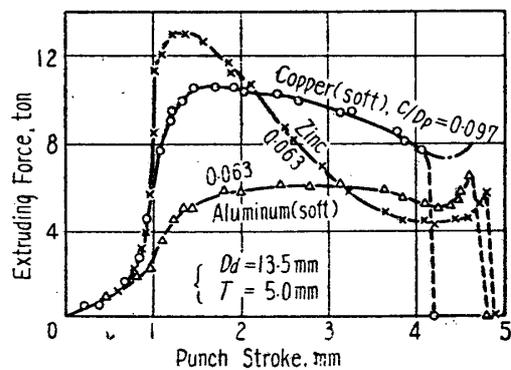
Fig. 11. Dynamical Extruding Force-Stroke Diagrams.
