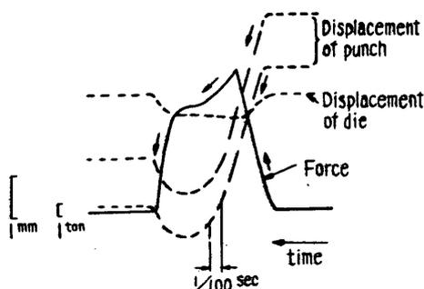
Fig. 4. An Example of Record of Punch Force and Displacement in Dynamical Extrusion of Copper. ( $D_p=11.3$  mm,  $T=5$  mm,  $C/D_p=0.097$ , Water Emulsion with Palm Oil)
