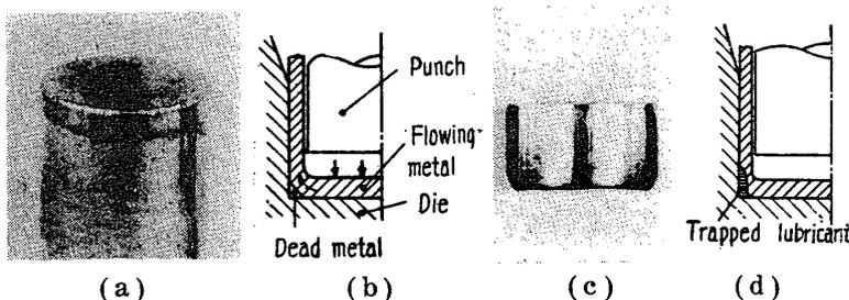
Fig. 24. Photographs and Discriptive Figures for Failures at Bottom Edge of Extruded Shell.
