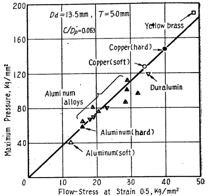
Fig. 8. Relation between Maximum Extruding Pressures and Flow-Stresses of Metals.
