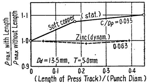
Fig. 15. Effect of Length of Press Track on Maximum Extruding Pressure.
