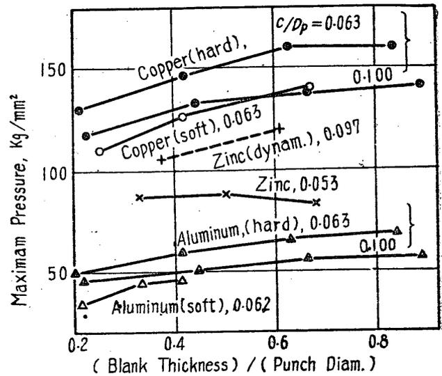
Fig. 17. Effect of Initial Blank Thickness on Maximum Static Extruding Pressure.
