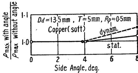
Fig. 14. Effect of Side Angle of Punch Face on Maximum Extruding Pressure.
