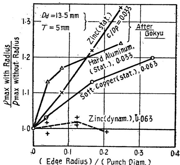
Fig. 13. Effect of Edge Radius of Punch Face on Extruding Pressure.
