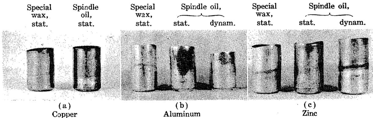
Fig. 25. Surface Appearances of Extruded Shells As Were Affected by Kind of Lubricant and by Extruding Speed.
