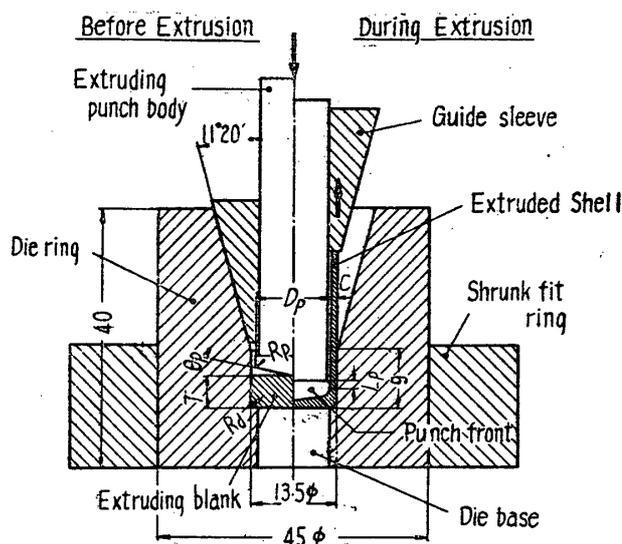
Fig. 1. Tool Assembly Used for Extruding Test with Die Cavity of Diameter 13.5 mm.
