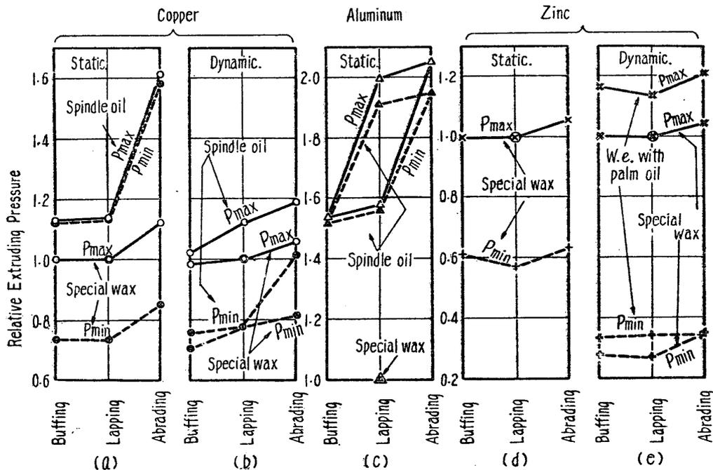
Fig. 20. Effects of Surface Roughness of Extruding Tool on Maximum and Minimum Extruding Pressures. (Extruding ratio  $C/D_p=0.063$ , die diameter 13.5 mm., blank thickness 5 mm.)
