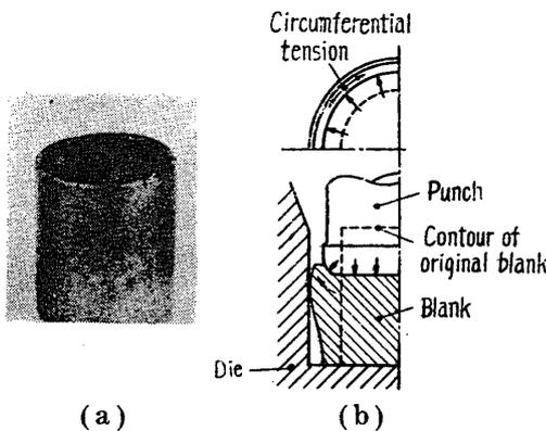
Fig. 22. Photograph and Descriptive Figure for Radial Cracking at Top Edge of Extruded Shell Wall.
