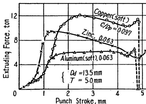
Fig. 5. Statical Extruding Force-Stroke Diagrams.
