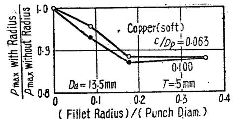
Fig. 16. Effect of Fillet Radius of Die Bottom on Maximum Static Extruding Pressure.
