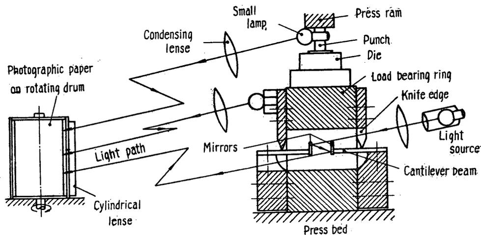
Fig. 3. Load and Displacement Recording Devices Used for Dynamical Extrusion.
