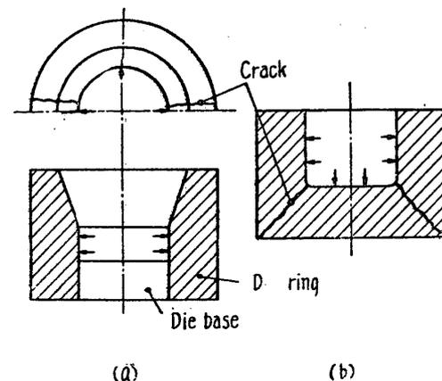
Fig. 28. Radial Cracking (a) and Cracking along Conical Surface (b) of Die.
