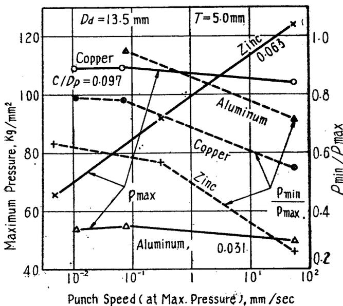
Fig. 10. Effect of Extruding Speed on Maximum Pressure and on Ratio of Minimum to Maximum Pressure.
