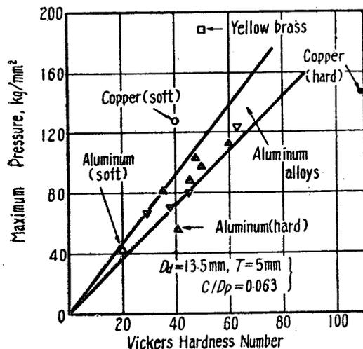
Fig. 30. Relation Between Maximum Extruding Pressures and Vickers Hardness Numbers of Metals.
