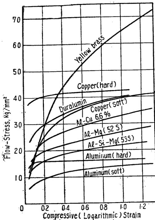
Fig. 7. Statical Flow-Stress Curves or Compressive Stress versus Strain Relations for Metals Tested.
