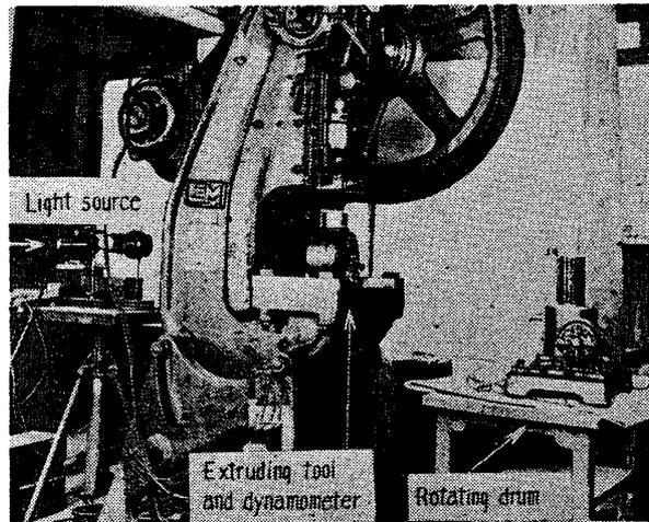
Fig. 2. Photograph Showing Crank Press, Extruding Tool and Ring Dynamometer Used for Experiment.
