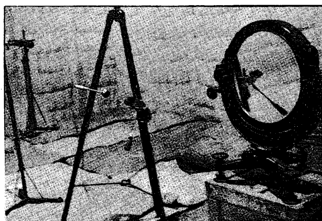
Fig. 5 (b) Arrangement of pistol, microphone and concave mirror.
