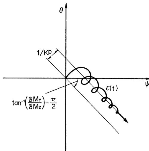
FIGURE 2.5. Locus of the complex angle for the step input of control movements (for  $\mu > 0$ ).
