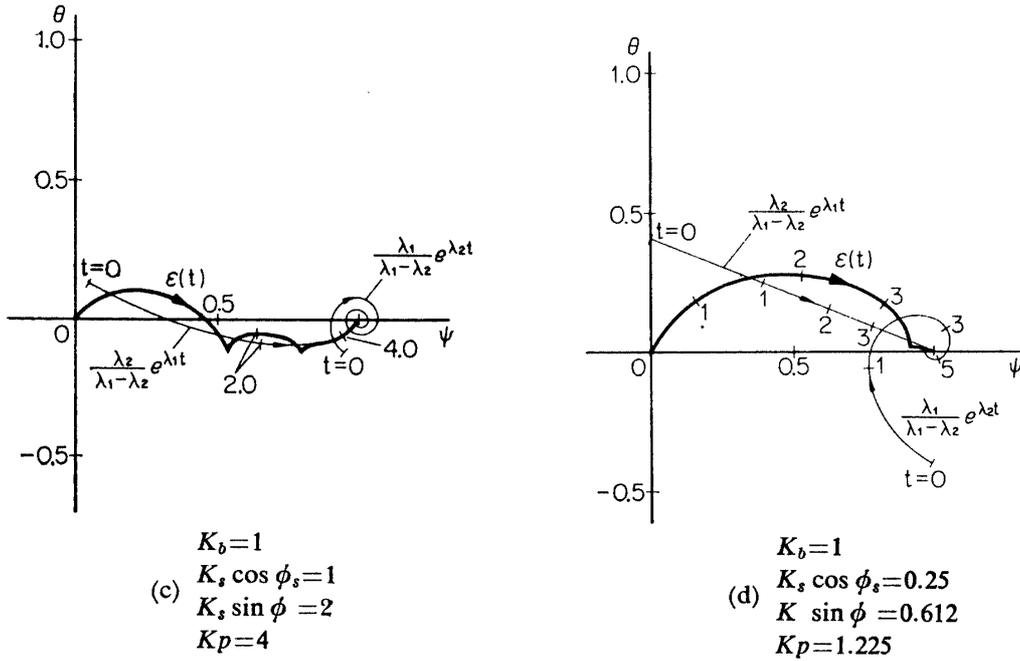
FIGURE 4.10. Time response for step input,  $\epsilon_i=1$  for optimum condition (4.11) or (4.19).
