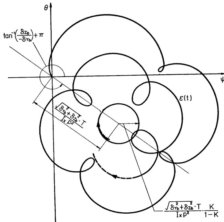
FIGURE 2.4. Locus of the complex angle for step input of thrust malalignment (for  $\mu > 0$ ).
