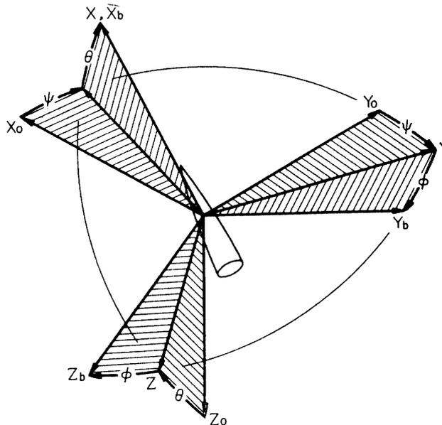
FIGURE 2.1. Orientation of body and stability axes with respect to space fixed axes.
