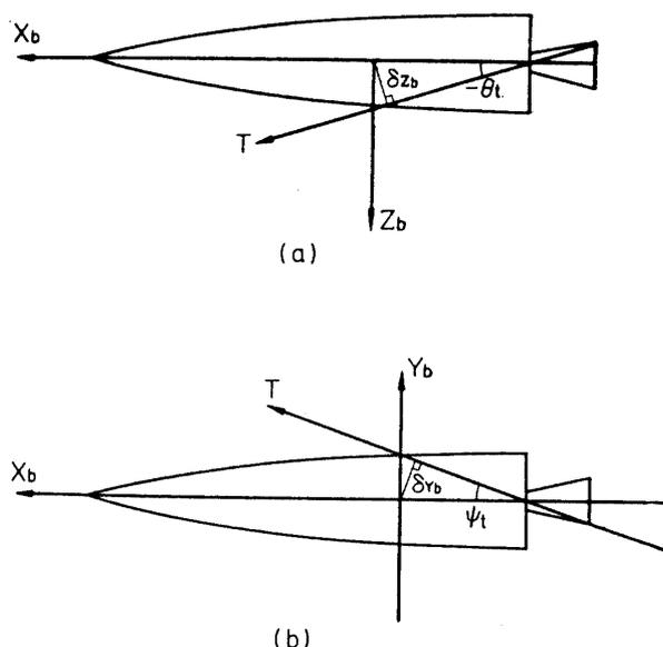
FIGURE 2.2. Thrust malalignment.
