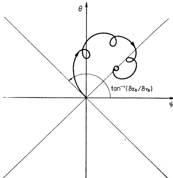
FIGURE 3.2. Locus of the complex angle for the thrust malalignment about the feedback system.
