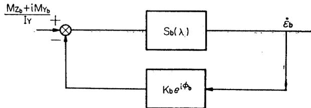
FIGURE 3.1. Angular rate feedback system.
