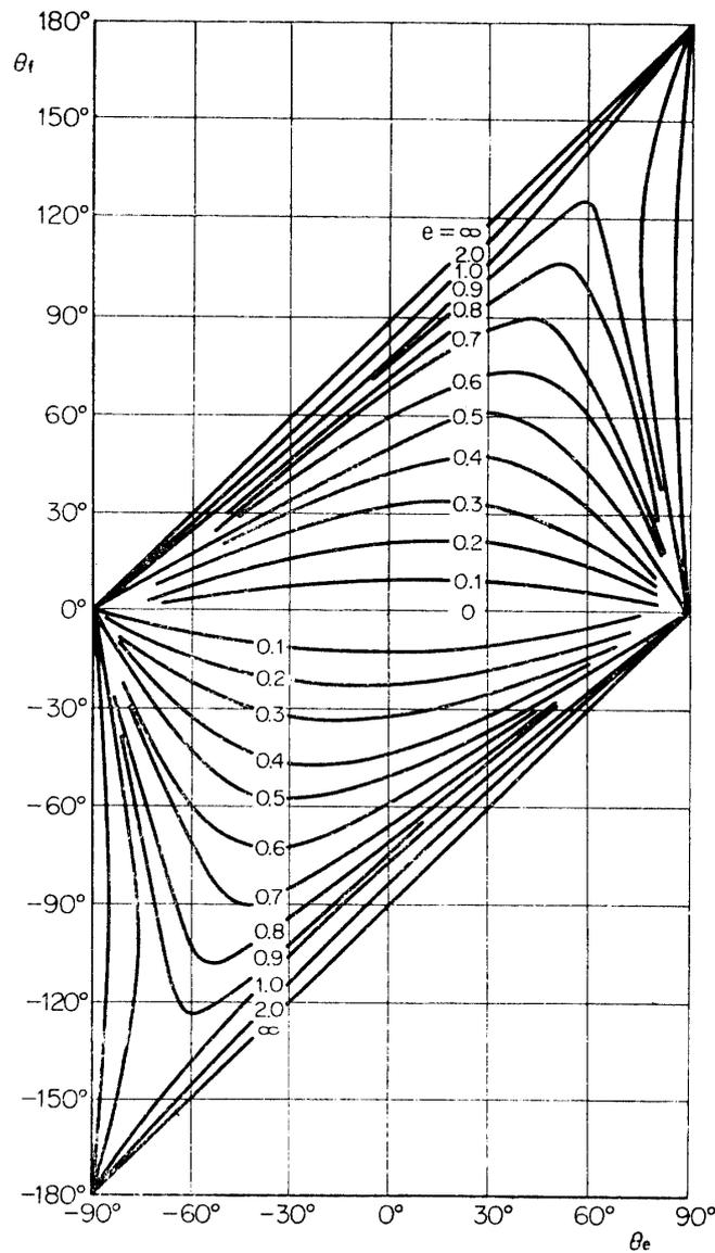
FIGURE 2.7. Stability region for the second order system with complex coefficients.
