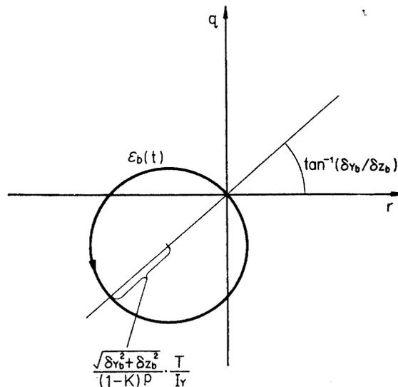
FIGURE 2.3. Locus of the complex angular velocity for step input of thrust malalignment.
