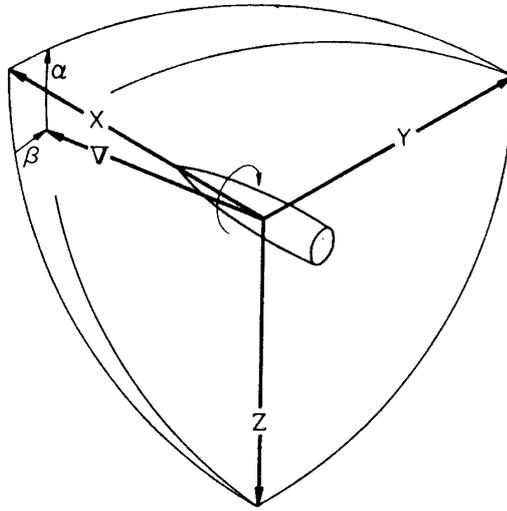
FIGURE 5.1. Orientation of velocity vector with respect to stability axes.
