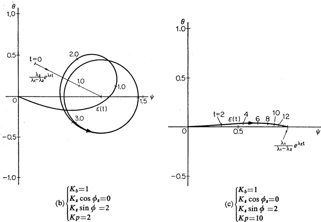
FIGURE 4.8. Time response for step input,  $\epsilon_i=1$ , for  $K_b=1$ ,  $K_s \cos \phi_s=0$   $K_s \sin \phi = 2$
