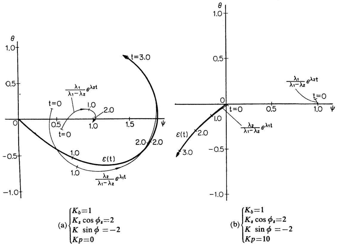
FIGURE 4.4. Time response for step input,  $\epsilon_i=1$ , for  $K_b=1$ ,  $K_s \cos \phi_s=2$ ,  $K \sin \phi = -2$
