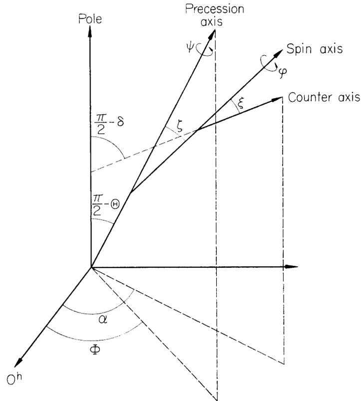
FIG. 20. Illustrative geometrical configuration to calculate the aspect of a counter on a rocket.
