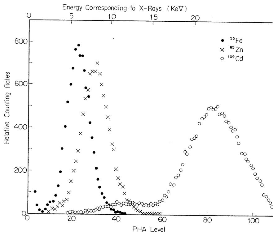
FIG. 4. Pulse height spectra of X-rays from  $^{55}\text{Fe}$ ,  $^{65}\text{Zn}$  and  $^{109}\text{Cd}$  detected with a scintillation counter.
