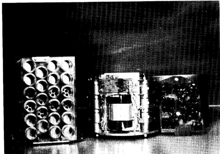
FIG. 14. The X-ray instrument with GM counter borne on the rocket, K-9M-15. On the left in this photo twenty-three GM counters are shown.
