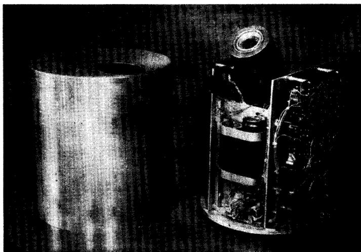
FIG. 1. The Scintillation counter borne on the rocket, L-3-3.
