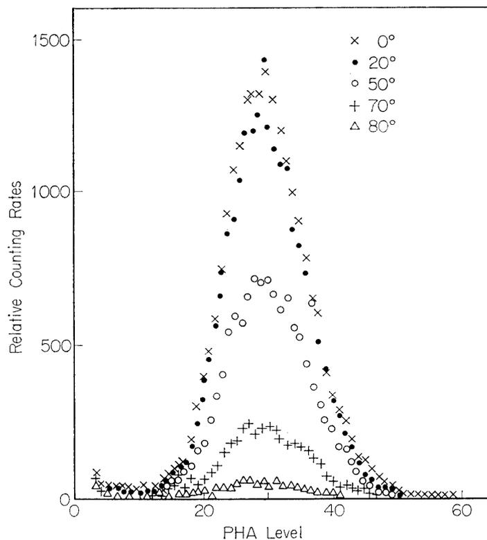
FIG. 5. Pulse height distributions of X-rays of 8.03 keV from directions of  $0^\circ$ ,  $20^\circ$ ,  $50^\circ$ ,  $70^\circ$  and  $80^\circ$  detected with a scintillation counter.
