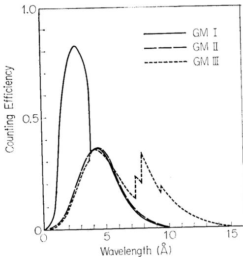
FIG. 15. Counting efficiencies of GM counters for normal incidence of X-rays.
