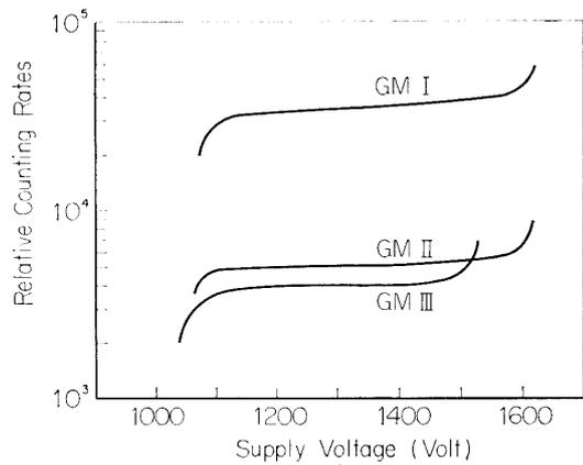
FIG. 16. Plateau curves of GM counters. Experimental results due to X-rays radiated from <sup>55</sup>Fe.
