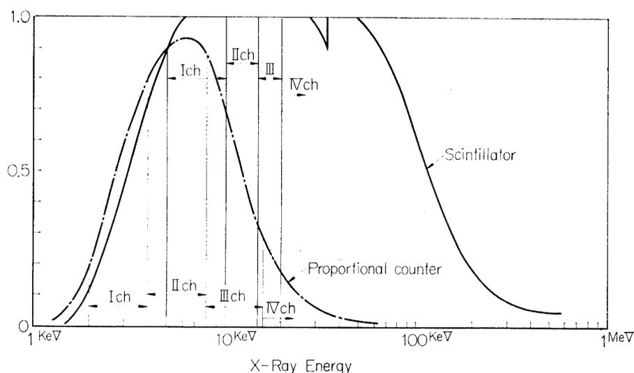
FIG. 2. Calculated counting efficiencies of a scintillator and a proportional counter for normal incidence of X-rays.
