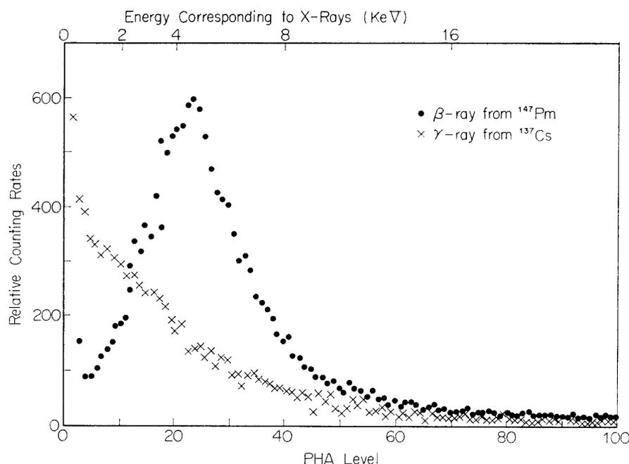
FIG. 12. Spectral distributions of  $\gamma$ - and  $\beta$ -rays detected with a proportional counter.
