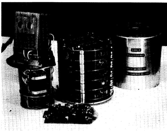
FIG. 9. The X-ray instrument with proportional counters borne on the rocket, K-9M-12. On the left in this photo four proportional counters packed and high tension supplies, in the center the electronic system and on the right the case of electronic system are shown.
