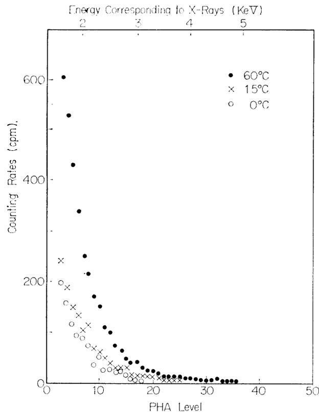
FIG. 3. Temperature dependence of thermal noise of a photomultiplier.
