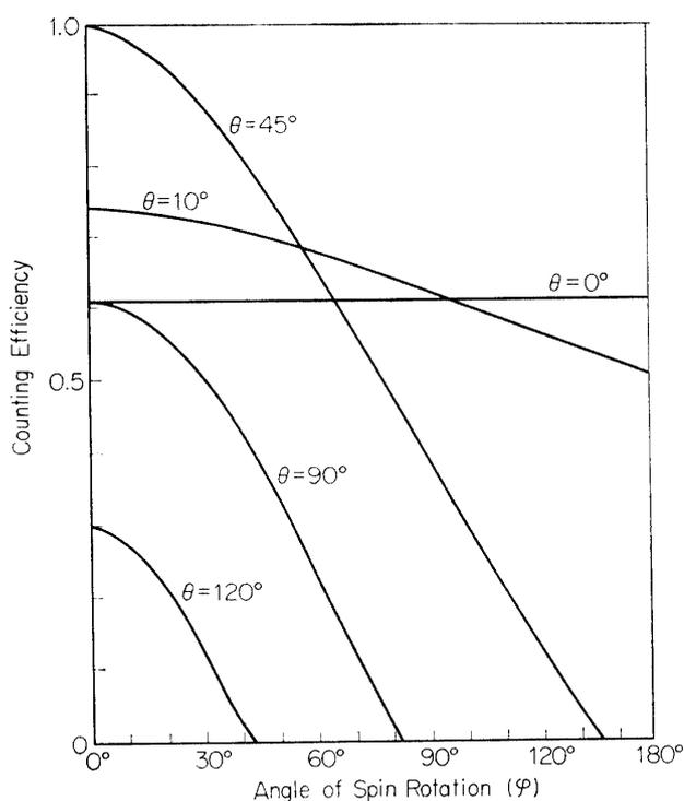
FIG. 6. Angular response of a scintillation counter.
