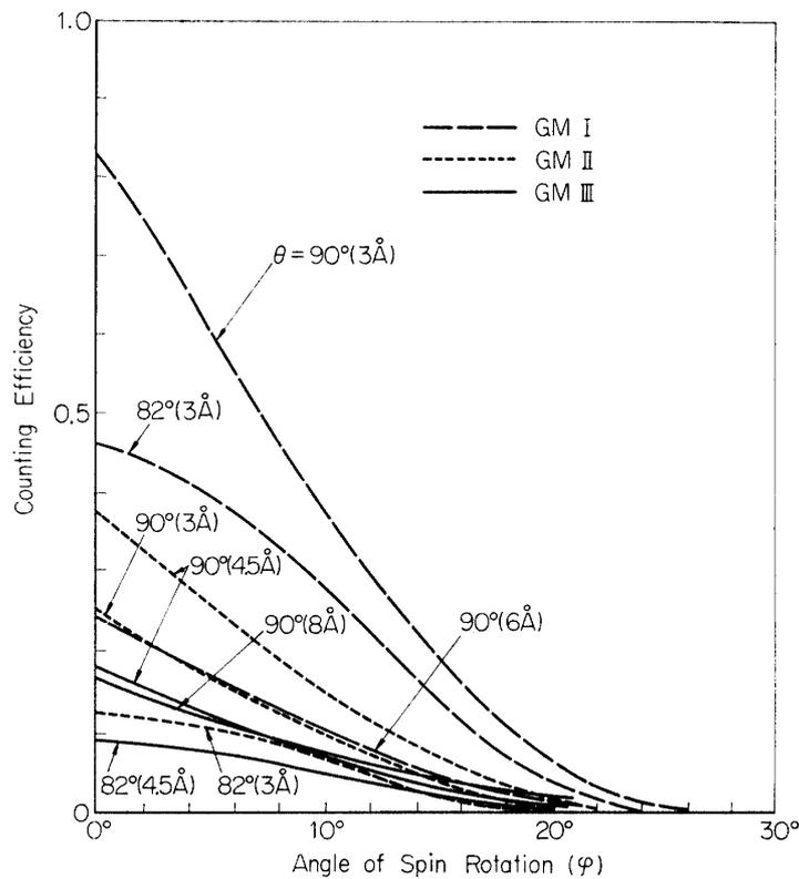
FIG. 17. Examples of angular responses of X-rays calculated for GM counters.
