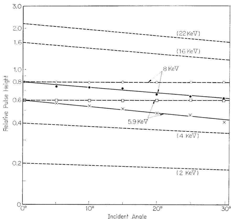
FIG. 10. Angular response of pulse heights. Solid lines and dotted lines denote those for X-rays of incident angles perpendicular to the anode line of a counter and dashed lines those for X-rays of incident angles on the plane perpendicular to the anode lines. Marks, ●, ○, × and □ denote experimental values.
