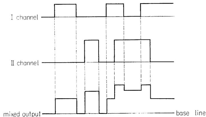
FIG. 19. Output mode of X-ray records.
