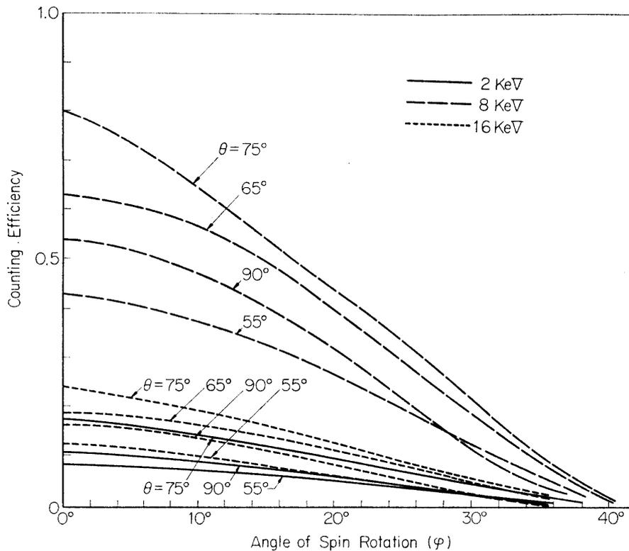
FIG. 11. Angular responses calculated for X-rays of 2, 8 and 16 KeV for a proportional counter in the case of  $\xi=75^\circ$ .
