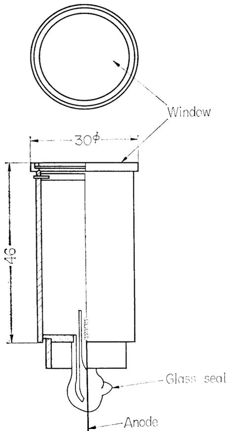
FIG. 13. Two side views of a GM counter (mm unit).
