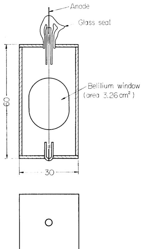
FIG. 8. Two side views of a proportional counter (mm unit).
