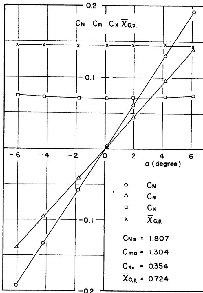
FIG. 11. Variation of  $C_n$ ,  $C_m$ ,  $C_x$  and  $x_{c.p.}$  with angle of attack.  $M=3$ .
