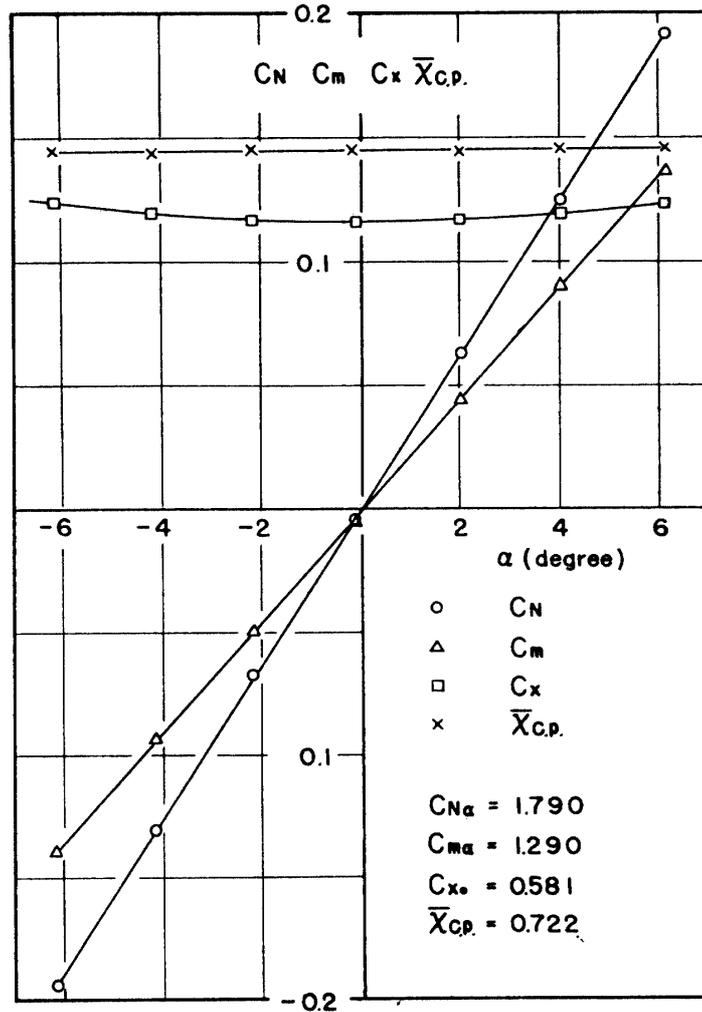
FIG. 10. Variation of  $C_n$ ,  $C_m$ ,  $C_x$  and  $x_{c.p}$  with angle of attack.  $M=2$ .
