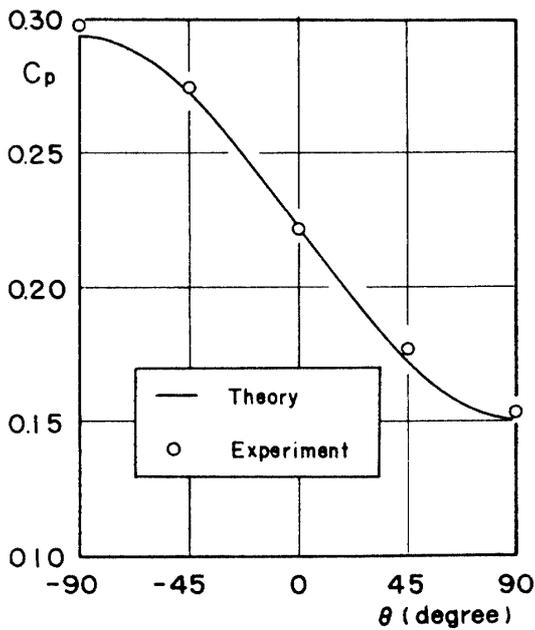
FIG. 8. Surface pressure distribution on cone.  $M=2$ ,  $\alpha=4^\circ$ .
