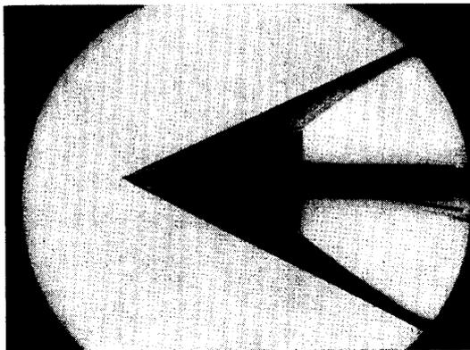
FIG. 12c. Schlieren photograph of a flow field around a cone.  $M=3$ ,  $\delta=16^\circ$ ,  $\alpha=0^\circ$ .
