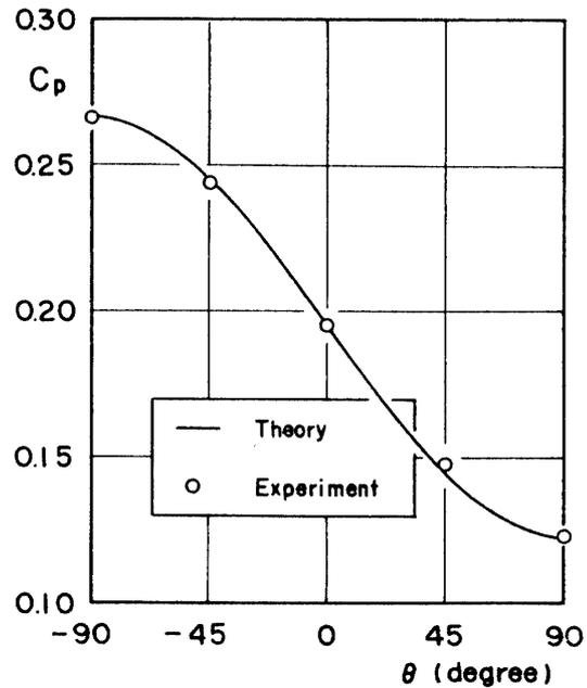
FIG. 9. Surface pressure distribution on cone.  $M=3$ ,  $\alpha=4^\circ$ .
