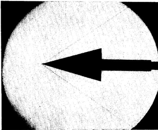
FIG. 12a. Schlieren photograph of a flow field around a cone.  $M=2$ ,  $\delta=16^\circ$ ,  $\alpha=0^\circ$ .
