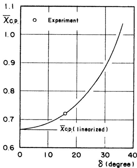
FIG. 5. Location of center of pressure for cone.
