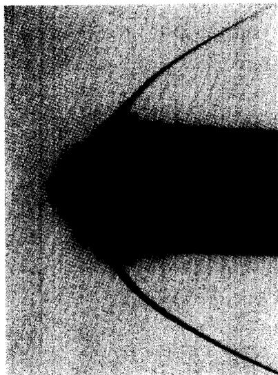
FIG. 13a. Schlieren photograph of a flow field around a cone.  $M=4$ ,  $\delta=40.57^\circ$ ,  $\alpha=0^\circ$ .
