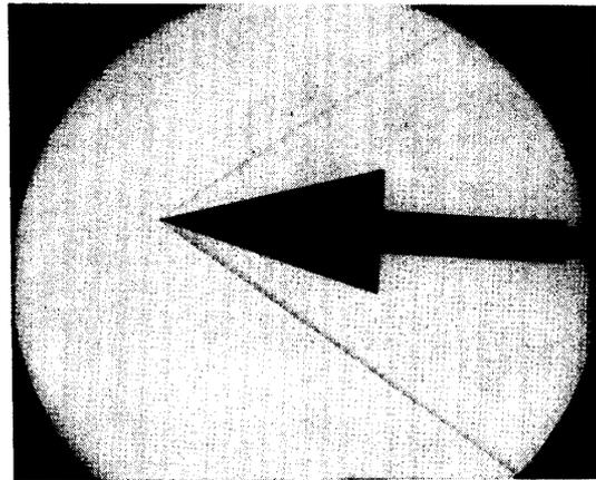
FIG. 12b. Schlieren photograph of a flow field around a cone.  $M=2$ ,  $\delta=16^\circ$ ,  $\alpha=4^\circ$ .
