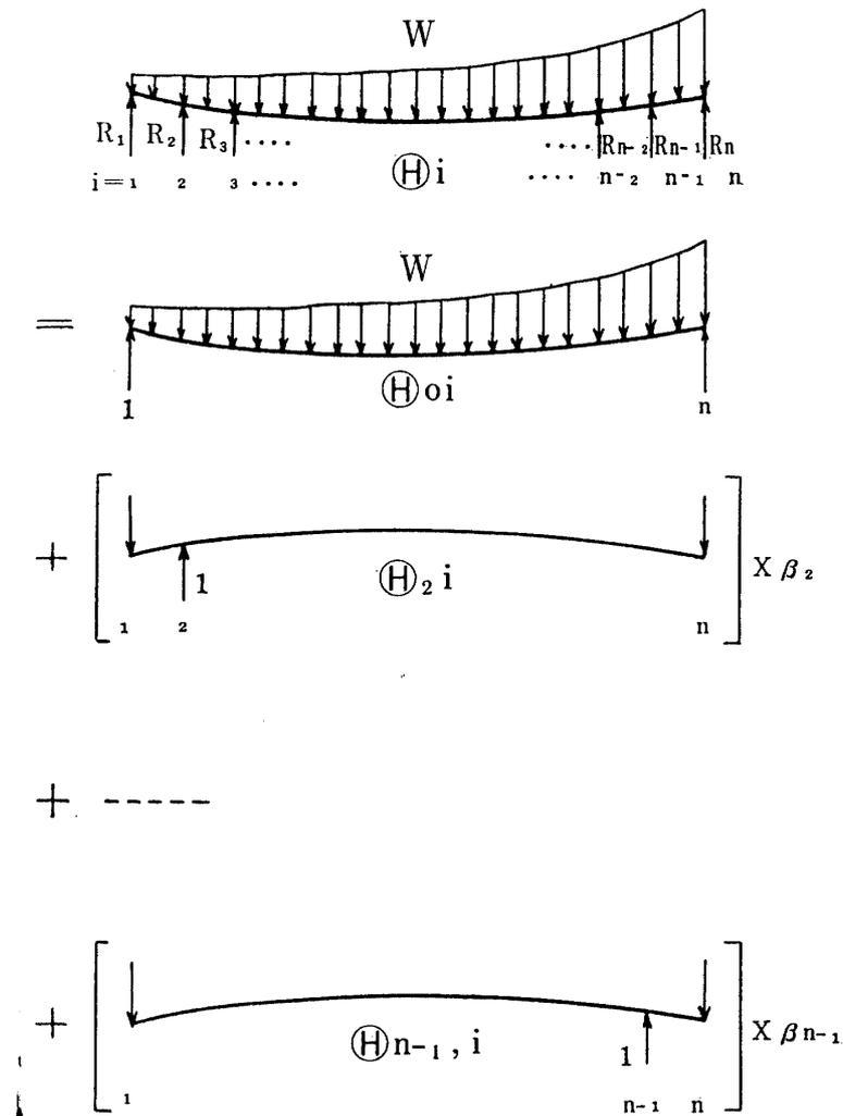
FIG. 1. Determination of the slope of the deflection
