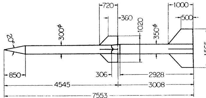
FIG. 2. Dimensional details of LS-A rocket
