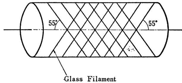
FIG. 1. 55 degree winding pattern sketch
