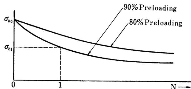
FIG. 2. Typical low cycle fatigue effects illustrated
