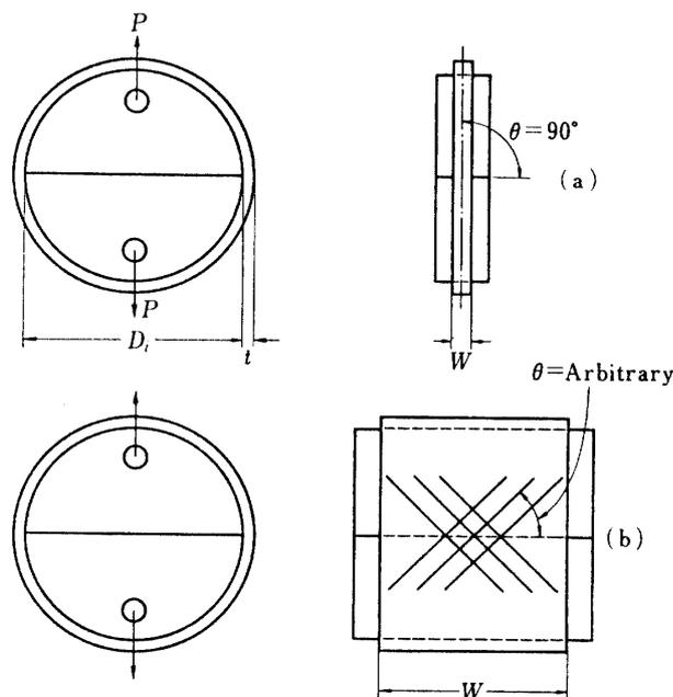
FIG. 4. (a) NOL ring test and (b) ISAS ring test
