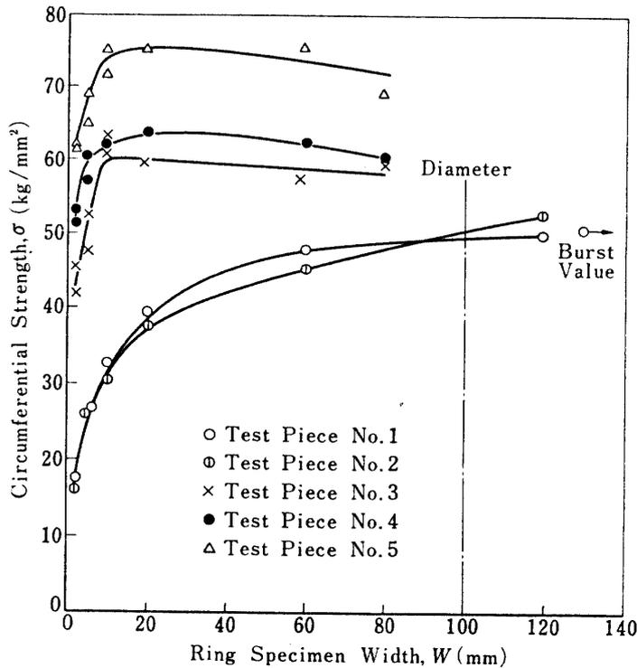
FIG. 9. Ring specimen width effects on circumferential strength: ISAS ring test and burst test
