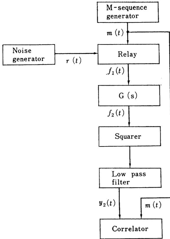
FIG. 2. Measuring system by  $M$ -sequence correlation method.
