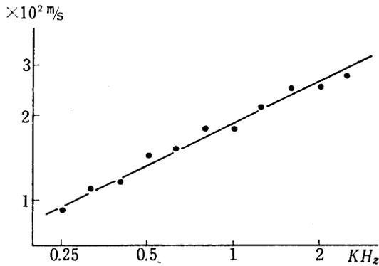
FIG. 10. Wave velocity vs. frequency. Measured by *M*-sequence signal correlation method.
