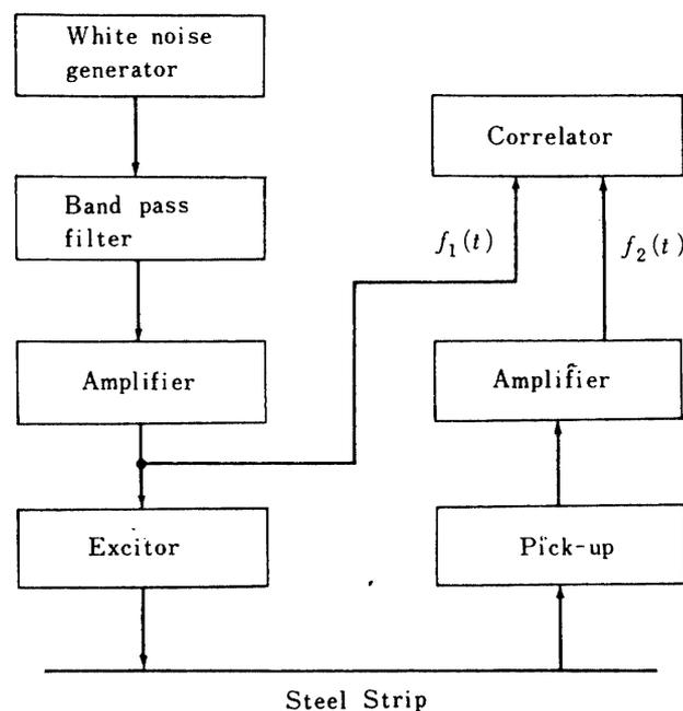
FIG. 3. Flexural wave propagation measurement by ordinary correlation method.
