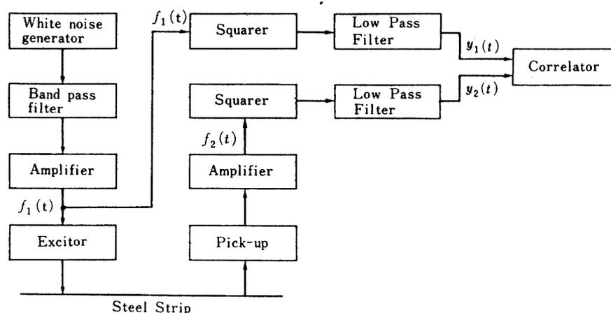
FIG. 6. Flexural wave propagation measurement by squared signal correlation method.
