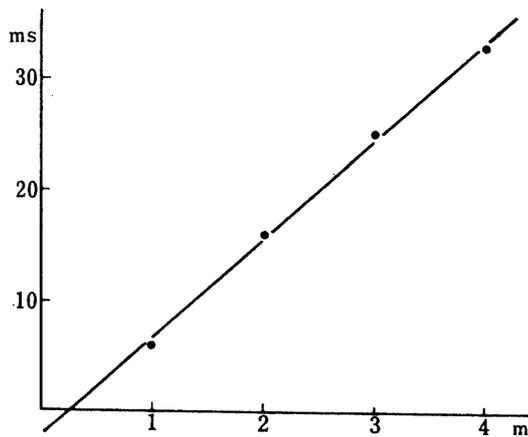
FIG. 8. Delay time vs. distance. Measured by squared signal correlation method.
