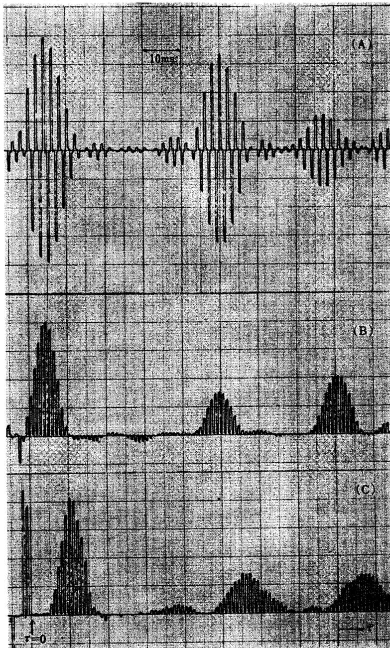
FIG. 11. Measurement of multiple wave paths by (A) ordinary correlation method, (B) squared signal correlation method and (C) *M*-sequence signal correlation method.
