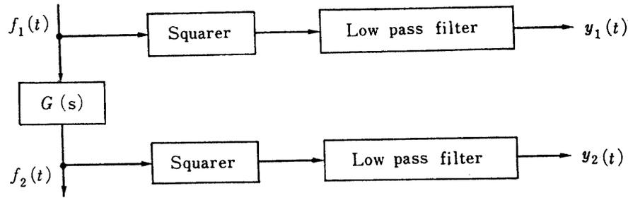
FIG. 1. Measuring system by squared signal correlation method.
