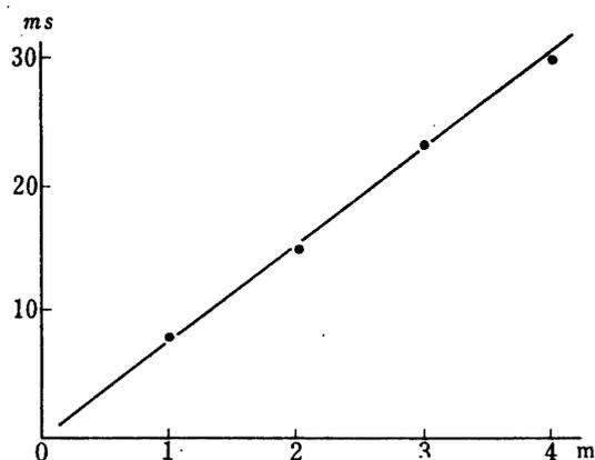
FIG. 5. Delay time vs. distance. Measured by ordinary correlation method.
