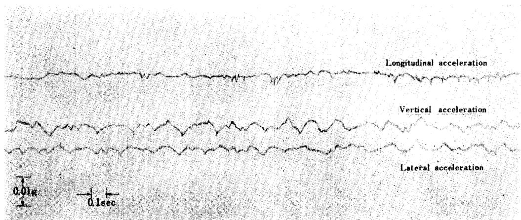
FIG. 21. An example of the variation of accelerations during 10 m/sec running test.
