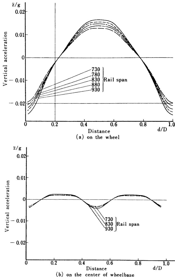
FIG. 5. Vertical acceleration caused by moving load.
