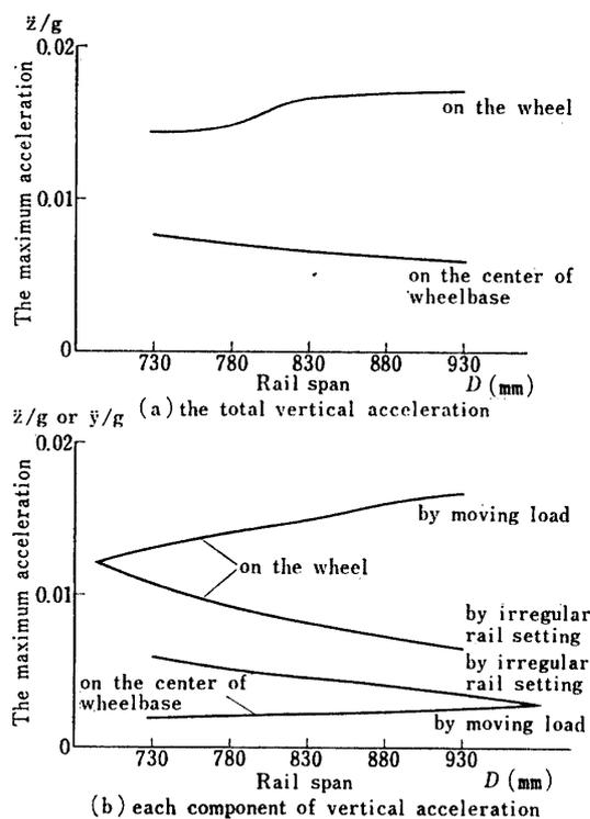
FIG. 8. The maximum acceleration.
