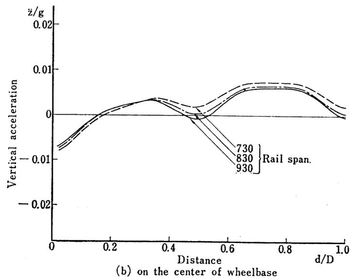
FIG. 7. The total vertical acceleration.
