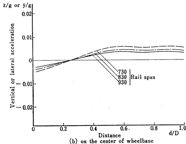
FIG. 6. Vertical or lateral acceleration caused by irregular rail setting.
