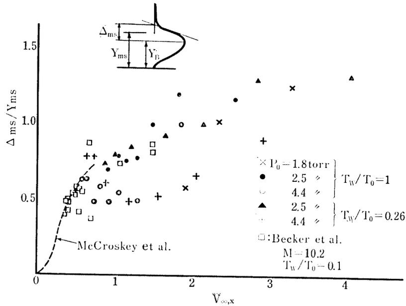
FIG. 19. Ratio of the thickness to the height of the shock layer
