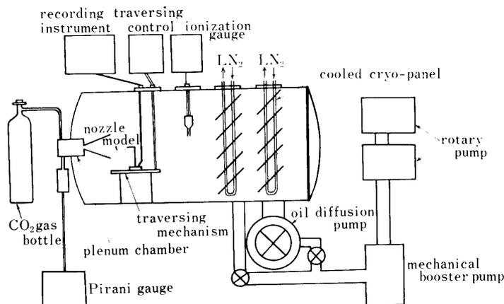
FIG. 2(a). Schematic view of the general setup
