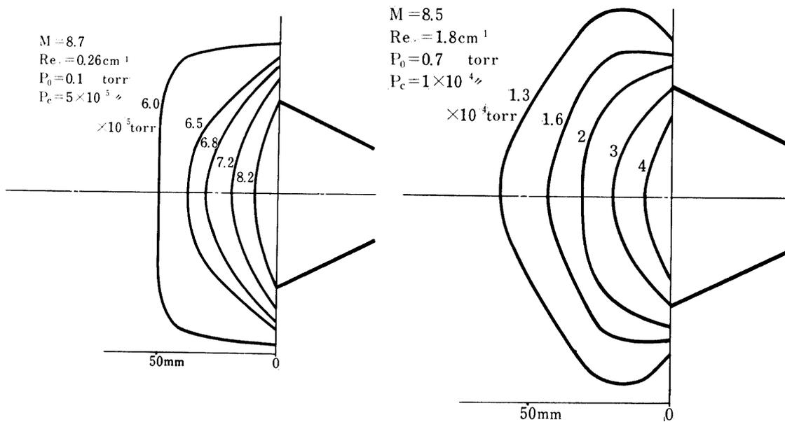
FIG. 14. Pressure distribution in the flow field (by the static pressure probe)
