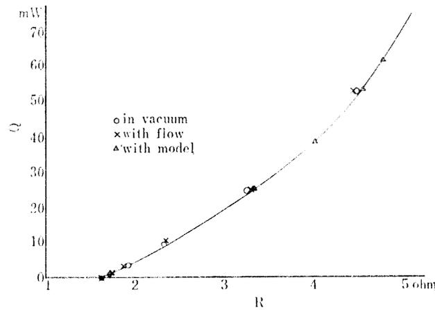
FIG. 7. Hot wire calibration curve
