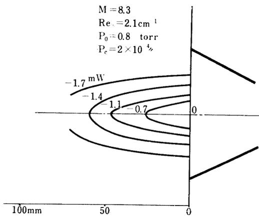
FIG. 15. Heat transfer rate due to the flow (by hot wire anemometer)
