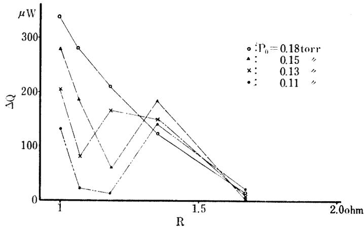
FIG. 9. The heat transfer rate due to the flow with the relation to wire resistance
