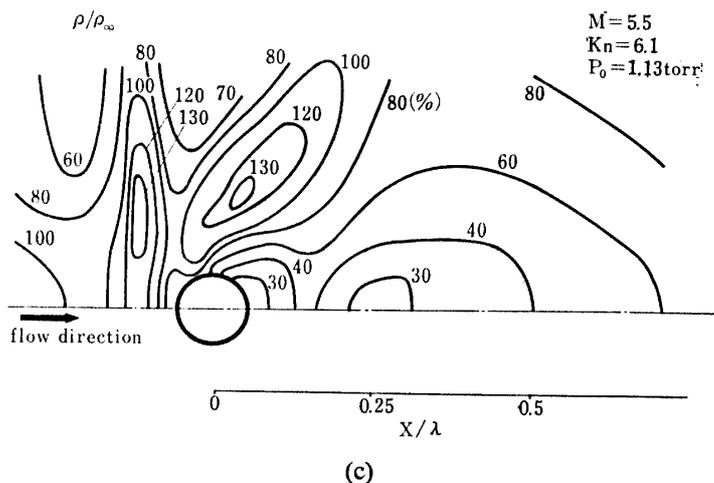
FIG. 24. Flow pattern around the cylinder (reduced from the Langmuir probe survey)
