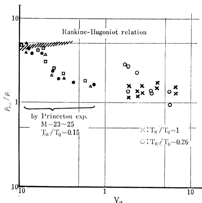
FIG. 22. Maximum density in the shock layer (reduced from the Langmuir probe survey)
