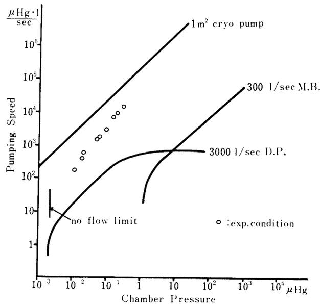
FIG. 1. Pumping performance of the wind tunnel.
