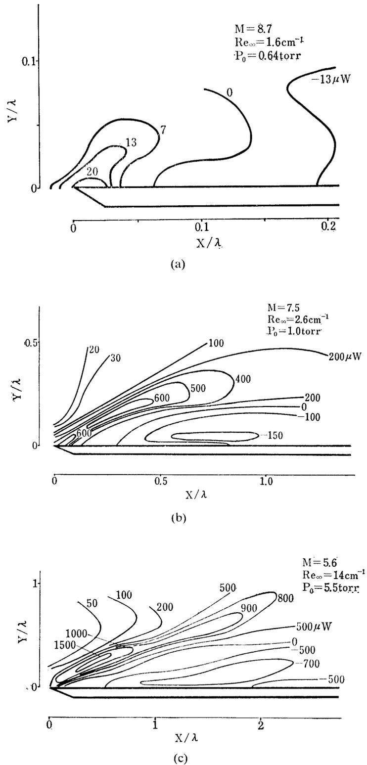
FIG. 23. Flow pattern past the sharp leading edge flat plate (reduced from the hot wire survey)
