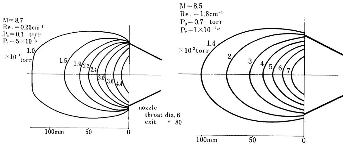
FIG. 13. Pressure distribution in the flow field (by the impact pressure probe)
