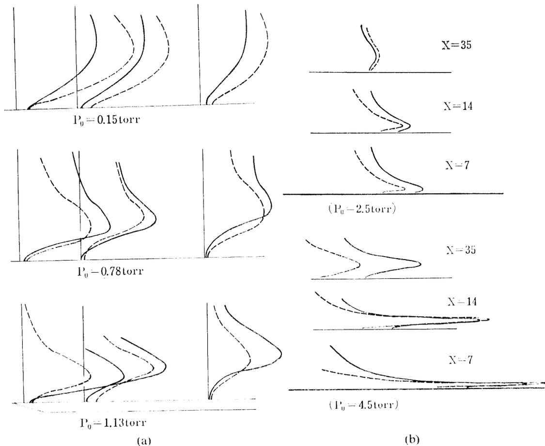
FIG. 21. Profiles by the probe surveys (The solid curve shows the adiabatic wall condition  $T_w/T_0=1$  and the dotted one the cold wall condition  $T_w/T_0=0.26$ .)
