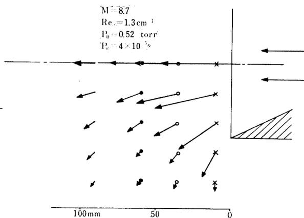
FIG. 16. The distribution of the free stream velocity vectors (by the hot wire anemometer)
