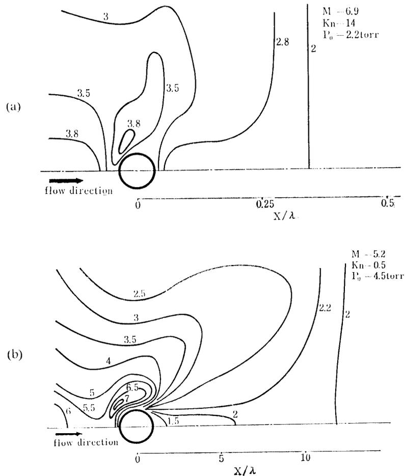
FIG. 25. Flow pattern around the cylinder (reduced from the hot wire survey)
