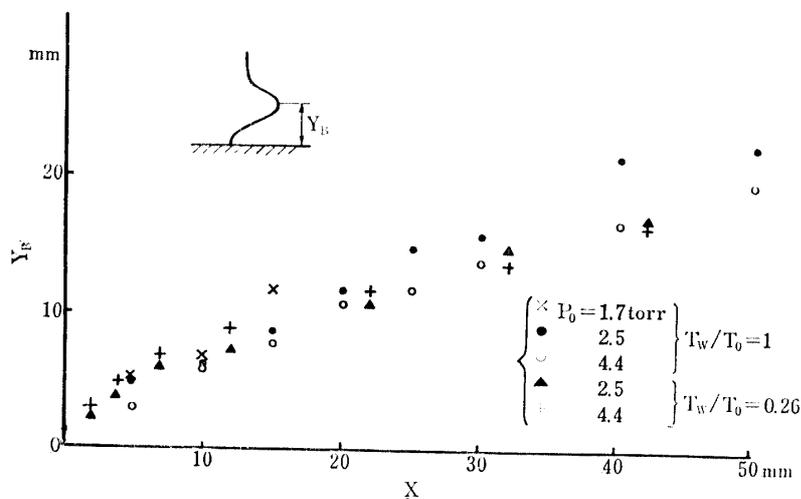
FIG. 20. Characteristic height of the shock layer with the relation to the distance from the leading edge
