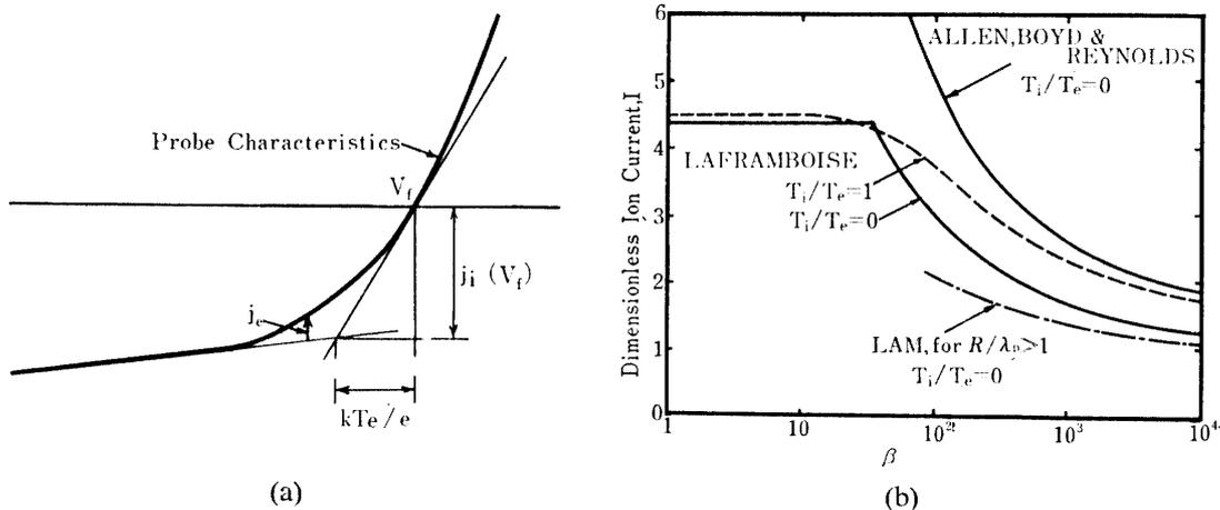
FIG. 12. Langmuir probe performance (from reference [53])
