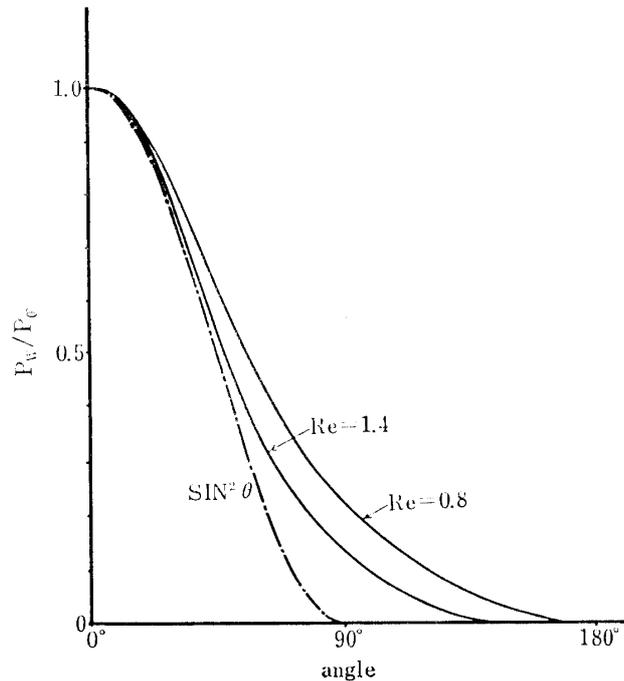
FIG. 27. Normalized surface pressure distribution around the cylinder
