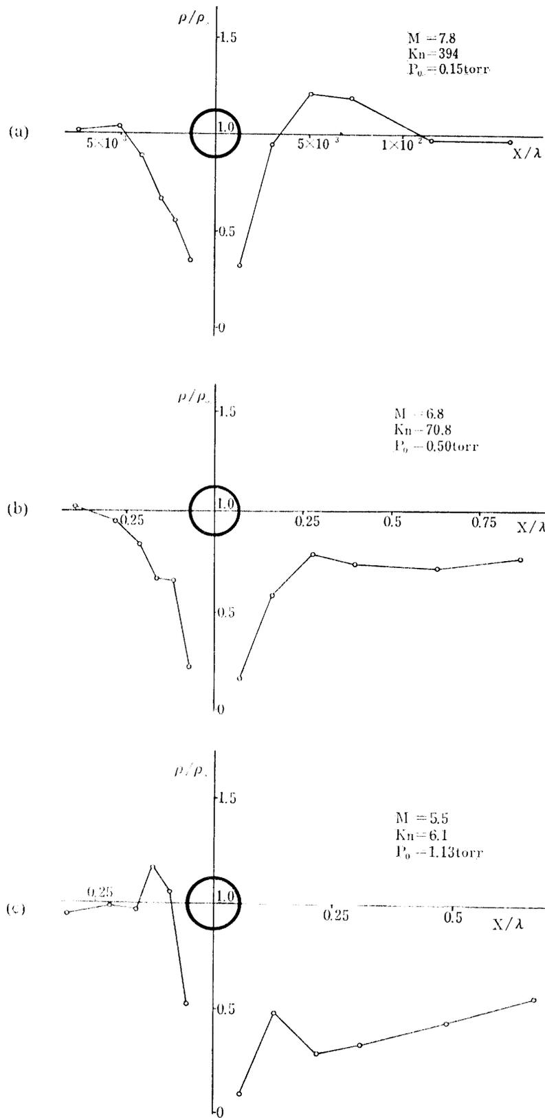
Fig. 26. Density distribution around the cylinder along the flow axis
