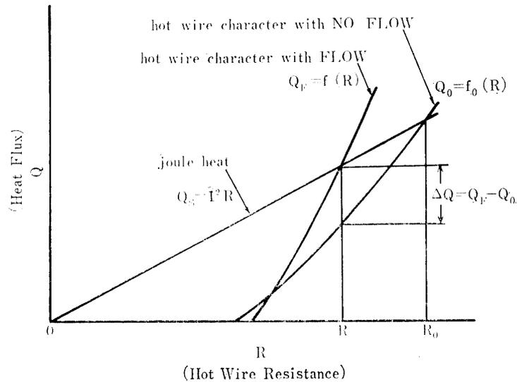
FIG. 8. Explanatory curves for the calculation of the heat transfer rate
